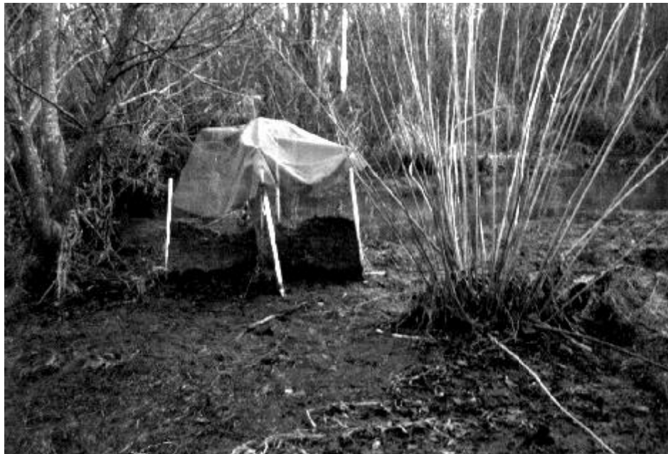
Figure IV-1. Multi-directional lateral litter collector (Mudll) before (A) and after (B) a significant flood event in riparian forests of South Carolina.
