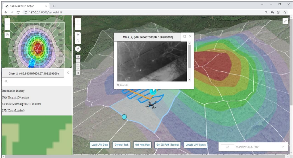
Figure 15. Pictures from the UAVs are displayed for further human identification during the human-UAV collaborative search task.
