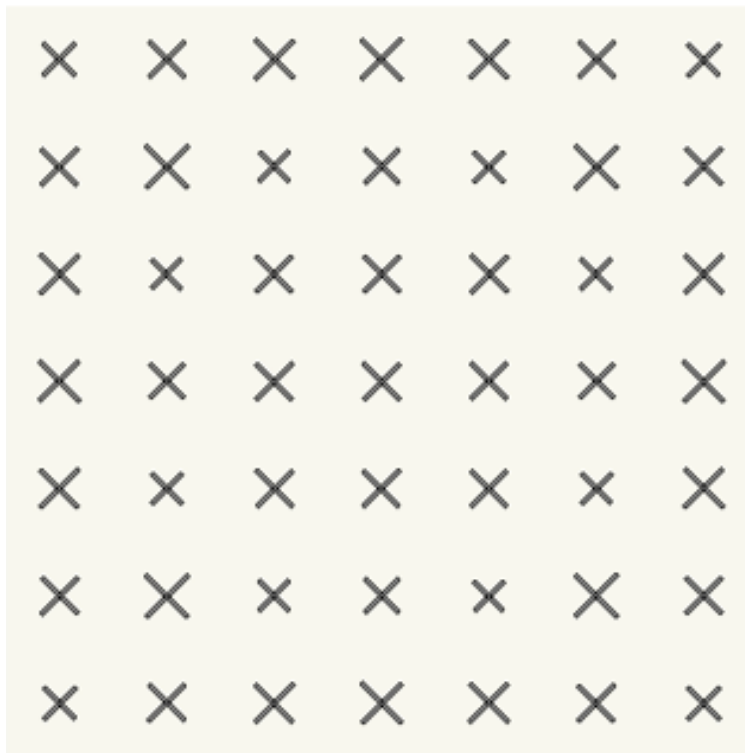
Figure 4.4: Simulation of the cross dipole reflectarray model
