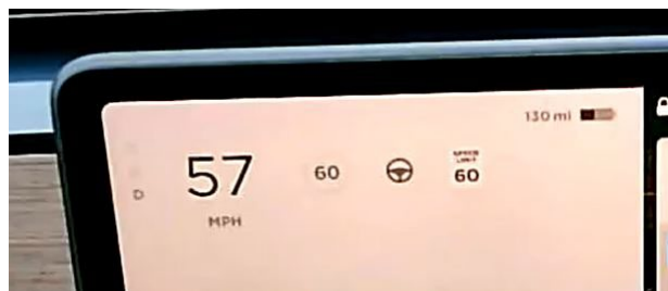
Figure 7. Photo. L2 Inactive (on standby) – Steering wheel and ACC speed set but steering wheel is black.
