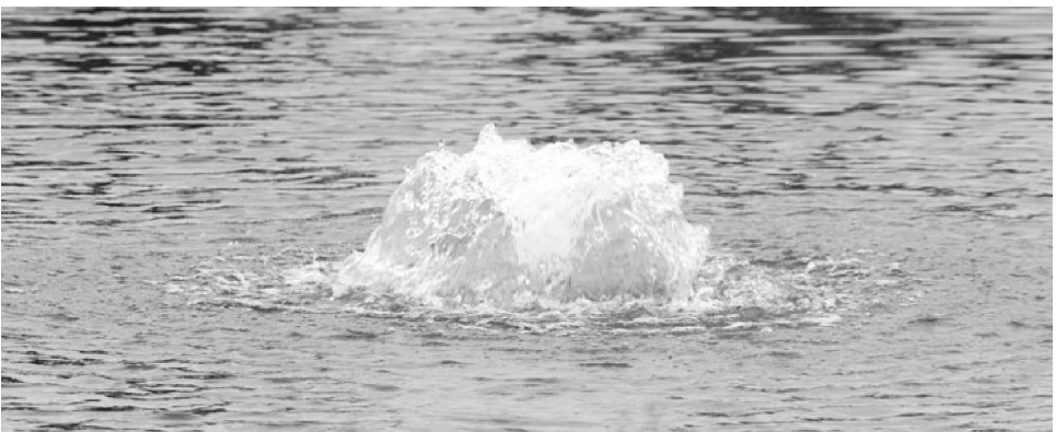
Figure 3. Water breakup pattern for Sweetwater Model HS5 unit (high air exposure, HAE).
