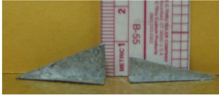
Figure 2.6 Side profile of the large (left) and small (right) surface mounted vortex generators
