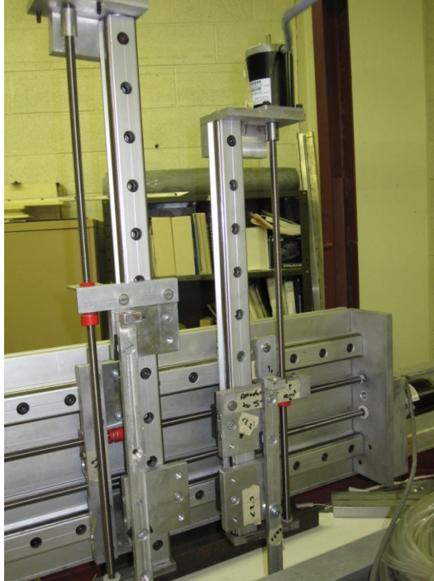
Figure 2.14 Downstream 2-D traverse for pitchwise and spanwise probe motion
