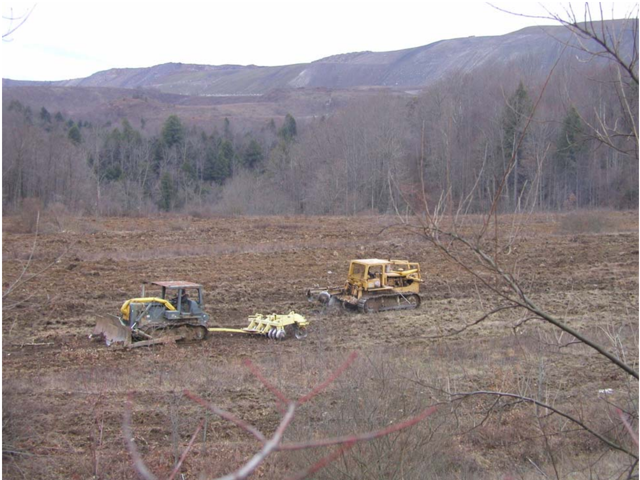
Figure 2. Preparing the experimental site in December, 2007. The large disk (left) is used first to break up the sod, then an advanced ripping device (right) was used to prepare the land for planting. See Evans et al. (2009) for further details.
