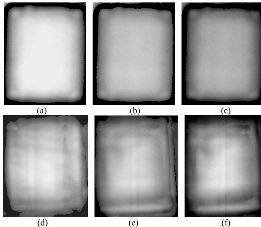
Figure 3.47. The SAM images of the sintered silver joints on nickel/silver-coated AlN DBC after 0 (a), 1000 (b), 2000 (c), 4000 (d), 6000 (e), and 8000 (f) thermal cycles, respectively.
