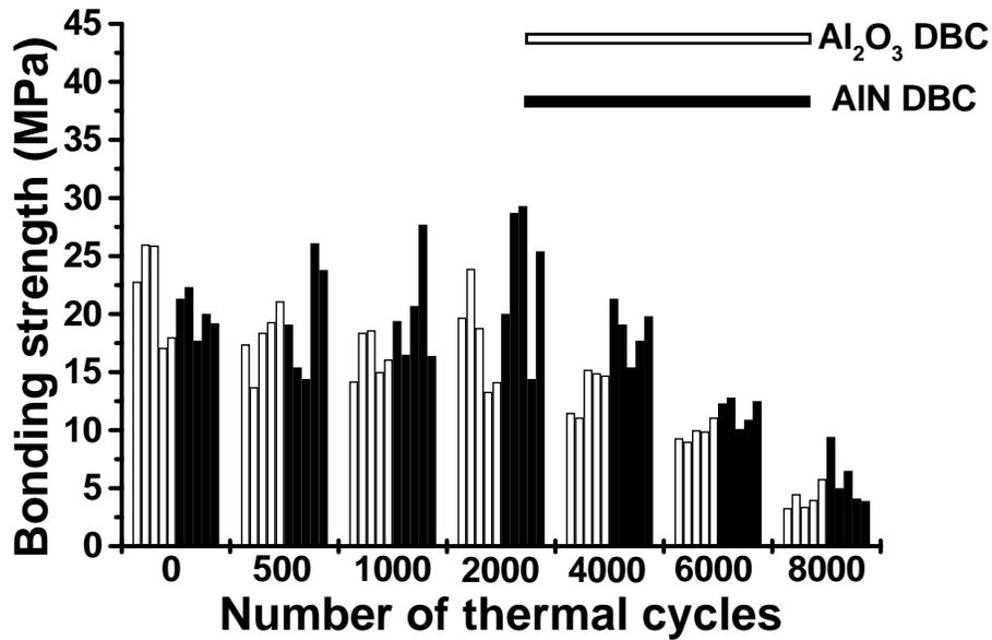
Figure 3.52. Changes of shear strength of the low-temperature sintered silver joints on nickel/gold-coated DBC substrates during the temperature cycling experiment.
