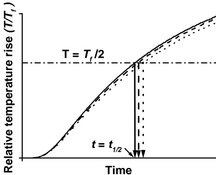
Fig. 2. The changes of the temperature transient curve at the rear surface of a specimen when changing the values of the solder/copper interfacial thermal resistance.
