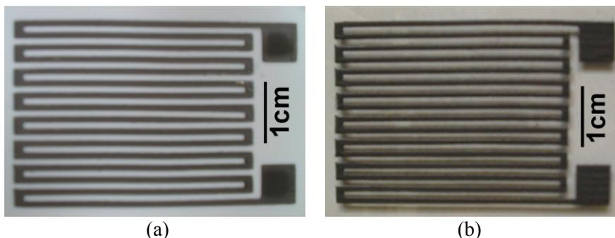
Figure 3.4. The stencil-printed nanoscale silver pattern on alumina (a) and that on glass (b) before sintering.
