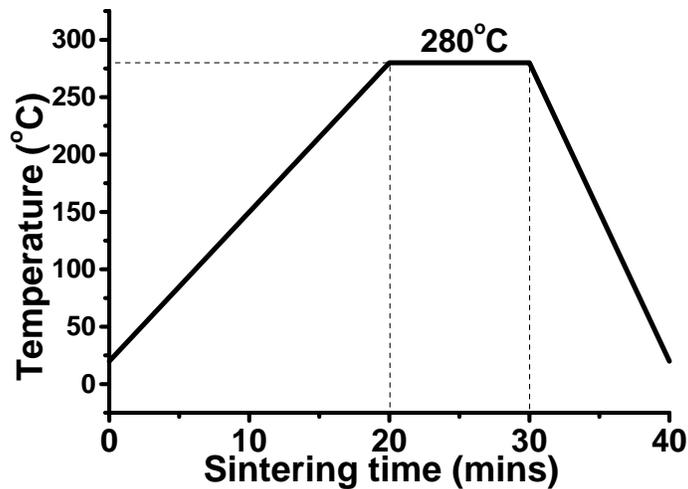
Figure 2.6. Typical temperature profile for sintering nanoscale silver pastes.
