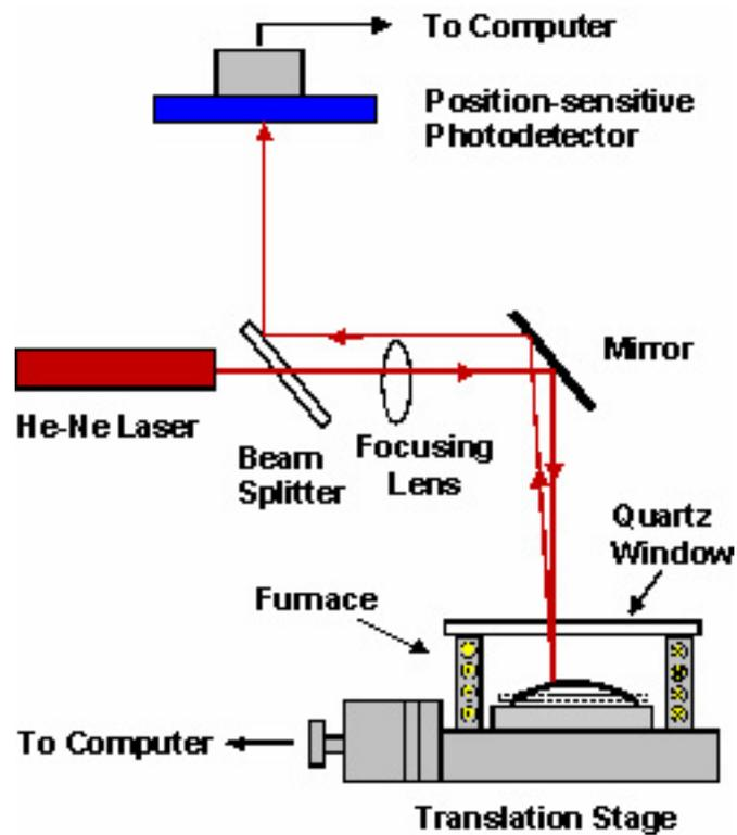
Figure 2.18. The schematic of optical setup for measuring the curvature of bi-layer composite during thermal heating.
