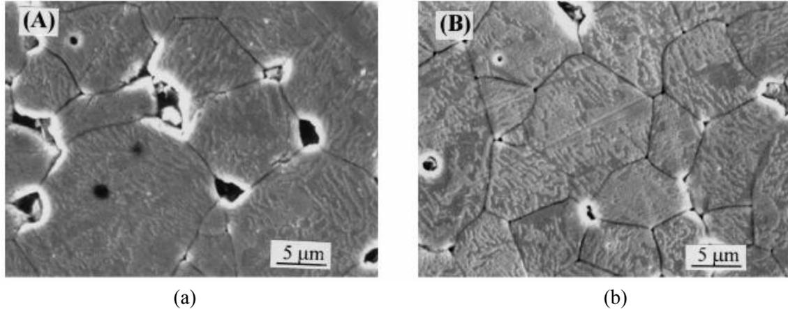
Figure 1.24. The SEM micrographs of PZT sintered at 1150°C for 2 hours in air: (a) with the heating rates of 0.5°C/min and (b) 100°C/min [57].
