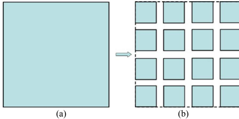
Figure 3.32. Illustration of using small patterns for the enhancement of organic burnout and paste sintering for large area silver bonding.
