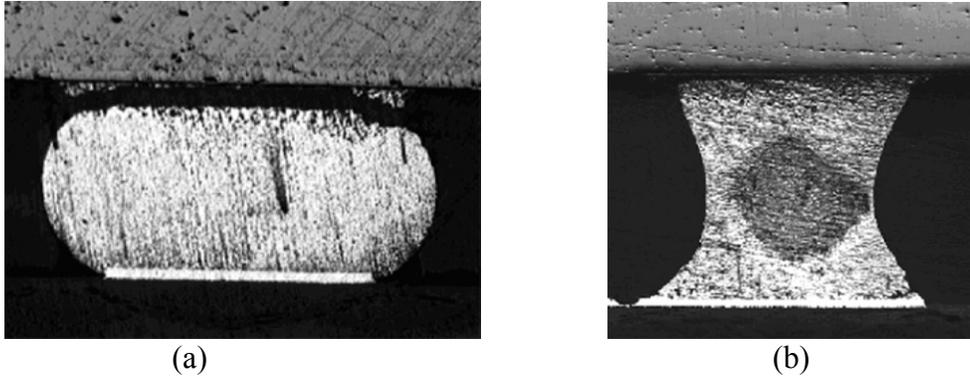
Figure 1.27. The solder bump failure after thermal cycling. (a) Barrel-shaped solder joints and (b) hourglass-shaped solder joints [63].
