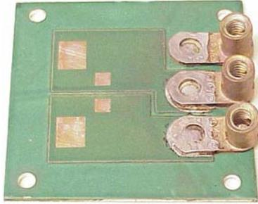
Fig. 8 An IMS after etching, solder mask patterning process and attaching power outlets.
