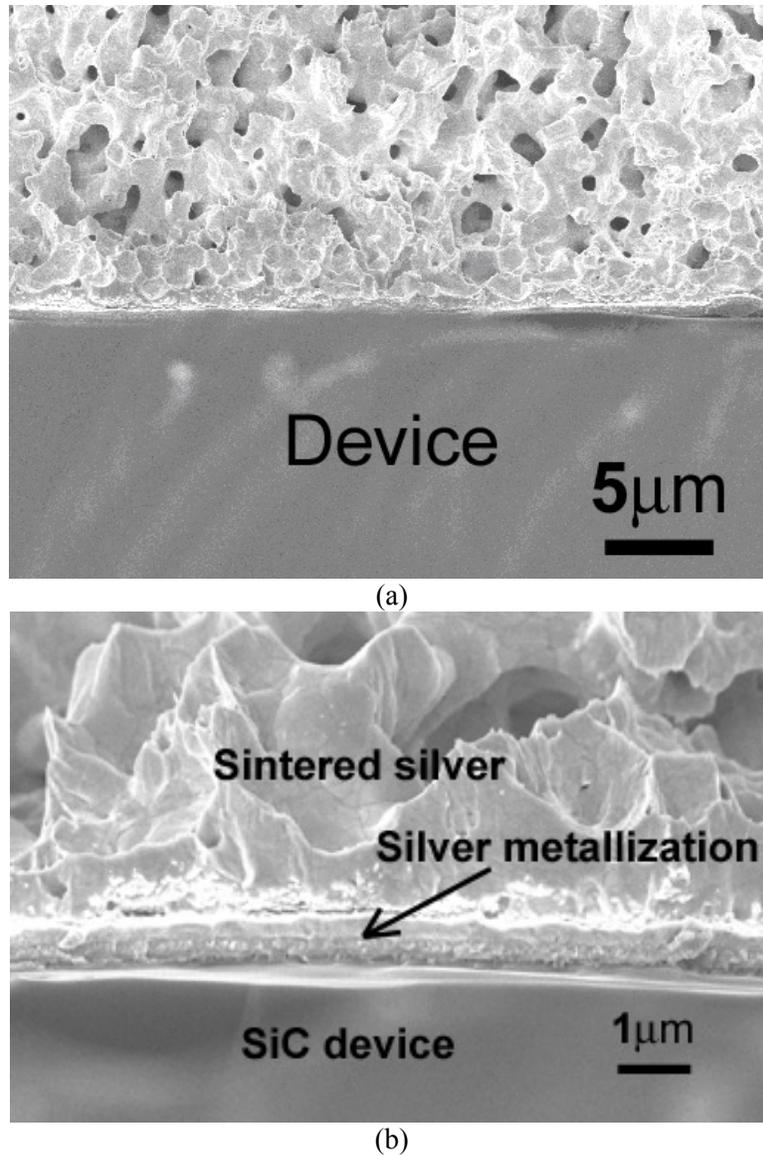
Figure 3.43. Scanning electron microscope pictures of the cross-section of the sintered silver joints.
