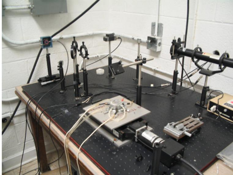
Figure 2.17. The optical setup for measuring the curvature of bi-layer composite during thermal heating.
