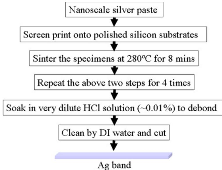
Figure 2.12. Preparation steps of the sintered silver band-shaped samples for the tensile tests.
