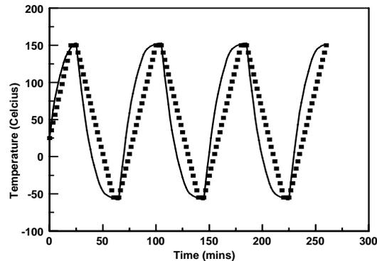
Fig. 2. Temperature profiles for the thermal cycling experiment. Solid line: experimental temperature profile; Squares: temperature datum inputs for the thermal cycling FEA simulation.
