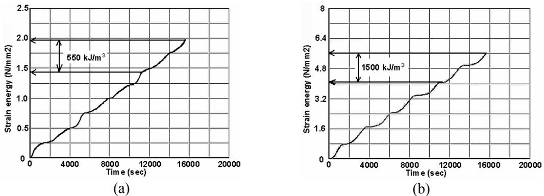
Fig. 9. The average inelastic strain energy density accumulation at the corner elements of the SB (a) and DS (b) interconnections, respectively, during the first three thermal cycles.
