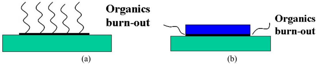
Figure 3.26. The organic components are more difficult to burn out in covering case (b) than in the open-air case (a).
