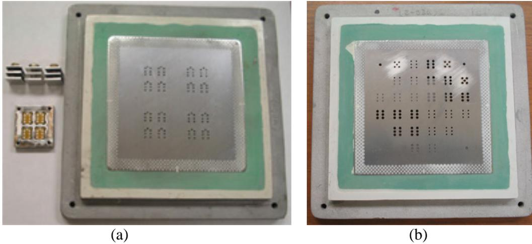
Figure 4.4. The stencil masks and fixtures used for stencil-printing silver paste. (a) The stencil pattern designed for the IXSD35N120A bare dies, and (b) the pattern for the drain terminals of the silver joints.
