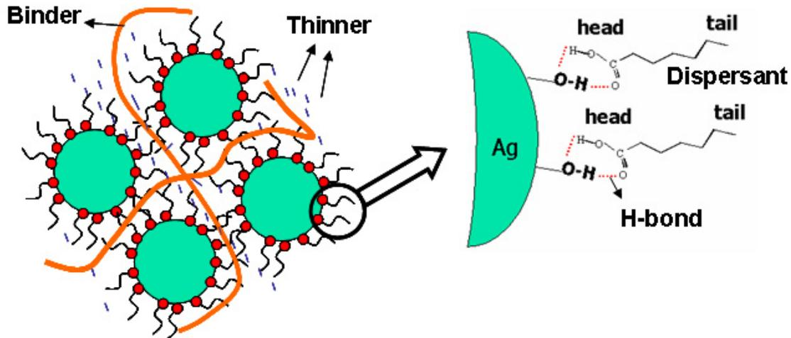
Figure 2.1. Functions of the dispersant, binder and thinner in the formulation of nanoscale silver pastes.
