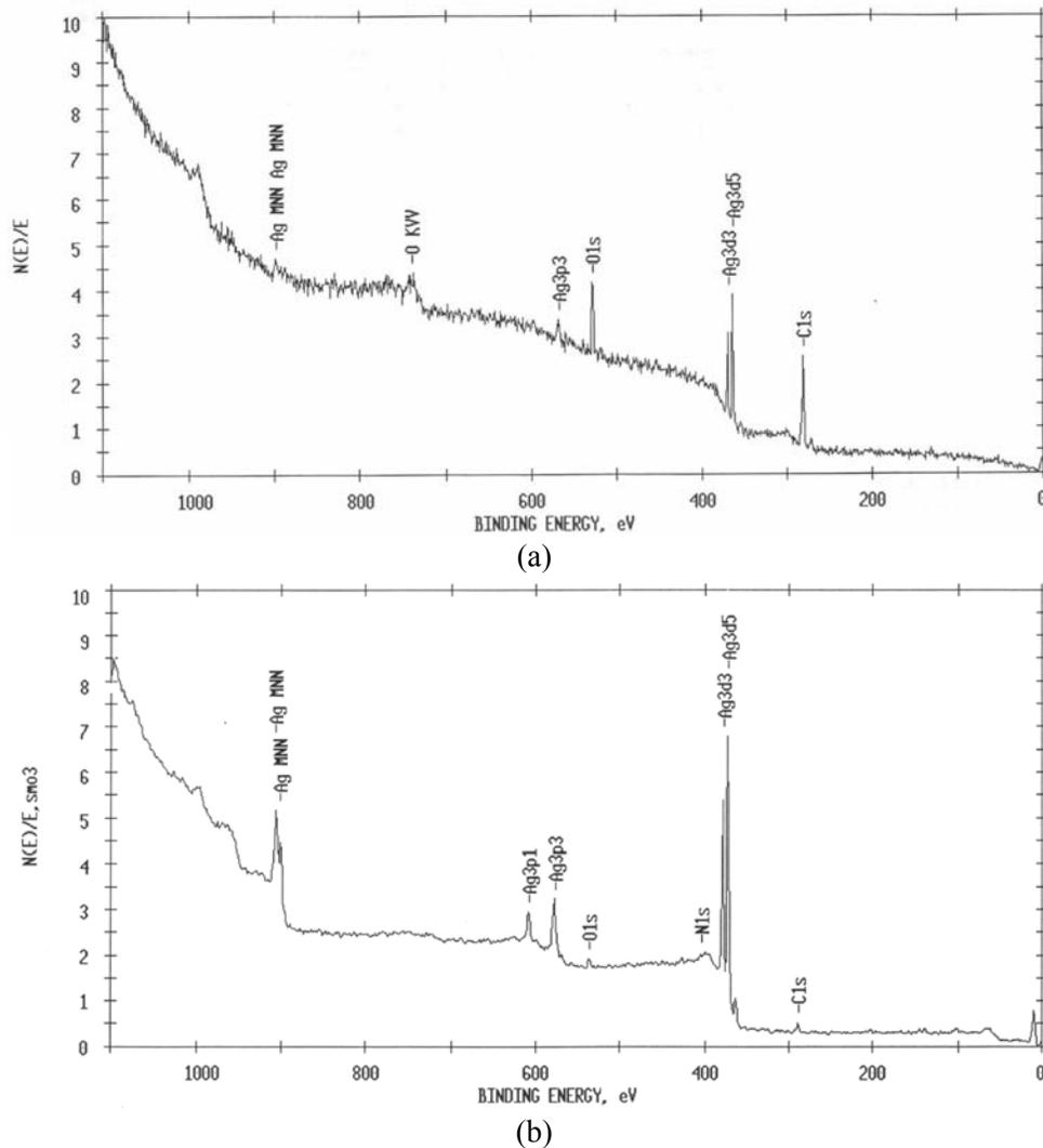
Figure 3.9. XPS analysis of the as-prepared 78 wt.% silver paste (a) and that of after the low-temperature sintering (b). Compared (b) to (a), it was found that the carbon and oxygen were reduced more than 90% during the low-temperature sintering.
