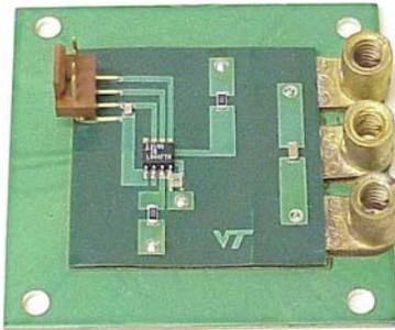
Fig. 9 A completed half-bridge FCOF-IPEM module.
