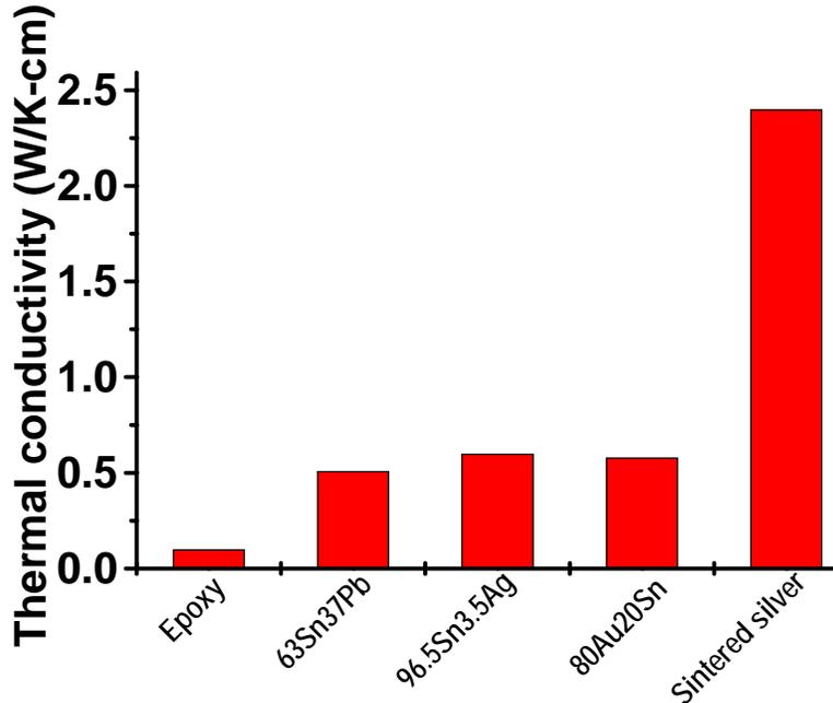
Figure 3.19. Comparison of thermal conductivity values of the common-used interconnecting materials with that of the sintered silver.
