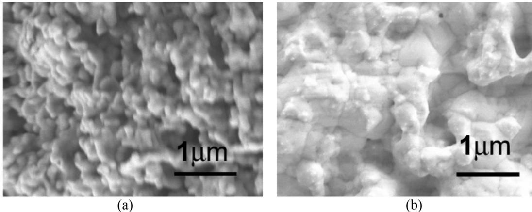
Figure 3.28. The comparison of the microstructures of unsintered silver (a) with those of sintered silver (b).
