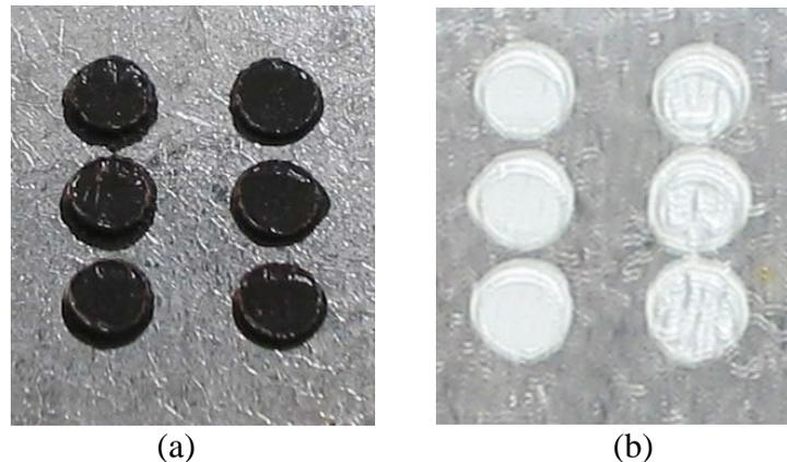
Figure 4.9. The stencil-printed silver paste patterns on nickel/silver coated DBC substrates (a) and those after the low-temperature sintering (b).
