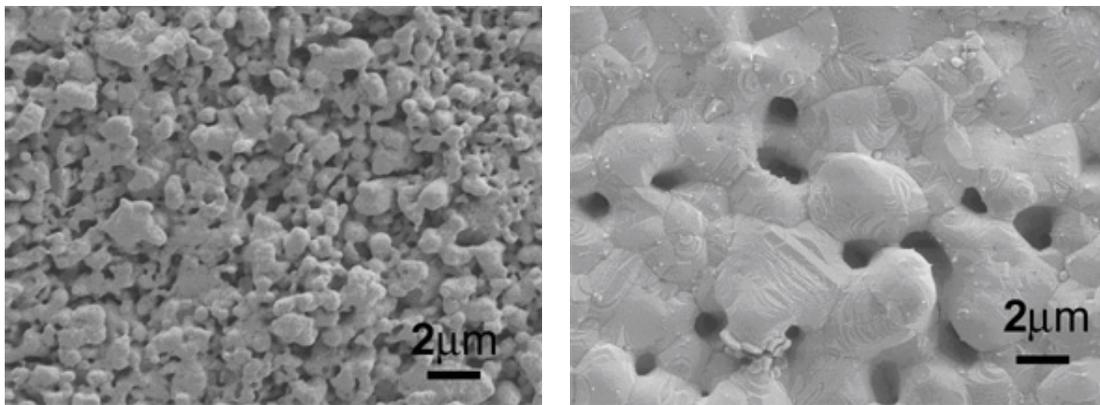
Figure 3.16. The microstructure evolution of the microscale silver paste before (a) and after (b) the heat treatment during the electrical resistivity measurement.
