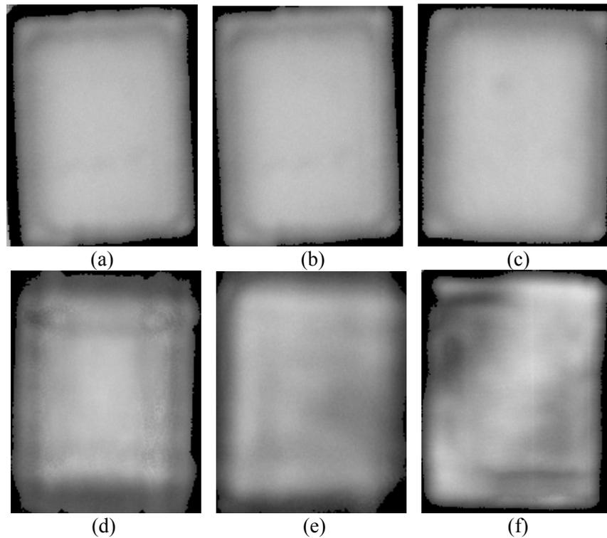
Figure 3.48. SAM images of the sintered silver joints on nickel/gold-coated  $\text{Al}_2\text{O}_3$  DBC after 0 (a), 1000 (b), 2000 (c), 4000 (d), 6000 (e), and 8000 (f) thermal cycles, respectively.
