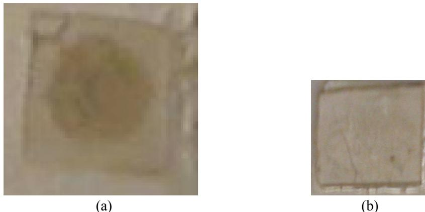
Figure 3.31. The 84 wt.% silver paste sintering under a  $6 \times 6 \text{ mm}^2$  glass slide (a) and that under a  $3 \times 3 \text{ mm}^2$  glass slide coverage after 5-min dwell at  $300^\circ\text{C}$ .
