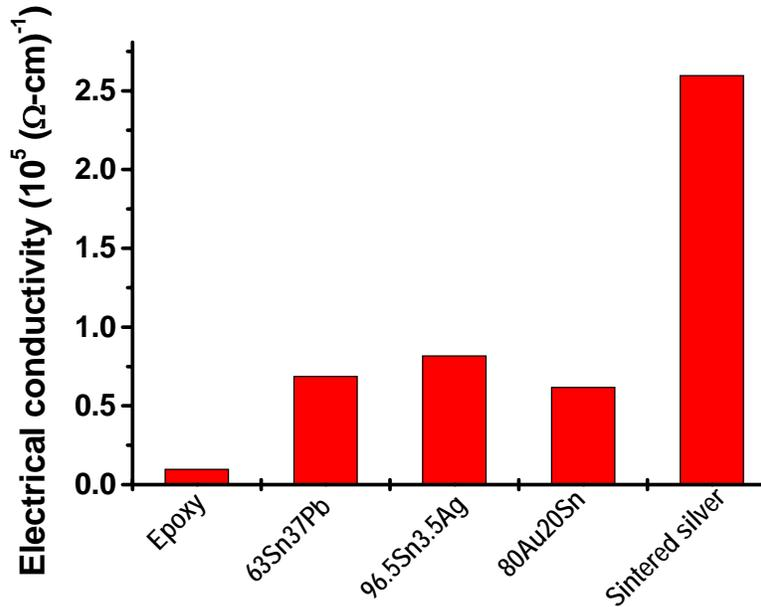
Figure 3.17. Comparison of electrical conductivity values of the common-used interconnecting materials with that of the sintered silver.
