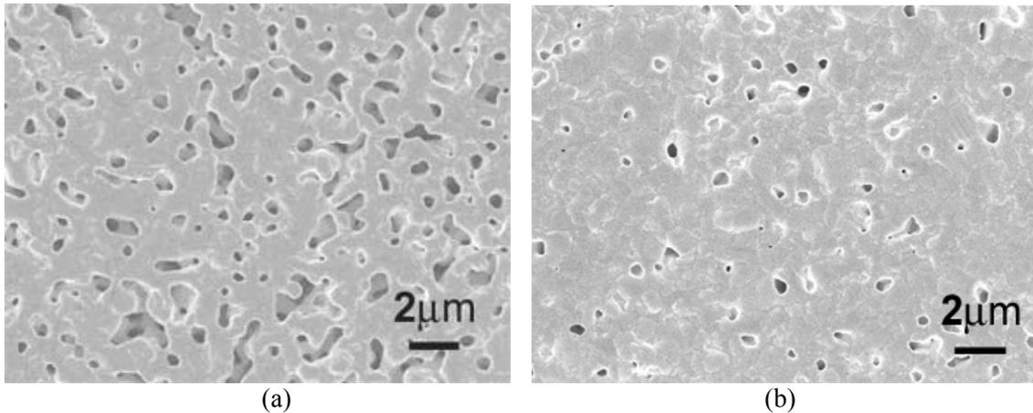
Figure 3.12. Microstructures of the low-temperature sintered nanoscale silver (a) by follows the profile in Figure 2.6 and (b) abrupt sintering, respectively.
