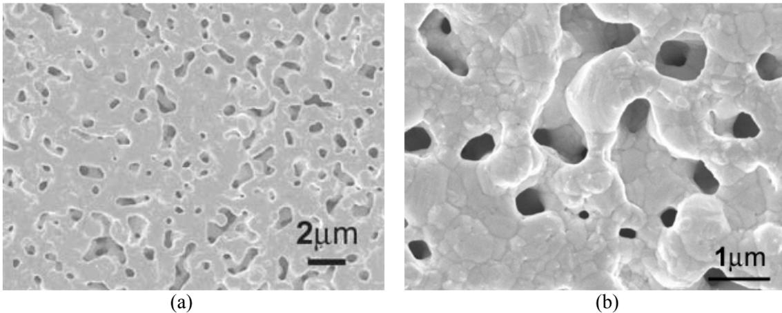
Figure 3.11. Microstructure of the low-temperature sintered nanoscale silver on an alumina substrate (top surface of a sintered film with thickness about 1 mil). (a) at 10 Kx and (b) 50 Kx.
