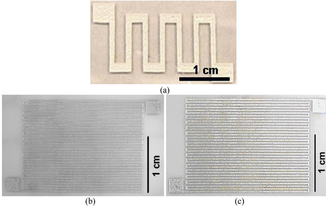
Figure 3.8. Screen-printed and low-temperature sintered silver patterns on alumina substrates.
