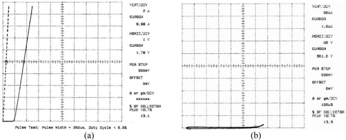
Figure 3.34. Forward (a) and reverse (b) I-V curves obtained from the Infineon devices. Dashed curve in (a) is due to the test fixture.
