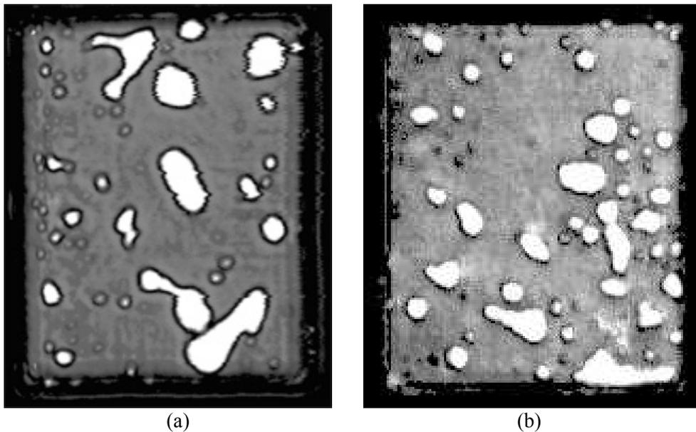
Figure 1.26. The initial void problems in the reflowed die-attaching solder layers in (a) lead-tin solder and (b) lead-free solder.
