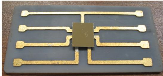
Figure 4.8. Flip die-attached IXSD1765 on the nickel/gold coated DBC substrate.
