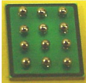
Figure 1.12. Die-dimensional BGA power packages developed in CPES [10].
