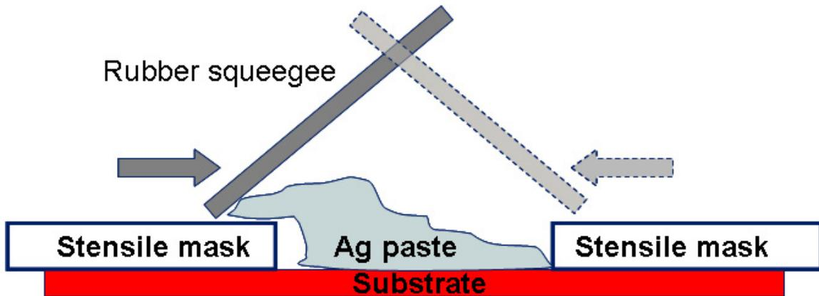
Figure 2.23. Illustration for the stencil printing process.
