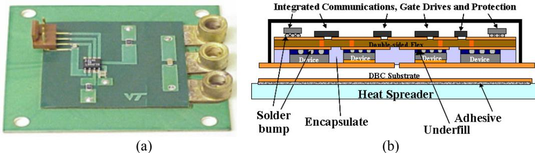
Figure 1.13. A Flip-chip on flex integrated power electronics module (a) and its schematic structure (b) [11].
