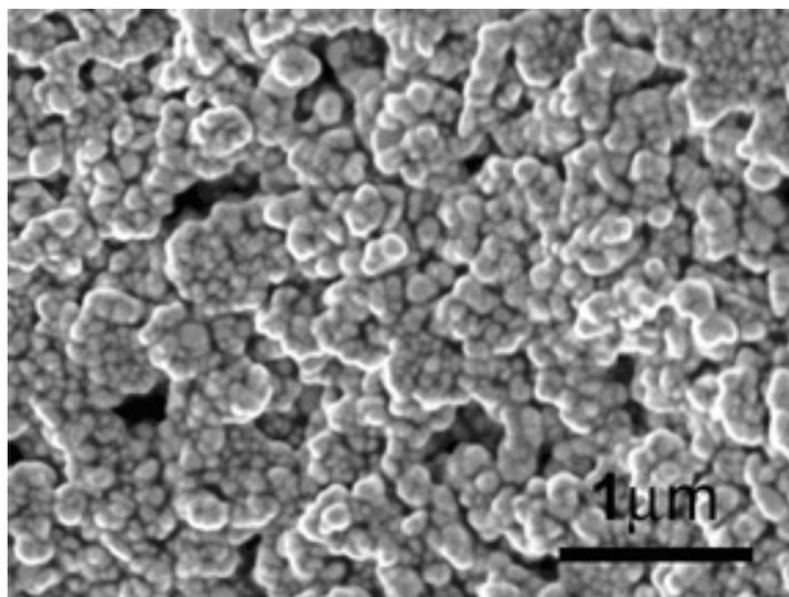
Figure 3.3. Scanning electron microscopy of the as-prepared 78 wt.% nanoscale silver paste.
