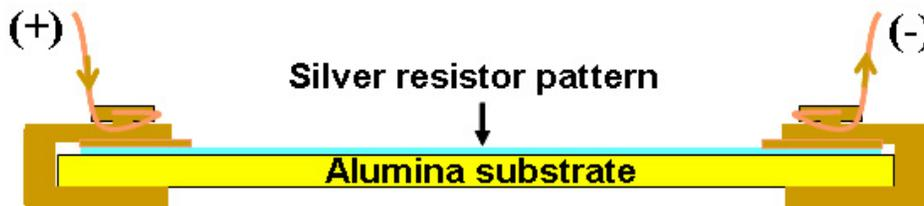
Figure 2.9. Illustration of electrical resistivity determination from printed resistor patterns.
