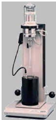
Figure 2.15. The quartz dilatometer used for the CTE measurement.
