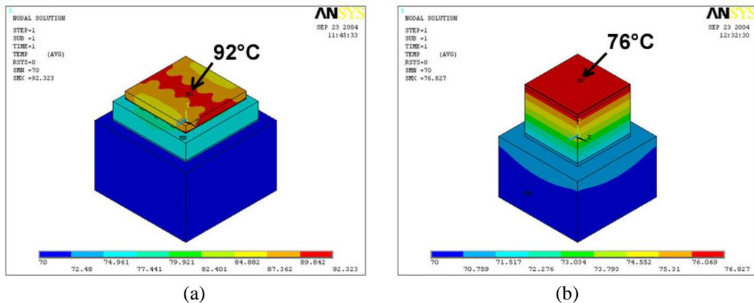
Figure 4.14. FEM thermal modeling of the temperature distributions in our proposed LED package versus the flip-chip LED package.
