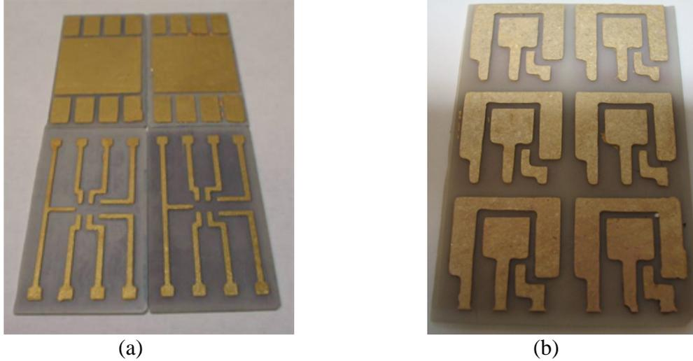
Figure 4.7. The etched and nickel/gold coated DBC substrates for the IXSD35N120A dies (a) and those for the IXSD1765 dies (b).
