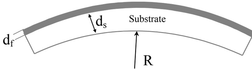
Figure 2.16. Deformation of a film–substrate bilayer composite.
