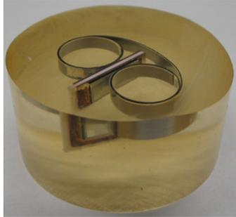
Figure 2.31. A silver joint specimen molded in cured epoxy for polishing and inspection.
