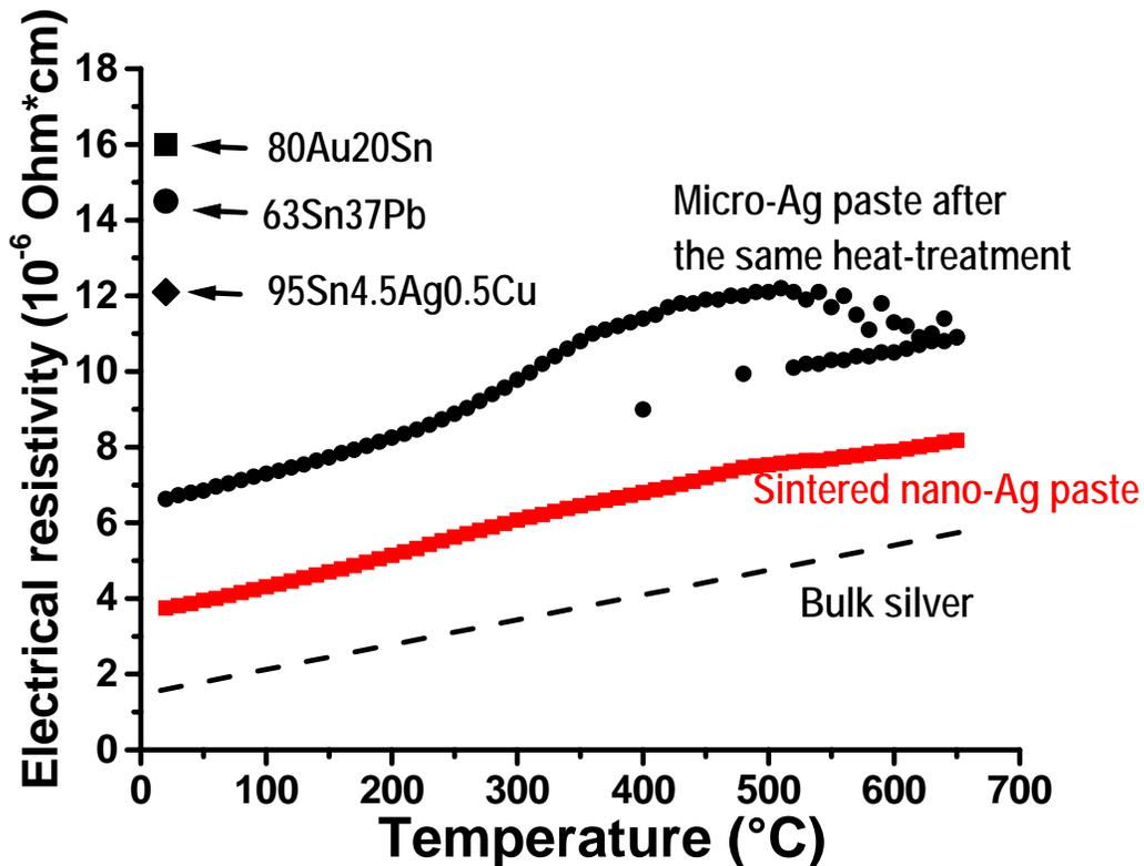
Figure 3.14. Comparison of electrical resistivity of several possible materials for semiconductor device interconnection.
