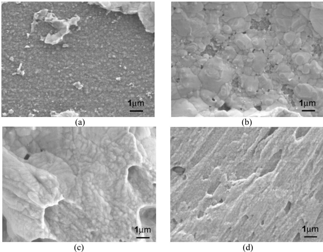
Figure 3.39. Microstructures of the debonded sintered silver joints on the silver-coated SiC devices after dwelling sintering at 300°C for (a) 10 mins, (b) 20mins, (c) 40mins, and (d) 60 mins.
