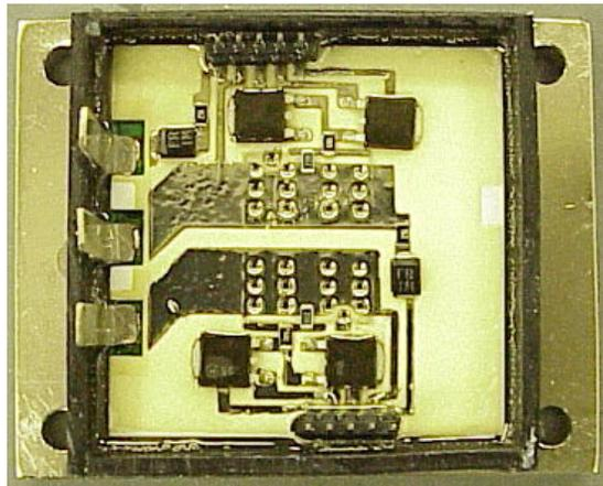
Figure 1.6. An IPEM packaged by the embedded power technology [3].
