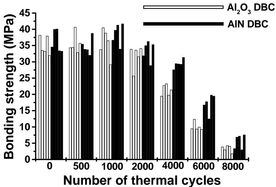
Figure 3.51. Changes of shear strength of the low-temperature sintered silver joints on nickel/silver-coated DBC substrates during the temperature cycling experiment.
