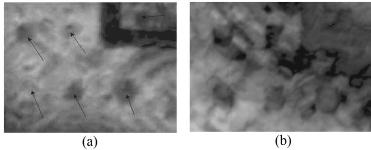
Fig. 5. SAM images of the SB interconnections in a failed SB package taken after 875 thermal cycles. (a) At the solder/power device interface and (b) at the solder/DBC copper interface.
