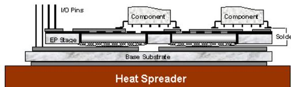
Figure 1.5. Cross-sectional schematic of embedded power module [3].
