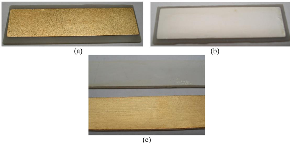
Figure 2.22. Nickel/gold (a) and nickel/silver (b) coated AlN DBC and the nickel/silver and nickel/gold coated copper substrates (c).
