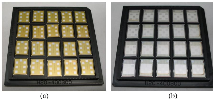
Figure 4.2. The IXYS bare dies used for single-chip power packaging demonstration. (a) Bare power IGBTs with type # of IXSD35N120A; (b) Bare power IGBTs with type # of IXSD1765.
