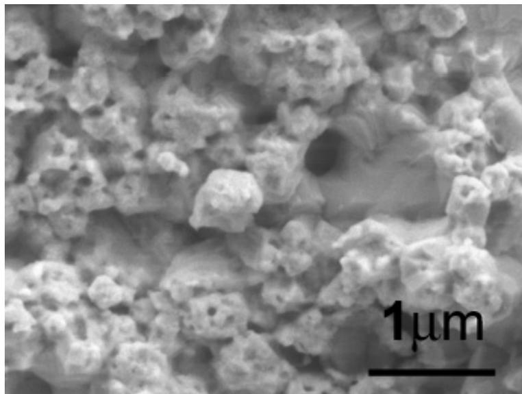
Figure 3.56. Microstructure changes of the debonded sintered silver joint surfaces after 4000 thermal cycles. The silver joints were debonded from the nickel/silver aluminum-oxide DBC substrates.
