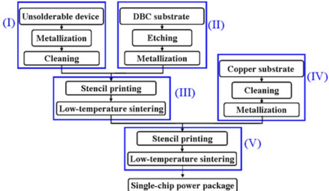
Figure 4.3. The fabrication steps for the silver jointed single-chip power packages.
