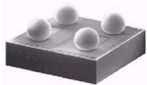
Figure 1.11. IR's FlipFET power MOSFET [9].
