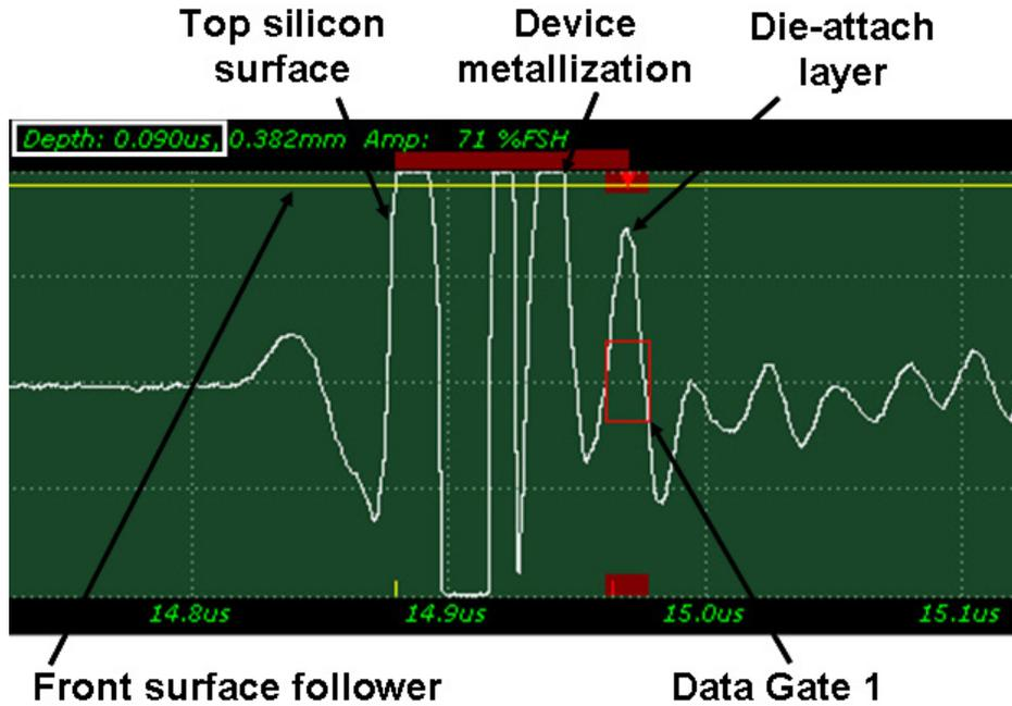
Figure 2.29. A typical scan SAM image of an Infineon SiC device die-attached silver joint.
