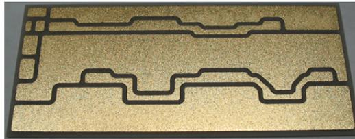
Figure A.3. An nickel and gold electroless-plated aluminum nitride DBC substrate sample.
