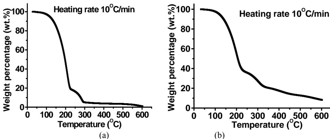
Figure 2.2. Thermogravimetric analysis (TGA) curves of the thinner (a) and binder (b) selected for the silver paste formulation. Heat treatment condition is 10°C/min in air. Note the quick weight percentage drops at temperatures below 300°C.
