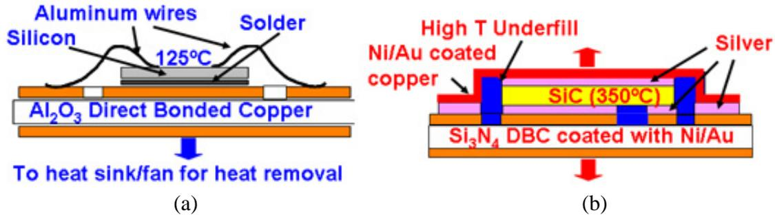
Figure 4.1. The solder die-attaching and wire-bonding technology (a) versus the low-temperature silver sintering technology (b).
