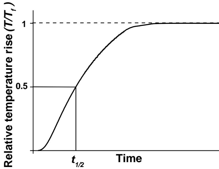
Fig. 1. A typical temperature transient curve at the rear surface of a specimen after the laser flash.
