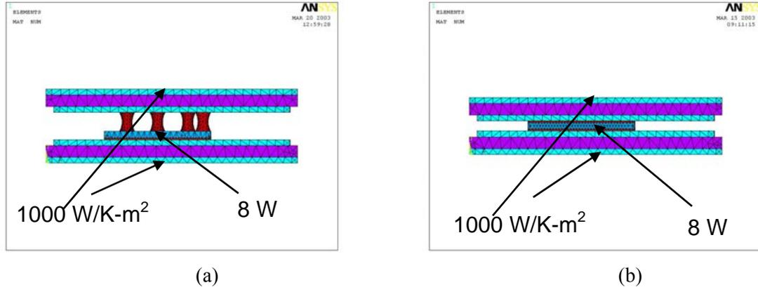
Fig. 3. The thermal FEA models for (a) the SB package and (b) the DS package.
