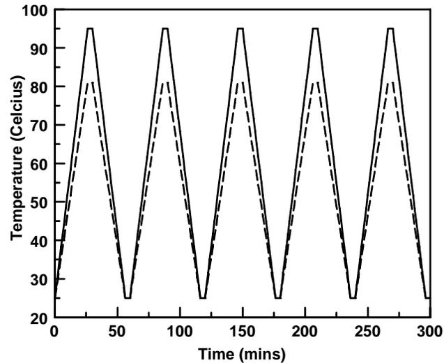
Fig. 10. Temperature profiles for power cycling simulation. Solid line for the SB package and dashed line for the DS package.
