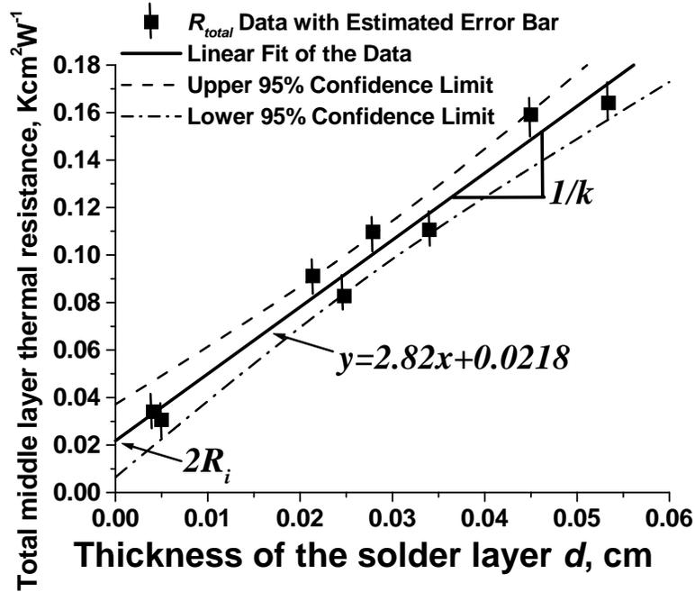
Fig. 3. Total thermal resistance  $R_{total}$  of solder in the tri-layered specimens as a function of the solder layer thickness.
