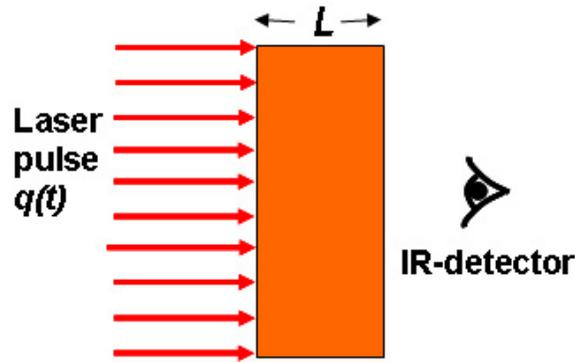
Figure 2.11. Illustration of the laser-flash experiment.
