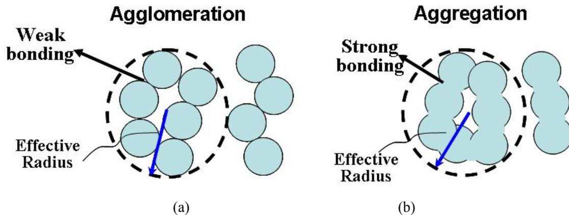
Figure 1.21. Illustration of agglomeration (a) and aggregation (b) and their effective particle sizes.
