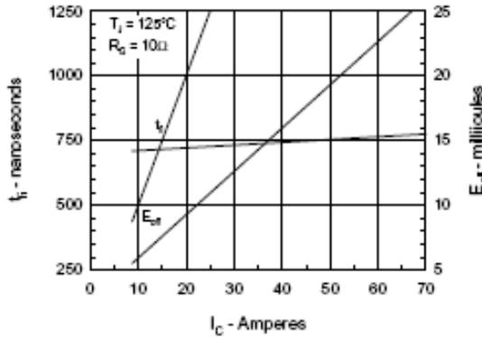
**Fig.8 Dependence of Turn-Off Energy Per Pulse and Fall Time on  $R_{\theta C}$**
