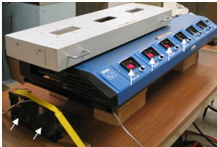
Figure 2.33. The Sikama belt reflow oven adapted for the 50-250°C thermal cycling experiment. The four perpendicular arrows in the middle show the four of the total five slots were set to be 280°C. The fifth is left for cooling and the last window is for setting the cycling speed. The two arrows in the lower left corner indicate the two blowing fans for cooling down.
