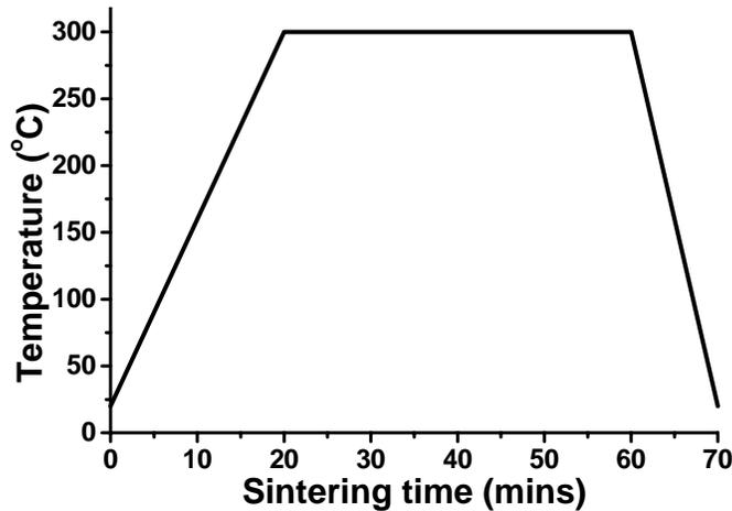
Figure 2.25. The sintering profile for achieve high bonding strength in the silver joints.
