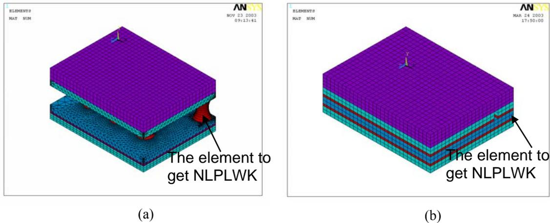
Fig. 8. The finite element models of the SB (a) and DS (b) packages used in the transient thermomechanical analysis to simulate both thermal and power cycling experiment.
