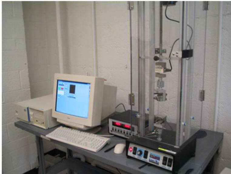
Figure 2.13. Setup of ComTen tensile test machine.
