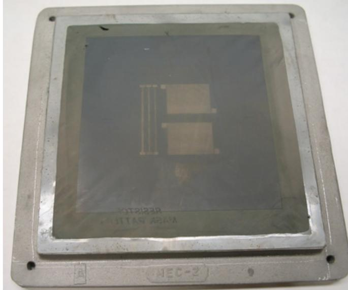
Figure 2.7. Screen was used for printing resistor patterns.
