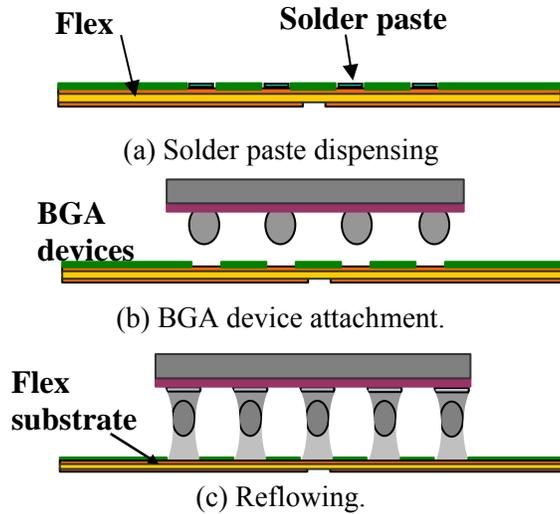
Fig. 5 The three steps of flip-chip bonding.
