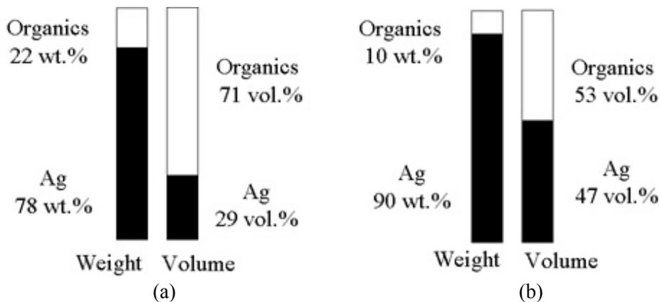
Figure 2.5. The weight and volume percentages of the 78 wt.% silver paste (a) and those of the 90 wt.% silver paste (b).
