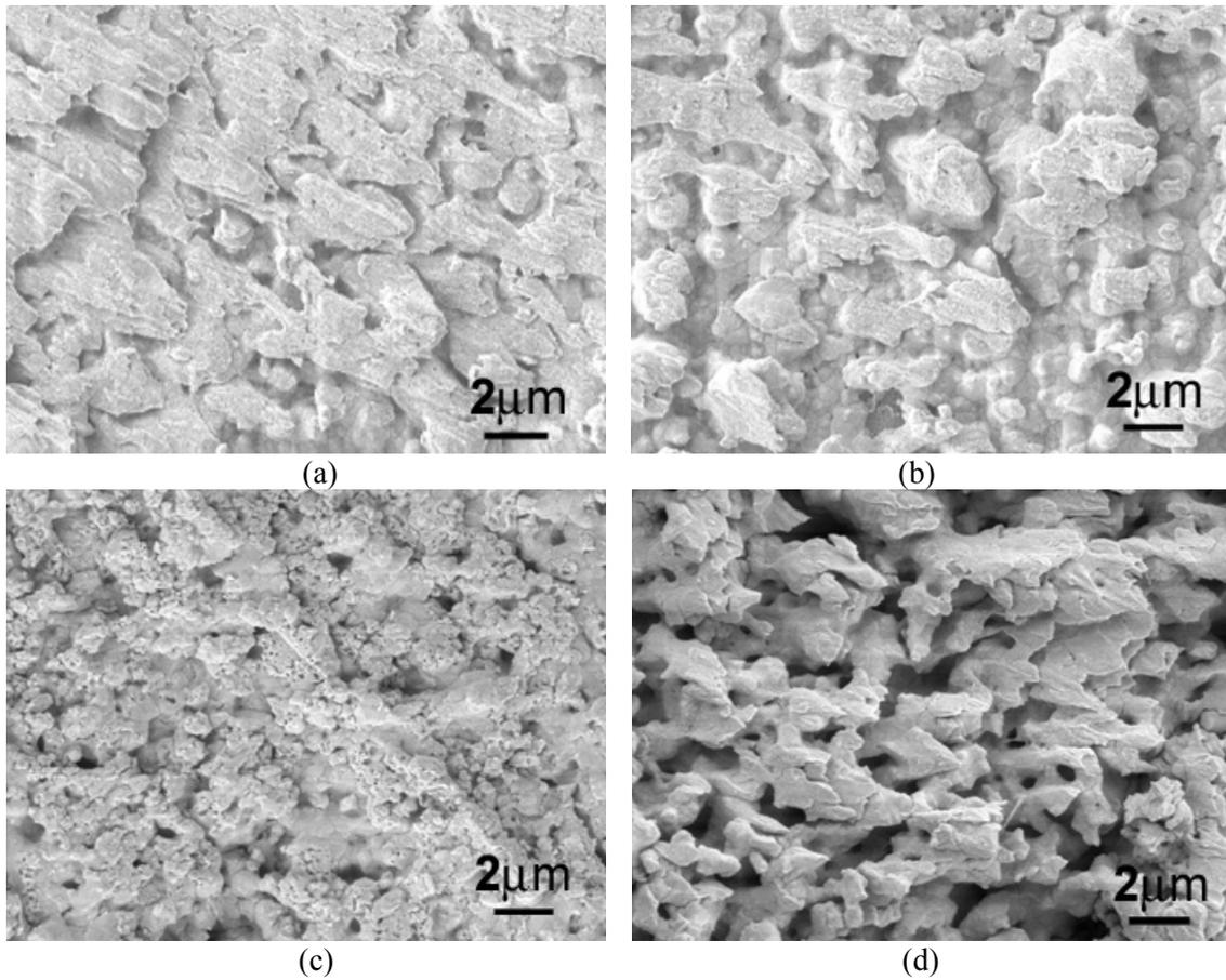
Figure 3.55. Microstructures of the debonded sintered silver joints on the silver-coated SiC devices after (a) 0, (b) 2000, (c) 4000, and (d) 6000 cycles. The silver joints were debonded from the nickel/silver aluminum-nitride DBC substrates.
