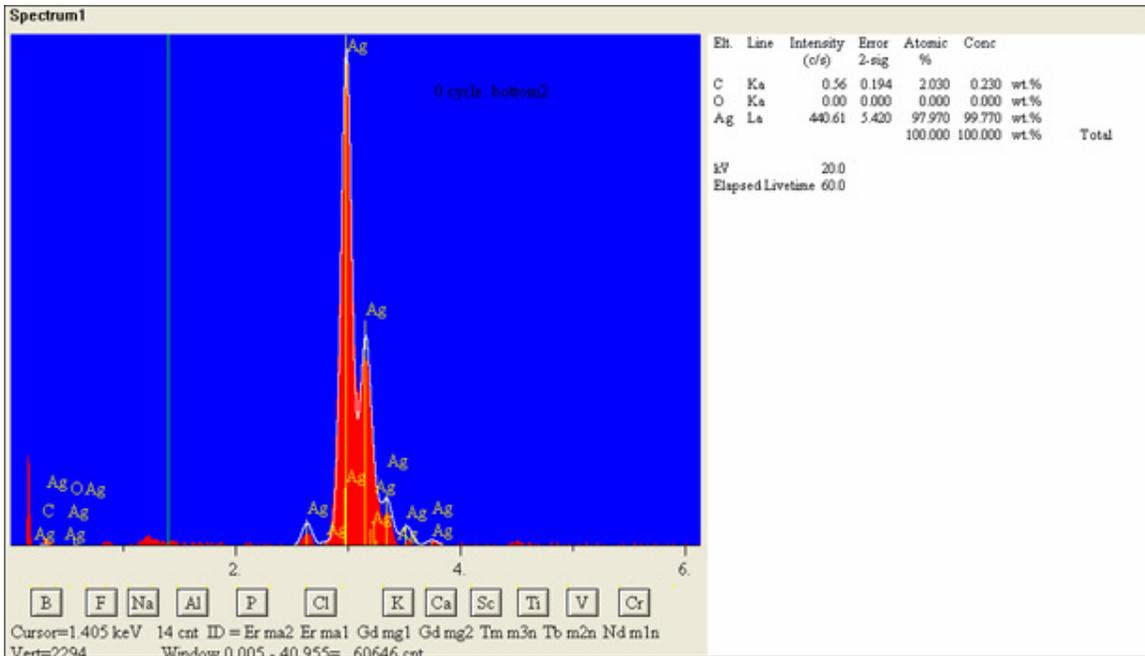
Figure 3.10. EDS analysis of the 78 wt.% silver paste after the low-temperature sintering. Silver is about 99.77 wt.% after the low-temperature sintering and the rest of the sintered silver is carbon (~0.23 wt.%). There is no detectable oxygen left.
