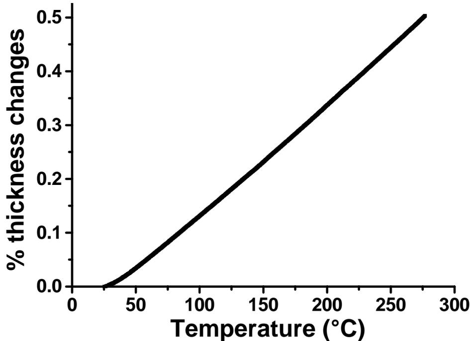
Figure 3.23. A typical thickness change-temperature curve of the quartz dilatometry test.
