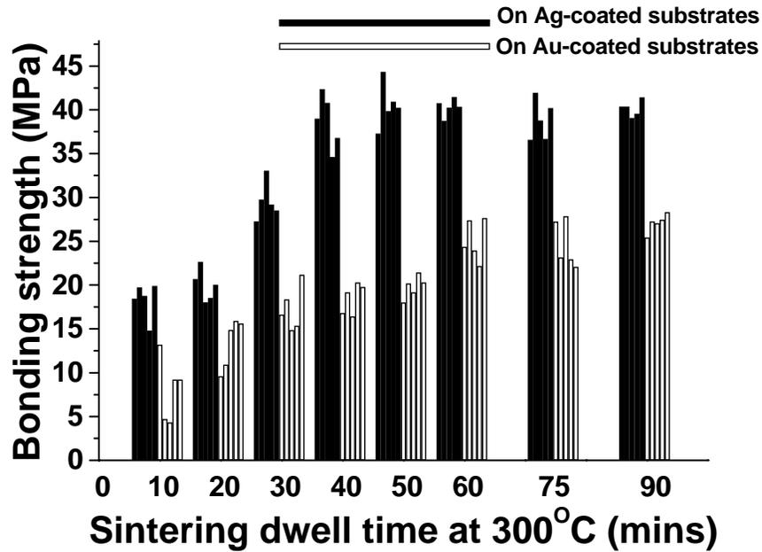
Figure 3.38. The bonding strength development versus the sintering dwell time.
