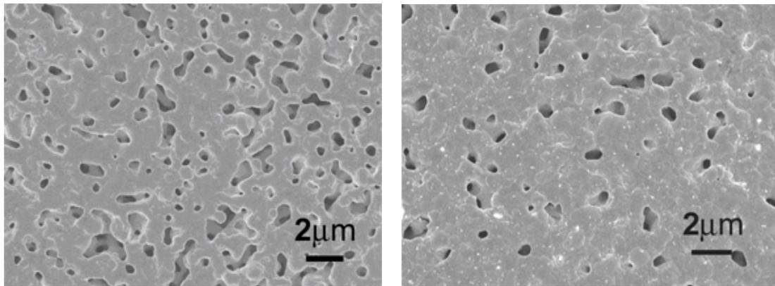
Figure 3.15. The microstructure evolution of the nano-silver paste before (a) and after (b) the heat treatment during the electrical resistivity measurement.
