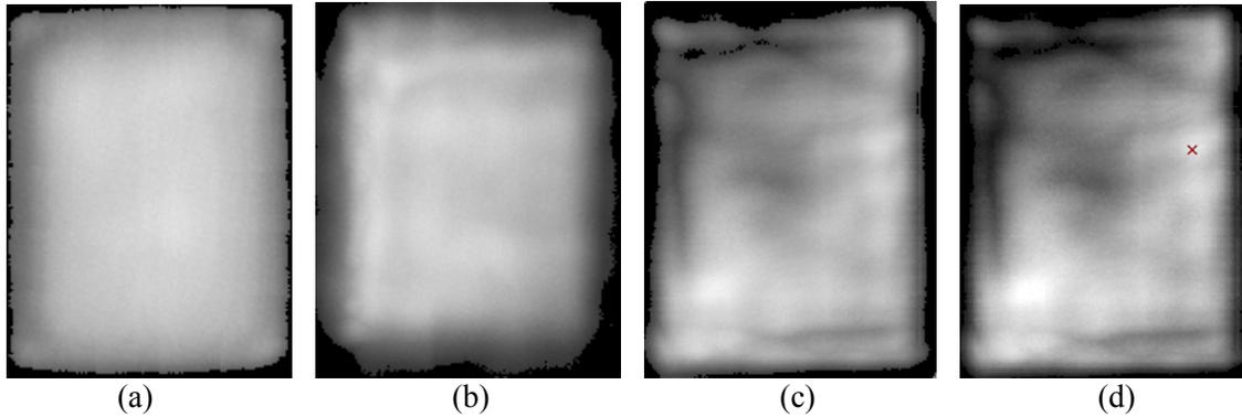
Figure 3.50. The SAM images of the sintered silver joints on nickel/silver-coated copper substrates after 0 (a), 500 (b), 1000 (c), and 2000 (d) thermal cycles, respectively.
