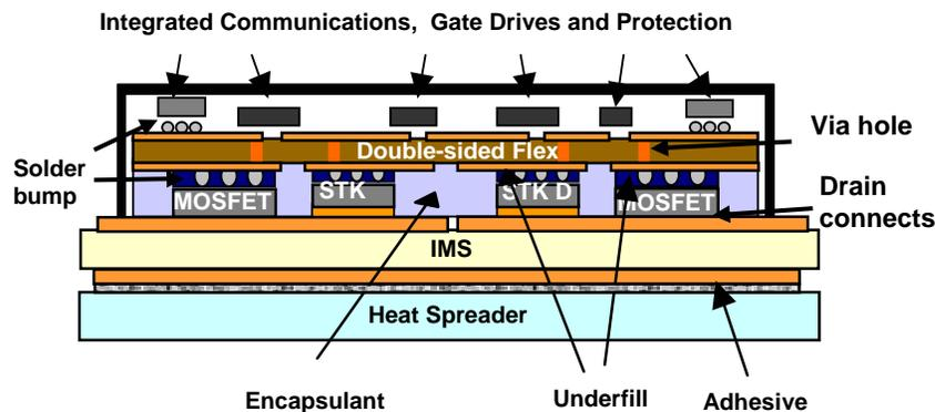
Fig. 1. Schematic structure of an FCOF-IPEM built using solder-bumped power devices.
