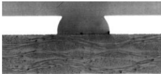
Figure A.1. The over-etch phenomena during the isotropic etching of DBC substrates. For the etching of 0.3 mm DBC Cu layer, the over-etching is about 0.1 mm (100  $\mu\text{m}$ ).
