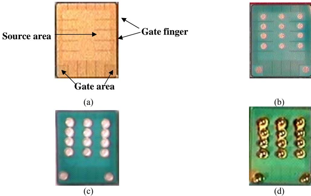
Fig. 3 (a) A commercial unsolderable power MOSFET from IXYS. (b) The MOSFET after solder-mask process. Except the gate and source pads, the entire surface is covered by solder mask. (c) The MOSFET after UBM sputtering process. (d) The solder-bumped MOSFET.
