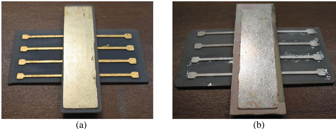
Figure 4.10. The finished single-chip power packages for the IXSD35N120A devices (a) using the nickel-gold plated DBC substrates and (b) the nickel-silver plated DBC substrates.
