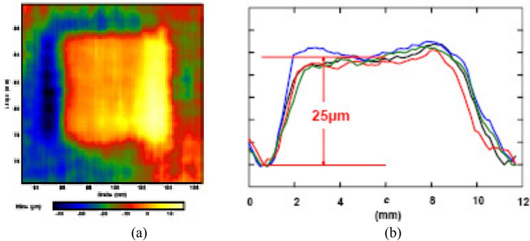
Figure 3.7. Topological image (a) and its two topological profiles (b) of the printed nanoscale silver paste after sintering.
