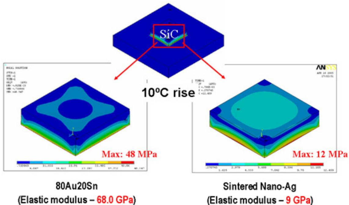
Figure 3.24. A finite element analysis shows that the sintered silver induces less thermal stresses than those of gold-tin solder.
