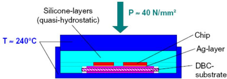
Figure 1.17. Schematic of a pressure-assisted silver paste sintering setup [26].
