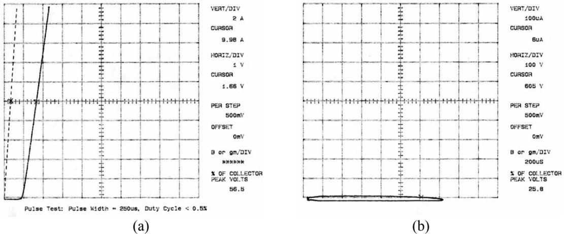
Figure 3.35. Forward (a) and reverse (b) I-V curves obtained from the CREE devices. Dashed curve in (a) is due to the test fixture.
