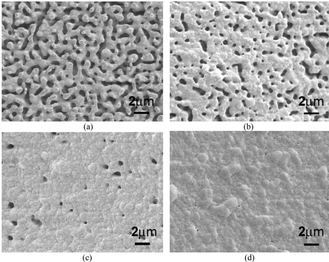
Figure 3.13. Microstructures of the low-temperature sintered nanoscale silver on a silicon substrate (a) at the silicon-silver interface, and at 1 mil (b) and 4 mil (c) away from the interface and (d) free sintering case (pill off the baked silver paste film and then sinter). All sintering profiles follow that shown in Figure 2.6.
