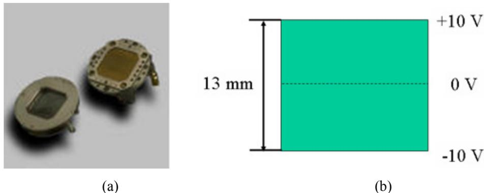
Figure 2.20. The position sensitive photodetectors used in the curvature determination optical setup (a) and their position-sensing mechanism (b).
