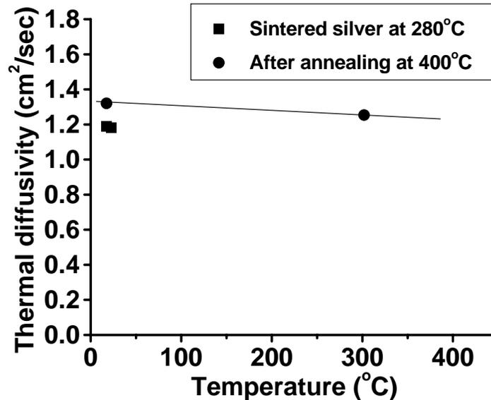
Figure 3.18. Data plot of thermal diffusivity of the low-temperature sintered silver versus temperature.
