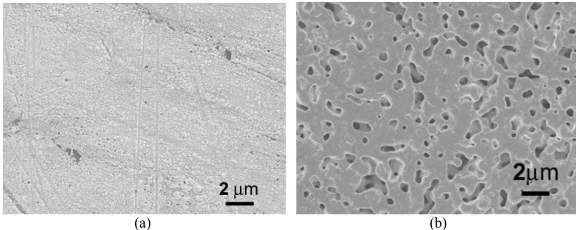
Figure 3.20. Comparison of surface microstructures of the polished samples for the thermal conductivity measurement (a) and those for the electrical conductivity measurement (b) (non-polished).
