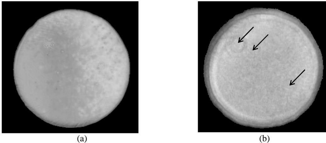
Fig. 4. SAM images of the solder/copper interface in the bi-layered specimens #4 (a) and #5 (b), respectively. Both specimens have a diameter of 1.27 cm. Arrows in (b) indicate the low density areas at the solder/copper interface.
