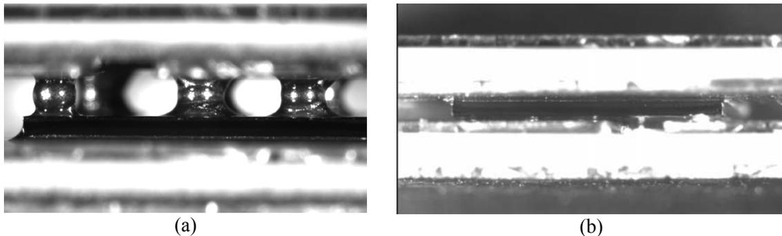
Fig. 1. (a) A SB package with the source/gate of the power MOSFET device attached to the top DBC substrate via six 1-mm-high solder-bumps, (b) a DS package with the source/gate of the device attached to the top DBC substrates via 100  $\mu\text{m}$  solder layers. Both 10X magnification.
