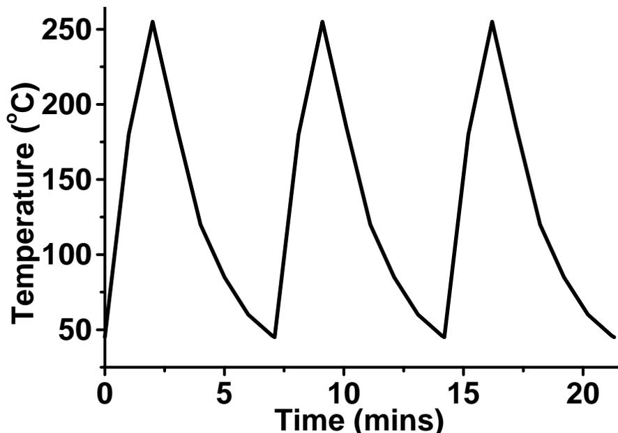
Figure 3.46. The temperature profile obtained using the Sikama belt reflow oven.
