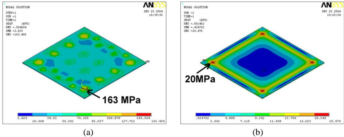
Figure 4.15. FEM modeling of thermomechanical stress distributions in the packaged LED devices versus that in the flip-chip LED device during operation (the stress-free state was assumed to be at the respective die-attach temperatures).
