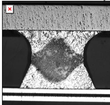
Fig. 7 SEM image of a triple stacked hourglass shaped solder bump.
