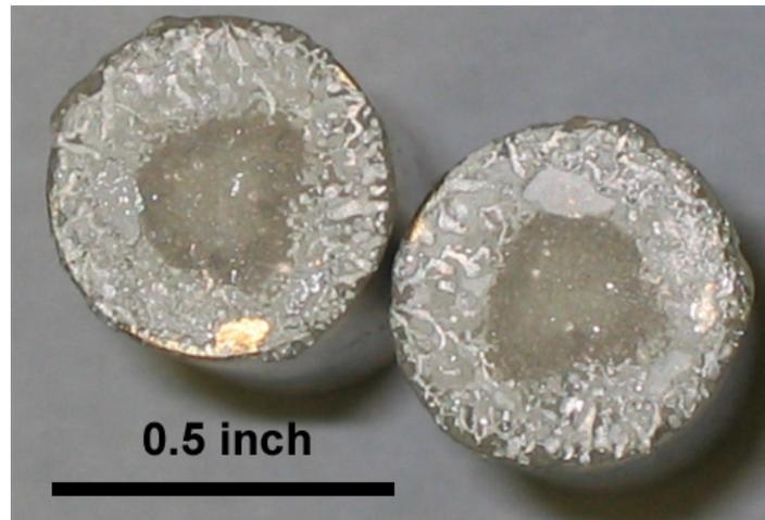
Figure 3.27. Low-temperature sintered silver at half-inch thick rod surfaces after debonding.
