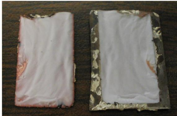
Figure 3.44. An alumina DBC substrate broken from the alumina layer between 100-200 cycles switching from 50°C to 300°C.
