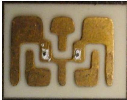
Figure 4.16. Low-temperature sintered silver die-attached LEDs. The two white parts are dispensed-silver after low-temperature sintering and the two black squares are two die-attached LEDs.
