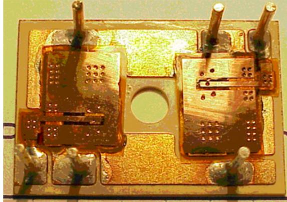
Figure 1.4. A prototype of power module packaged using power overlay interconnect technology.
