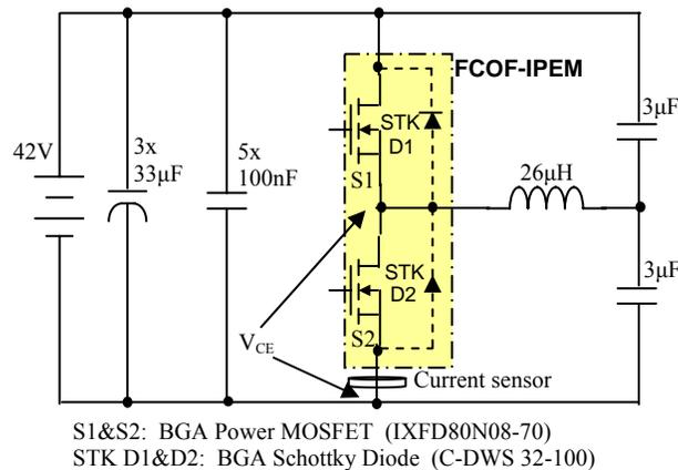
Fig. 10 Continuous switching test circuit.
