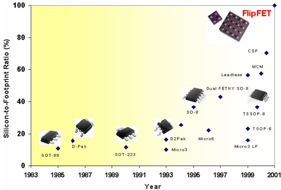
Figure 1.18. Technology roadmap of International Rectifier's chip-level discrete power packages.
