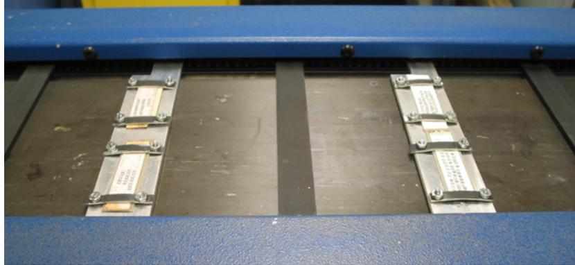
Figure 2.37. The loaded sample holders installed in the belt oven during the 50-250°C thermal cycling. The covering lid was removed for clarity.
