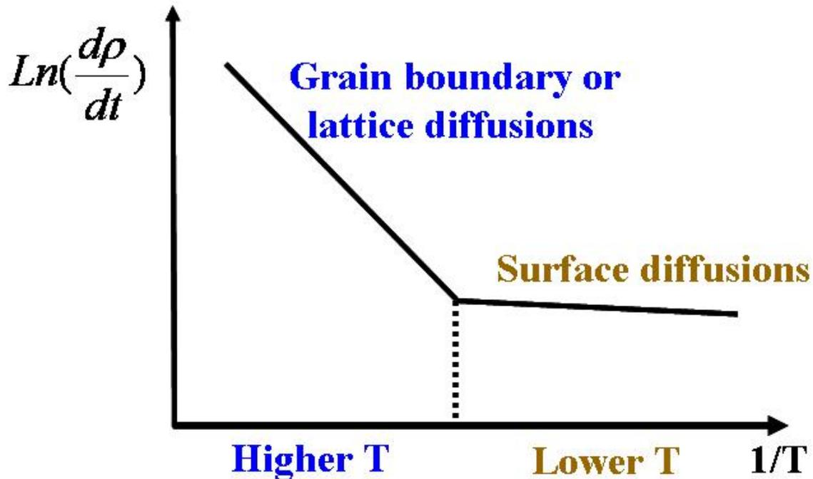
Figure 1.23. Schematic diagram of change in densification rate with temperature. According to rapid rate sintering theory, the two regimes should correspond to poor or no densification (surface) at low temperatures and much more efficient densification (via grain boundary or lattice diffusion) at high temperature [51].
