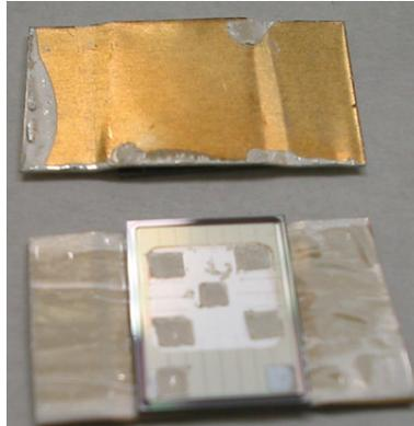
Figure 4.11. The IXSD1765 dies with the drain terminals interconnected to nickel-gold coated copper cavities.
