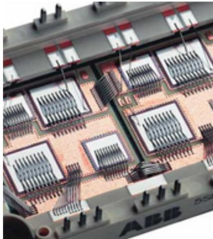
Figure 1.2. Top view of a wirebond multichip power module.
