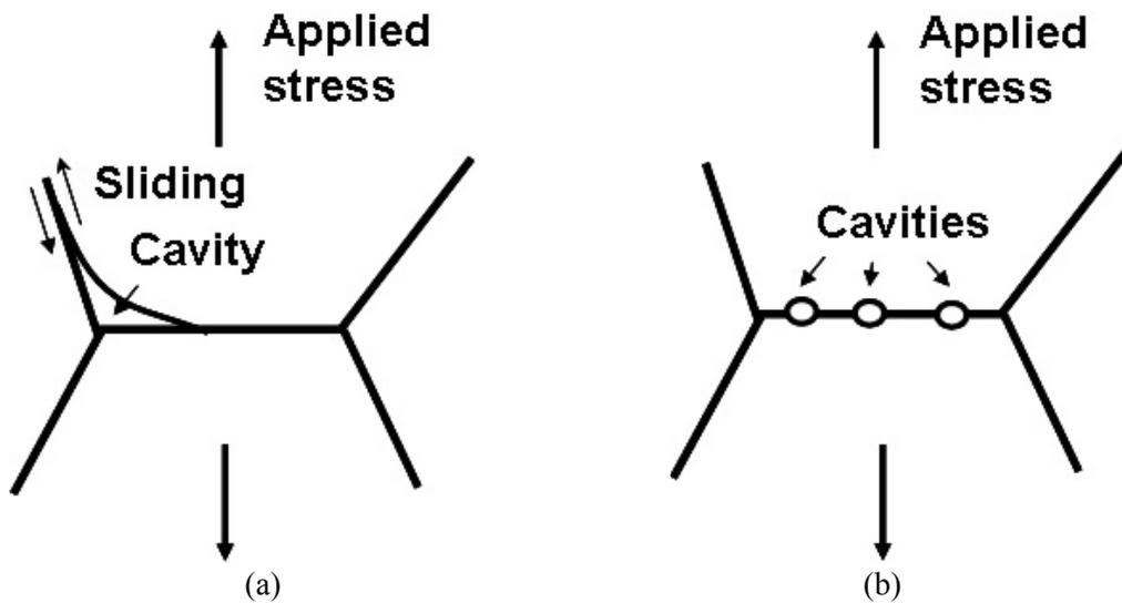
Figure 3.58. *w*-type cavitation at a grain-boundary triple point (a) and *r*-type cavitation at a grain boundary normal to the stress axis (adapted from Ref. [12], pp. 146-147).
