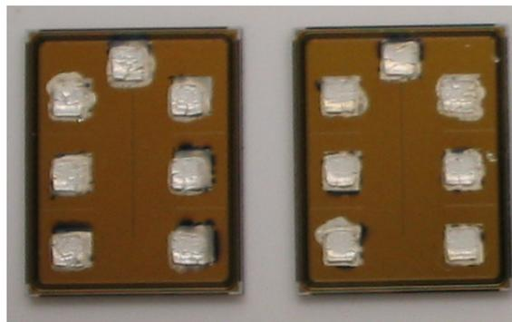
Figure 4.5. The IXSD35N120A bare dies after the sputtering metallization and low-temperature sintering of stencil-printed silver paste on the gate and source terminals. The top middle square is for gate and other six are for the source.
