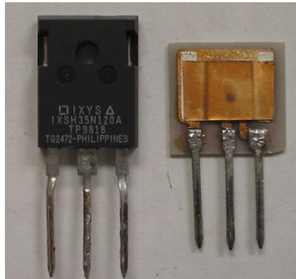
Figure 4.12. Comparison of the commercial wire-bonded single-chip power package (left, TO-247 power package) with the low-temperature sintered silver joint power package (right).
