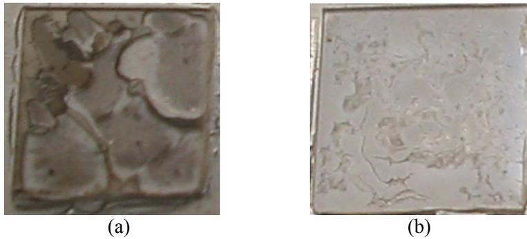
Figure 3.30. The 78 wt.% (a) and 84 wt.% (b) silver paste sintering under the  $4 \times 4 \text{ mm}^2$  glass slide coverage after 10-min dwell sintering at  $300^\circ\text{C}$ .
