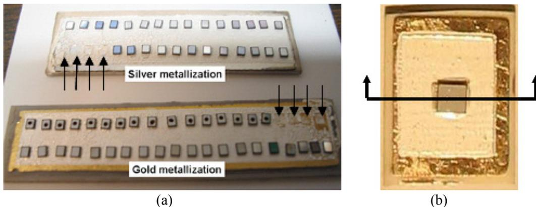
Figure 2.26. (a) Die-attached Infineon SiC devices on silver or gold-coated DBC substrates for the die-shear tests. Arrows indicate the die-attaching cavities where the devices have been sheared-off. (b) A die-attached CREE device for the cross-sectional inspections.
