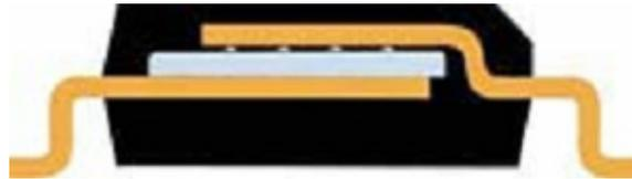
Figure 1.8. Cross-sectional view of a SO-8 Wireless chip-level power package [6].
