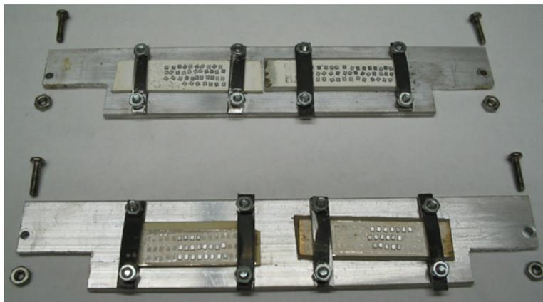
Figure 2.35. The fixture and samples used for the 50-250°C thermal cycling.
