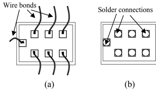
Fig. 12 Contact geometries of wire-bonds vs. flip-chip solder bump interconnections: (a) The long wire bonds with small contact areas; (b) the short flip-chip solder bumps with large contact areas (Victor).
