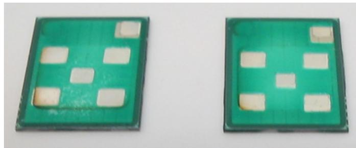
Figure 4.6. The IXSD1765 bare dies after the solder mask deposition to protect the exposed gate fingers. Note that the IXSD1765 dies are already metallized nickel/silver at the open windows for the gate and source terminals.
