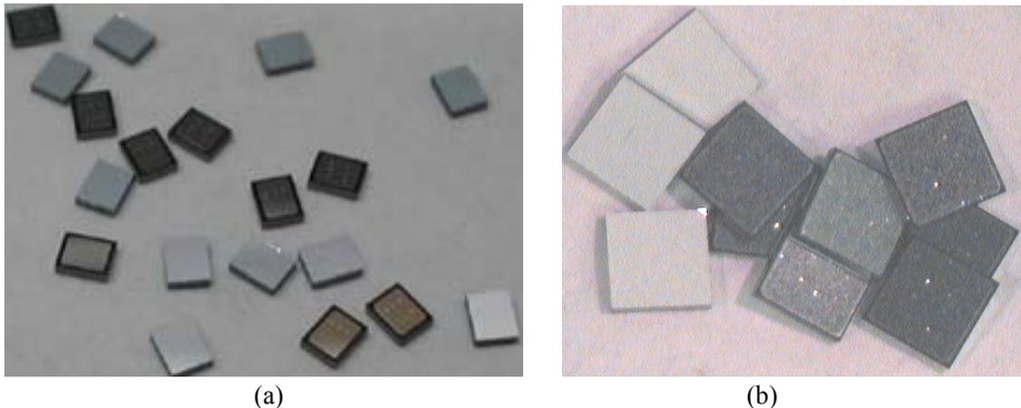
Figure 2.24. Infineon (a) and CREE (b) SiC devices used to form sintered silver joints.
