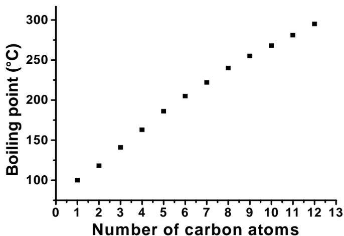
Figure 2.3. The relationship of the boiling point of fatty acid versus their number of carbon atoms (Adapted from the Sigma-Aldrich websites).
