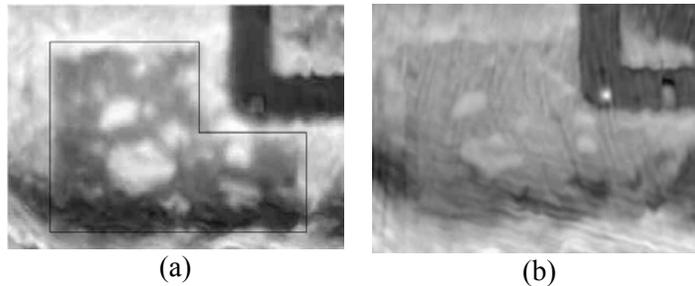
Fig. 6. SAM images of the DS interconnection in a failed DS package taken after 875 thermal cycles. (a) At the solder/power device interface and (b) at the solder/DBC copper interface.
