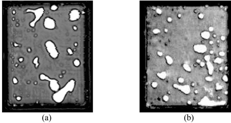
Figure 3.37. The initial void problems in the reflowed die-attaching solder layers (a) lead-tin solder and (b) lead-free solder.
