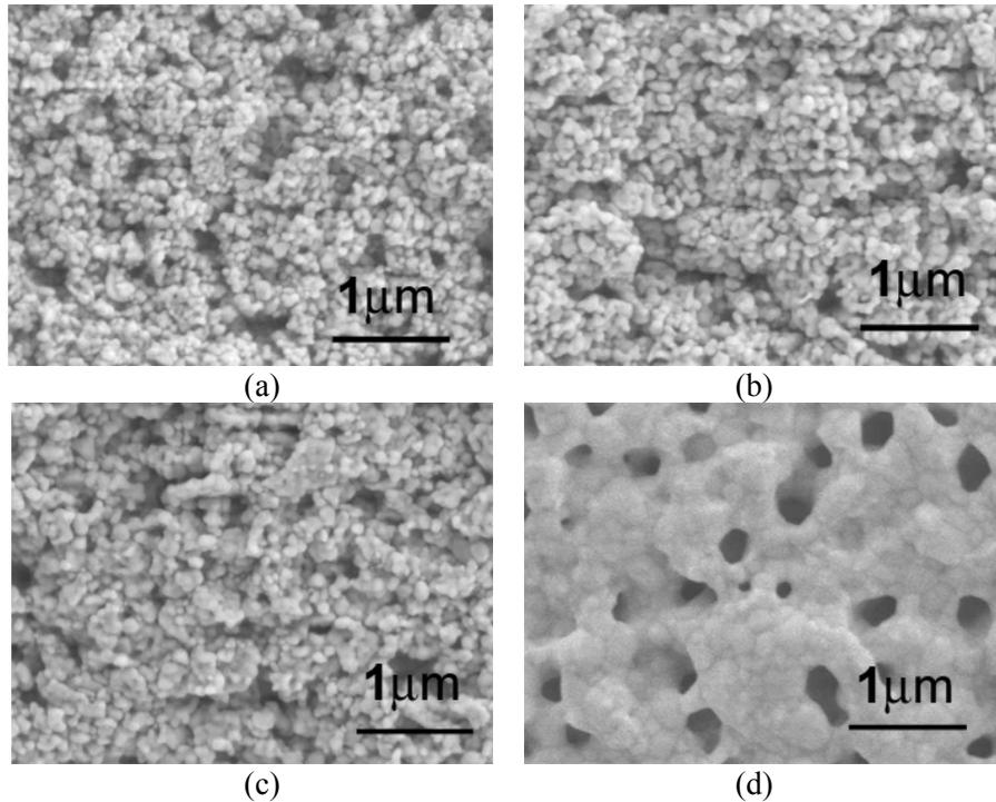
Figure 3.5. The microstructure changes of nanoscale silver heated up to 200°C (a), 225°C (b), 250°C (c) and 275°C, respectively, during the low-temperature sintering.
