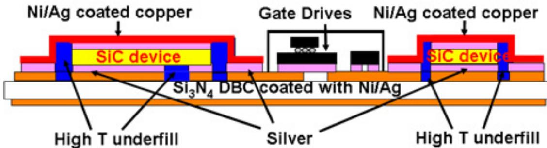
Figure 4.13. Illustration of a high-temperature integrated power electronics module bonded using low-temperature sintered silver.
