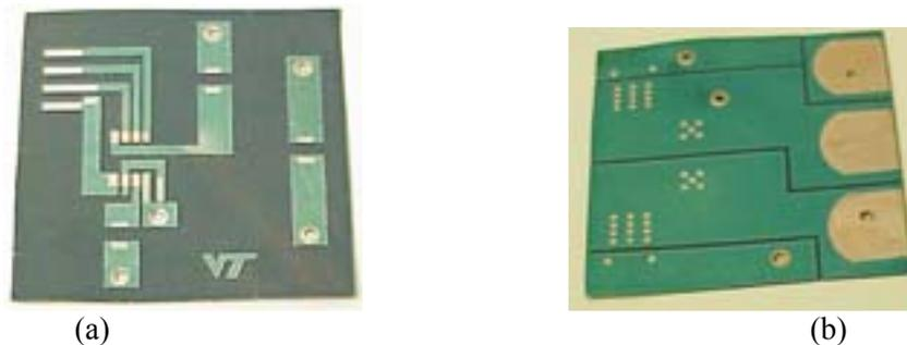
Fig. 4 A flex substrate which has a simple gate driver circuit on one side (a) and the power stage circuit on the other side (b).
