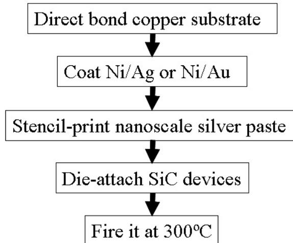
Figure 2.21. Preparation steps of the sintered silver joint samples.
