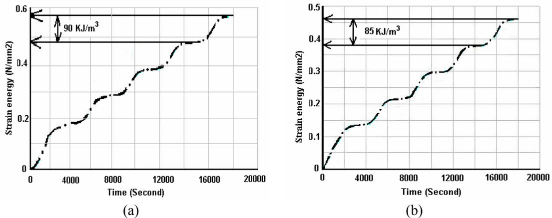
Fig. 11. The average inelastic strain energy density accumulation at the corner elements of the SB (a) and DS (b) interconnections, respectively, during the first five power cycles.
