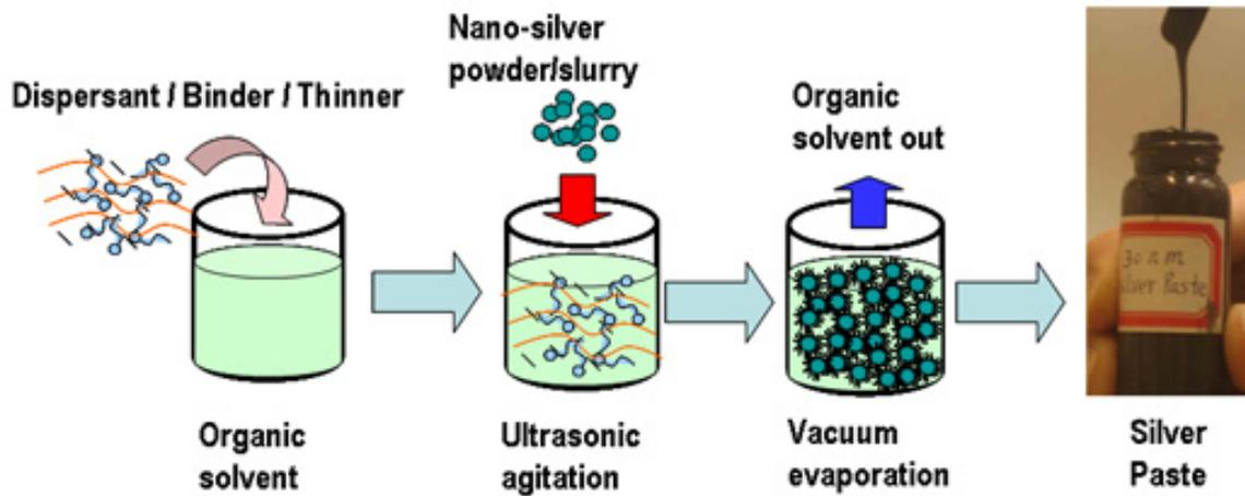
Figure 2.4. Preparation procedure of nanoscale silver pastes.
