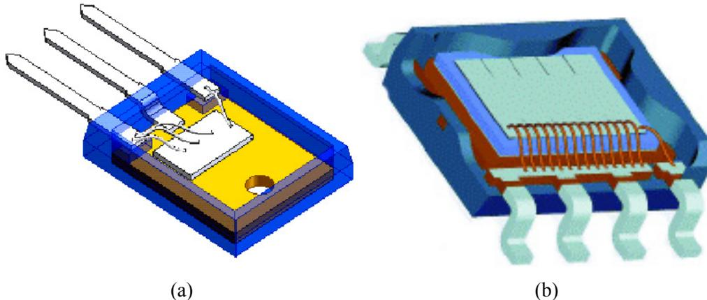
Figure 1.1. Top views of the wirebond TO-247 (a) and SO-8 (b) MOSFET packages.
