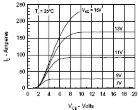
Fig.3 Collector-Emitter Voltage vs. Gate-Emitter Voltage
