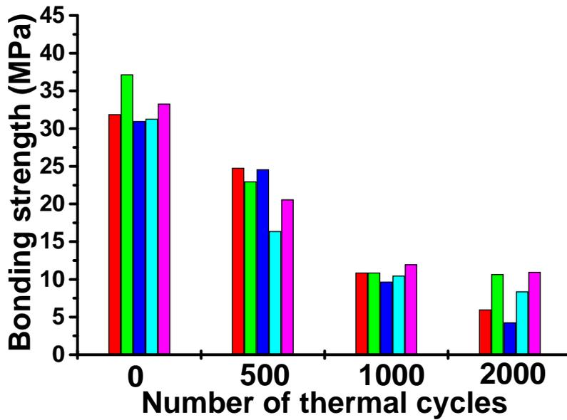
Figure 3.53. Changes of shear strength of the low-temperature sintered silver joints on nickel/silver-coated copper substrates during the temperature cycling experiment.
