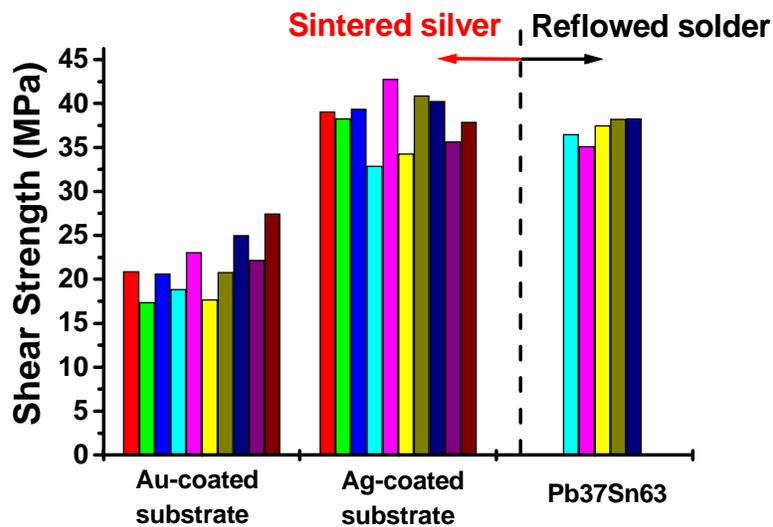
Figure 3.40. The comparison of the shear strength of the low-temperature sintered silver with that of the reflowed solder.
