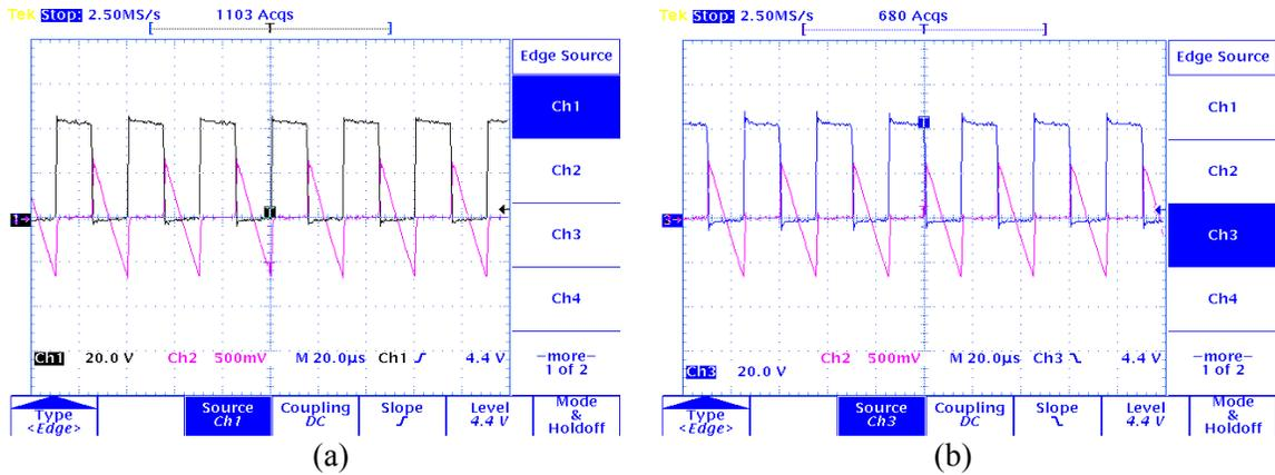
Fig. 11 Voltage and current waveforms from a continuous switching test. (a) The results from FCOF-IPEM; and (b) a commercial wire bonding power module.
