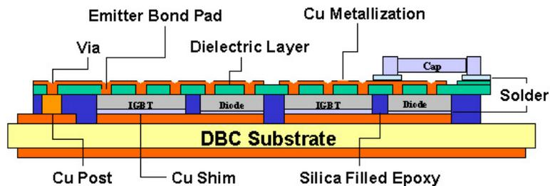
Figure 1.3. Cross-sectional schematic of power overlay module [2].
