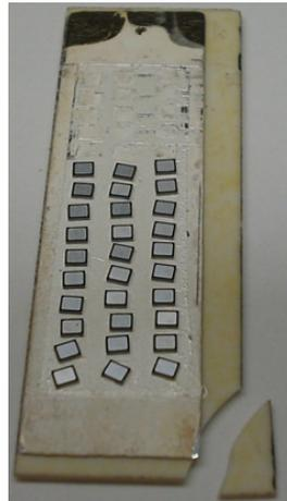
Figure 3.45. Another alumina DBC substrate broken from the alumina layer between 500 to 1000 cycles switching from 50°C to 250°C.
