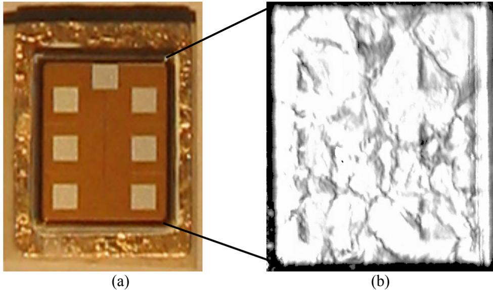
Figure 3.29. The silver sintering die-attached power IGBT with a size of  $8.91 \times 7.22$  mm<sup>2</sup> (a) and its SAM image (b).
