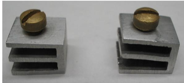
Figure 2.8. Two electrodes used for the measurement of electrical resistance.
