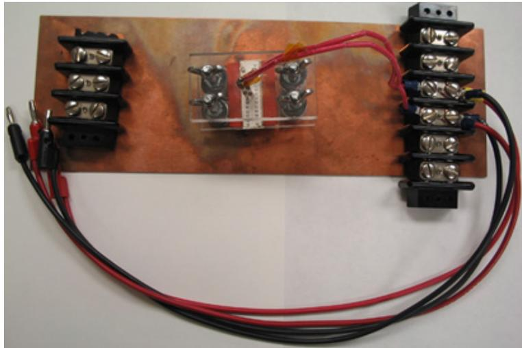
Figure 2.27. Fixture for the high-power curve tracer tests.
