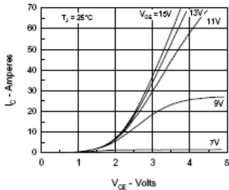
Fig.2 Output Characteristics
