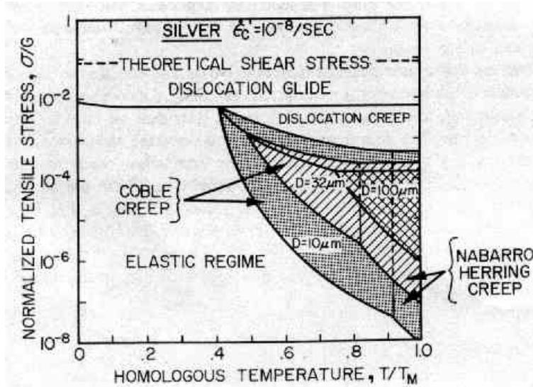
Figure 3.57. The deformation-mechanism map for pure silver, established for a critical strain rate of  $10^{-8} \text{ s}^{-1}$ ; it can be seen how the deformation-mechanism fields are affected by the grain size (reprinted from Ref. [12], p.677).
