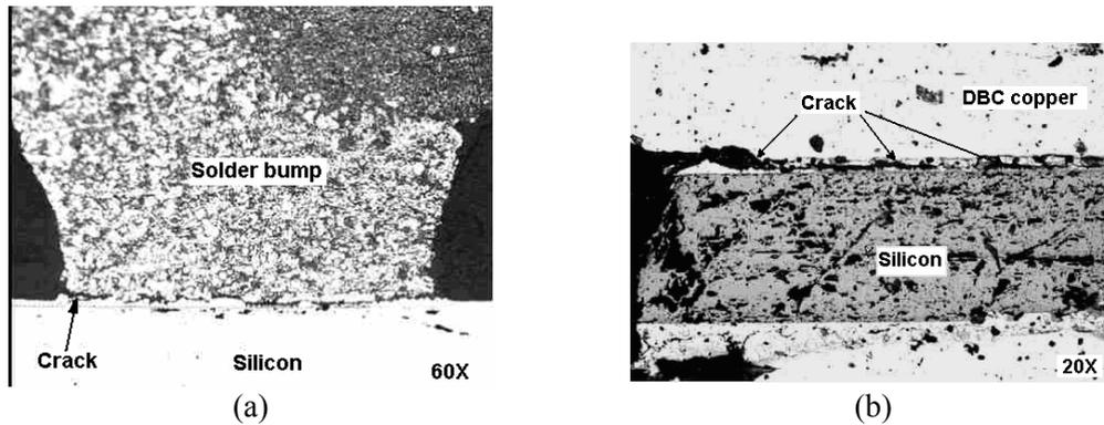
Fig. 4. Cracks at the solder-silicon interfaces in a failed SB package (a) and those in a failed DS package (b) after 875 thermal cycles.
