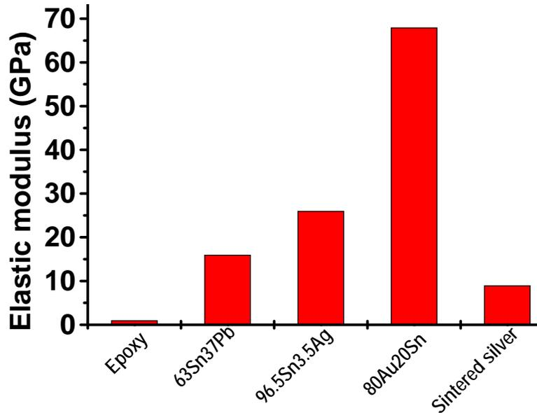
Figure 3.22. Comparison of elastic modulus values of common-used interconnecting materials with that of the sintered silver.
