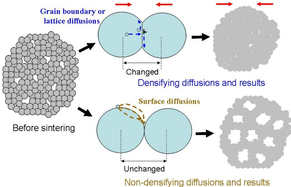
Figure 1.22. Illustration of densifying and non-densifying diffusions and their sintering results.
