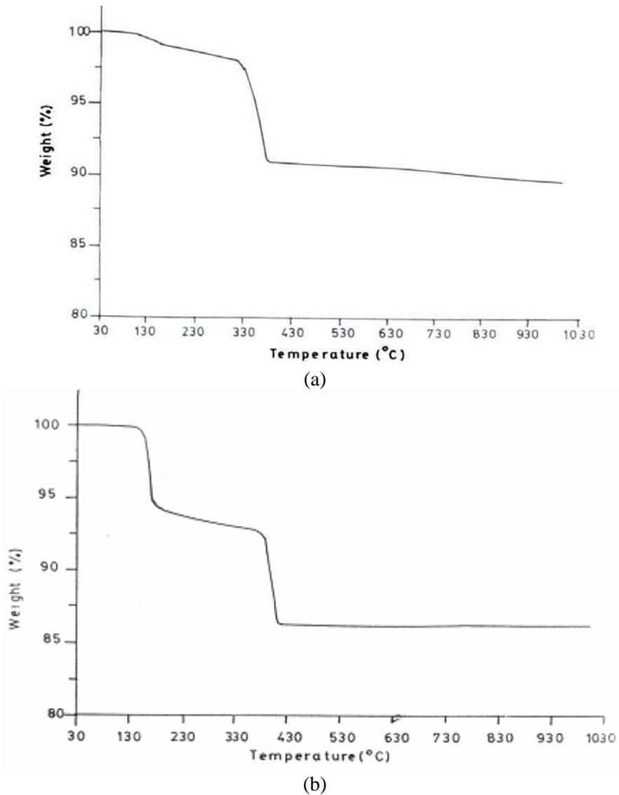
Figure 5.1. TGA curves of microscale Ag<sub>2</sub>O (a) and AgO (b).
