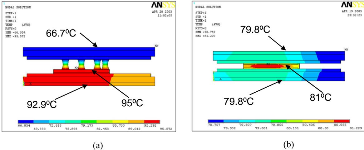
Fig. 7. Thermal FEA temperature distribution results of (a) the SB and (b) the DS packages under the same operation and double-sided cooling conditions.
