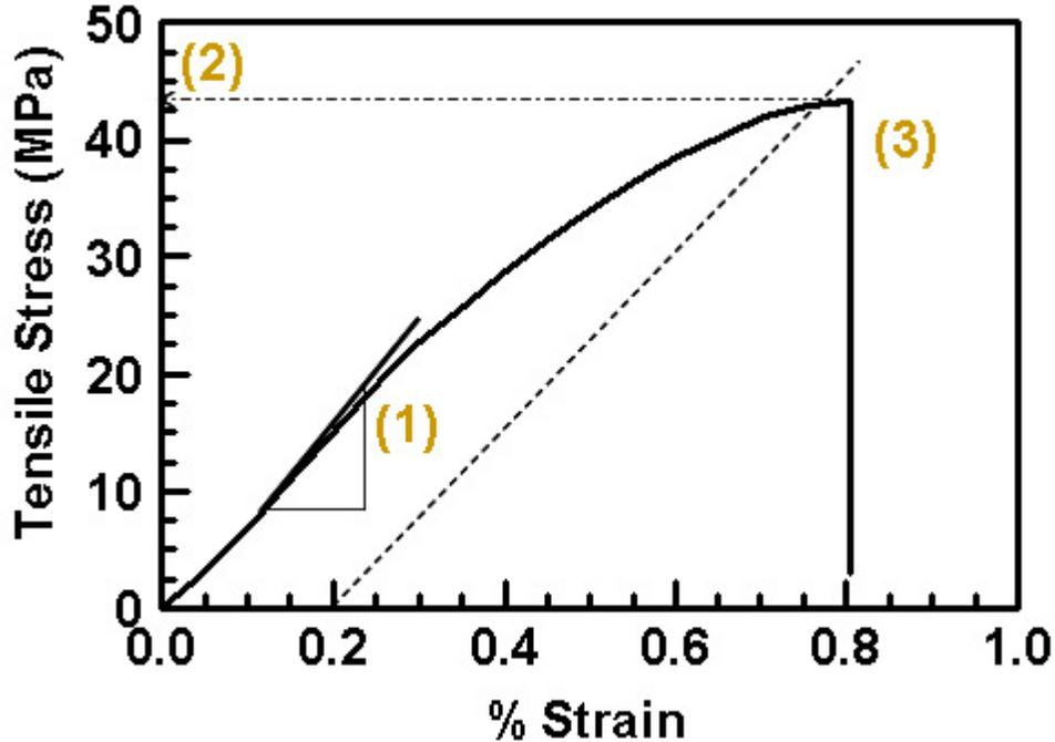
Figure 3.21. A typical stress-strain curve of the sintered silver in the tensile test.
