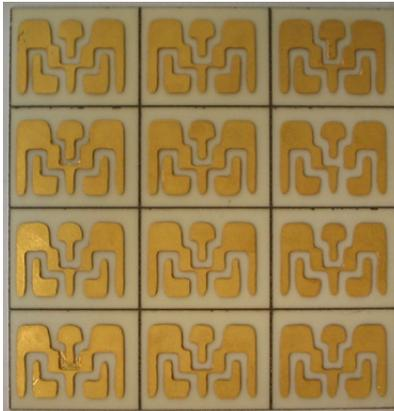
Figure A.2. The etched aluminum oxide DBC substrate for packaging white LEDs.
