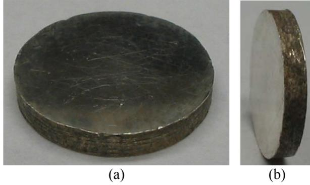
Figure 2.10. The disc-shaped silver specimens prepared by molding and low-temperature sintering.
