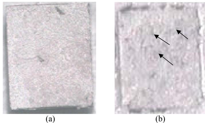
Figure 3.41. Optical microscopy pictures of one of the sheared-off Infineon SiC device (a) and the corresponding die-attach cavity on the gold-coated DBC substrate (b). The arrows in (b) indicate the debonding areas from the gold-silver interface.
