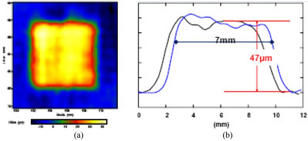
Figure 3.6. Topological image (a) and its two topological profiles (b) of the printed nanoscale silver paste before sintering.
