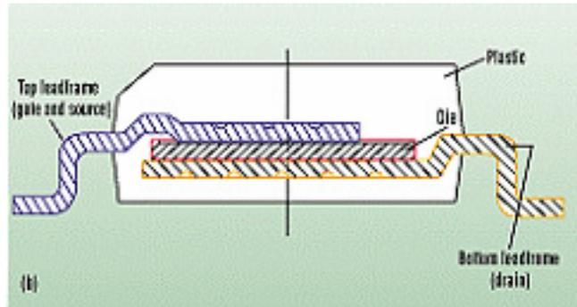
Figure 1.7. Cross-sectional schematic of a PowerConnect chip-level power package [5].
