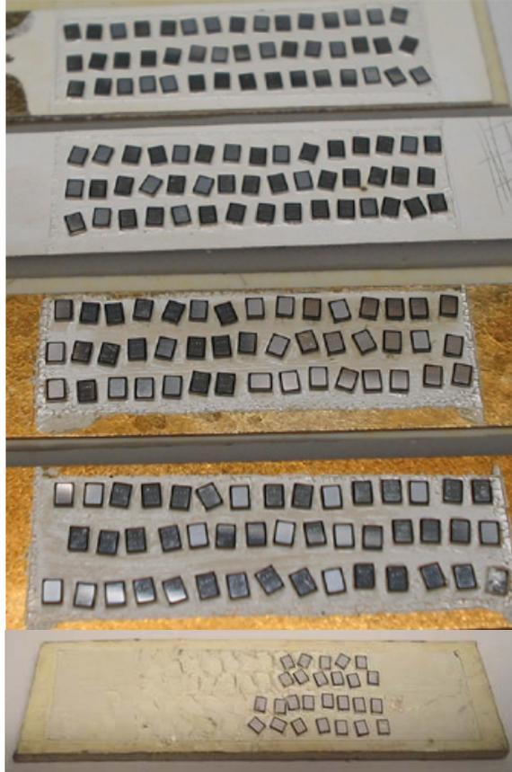
Figure 2.32. The die-attached Infineon SiC devices used for the 50-250°C thermal cycling experiment. From top to bottom: Ag-coated  $\text{Al}_2\text{O}_3$  DBC, Ag-coated AlN DBC, Au-coated  $\text{Al}_2\text{O}_3$  DBC, Ag-coated AlN DBC, and Ag-coated copper substrates.
