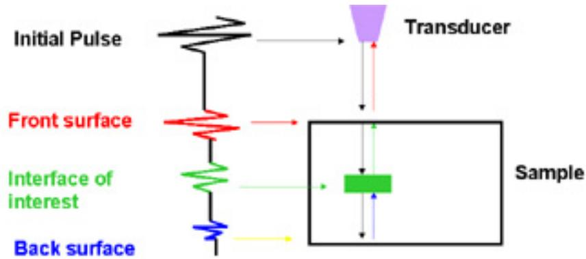
Figure 2.28. The pulse-echo mode illustration in scanning acoustic microscopy.
