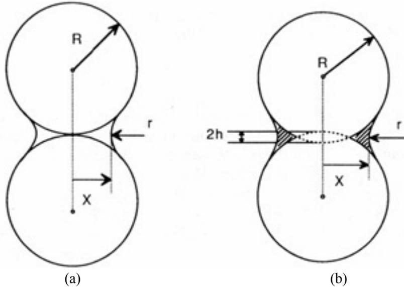
Figure 1.20. Two-particle geometric model for the initial stage of sintering [32].
