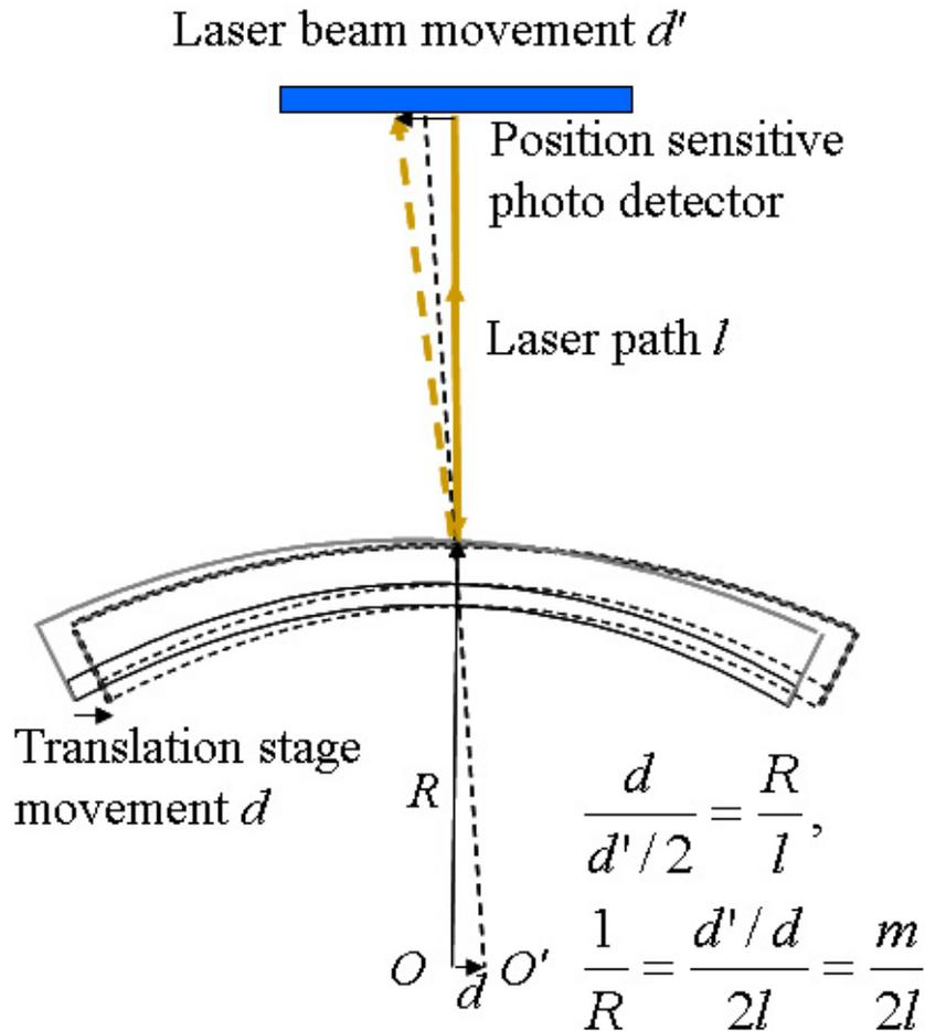
Figure 2.19. The illustration of the translate relationships in the optical setup during the curvature measurement.
