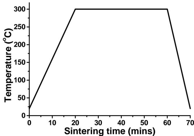
Figure 3.33. The sintering profile for achieving enhanced sintering and high bonding strength for the silver joints with size 4×4 mm<sup>2</sup> or below.
