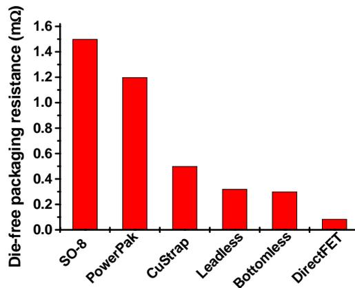
Figure 1.19. Reduction of die-free package resistance along IR's chip-level discrete power package developing roadmap.
