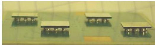
Fig. 6 The power devices and flex substrate assembly after flip-chip bonding.
