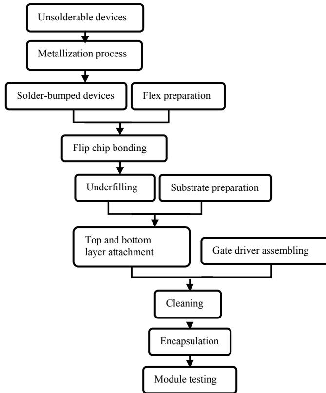
Fig. 2 The FCOF-IPEM fabrication flowchart.
