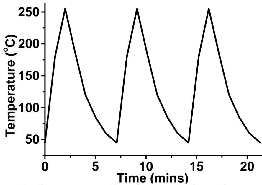
Figure 2.34. The temperature profile obtained using the Sikama belt reflow oven.
