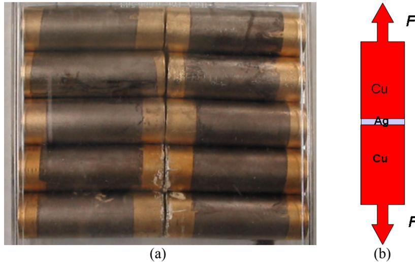
Figure 2.14. Nickel/gold plated copper rods for the preparation of sintered silver joints (a) and their debonding illustration.
