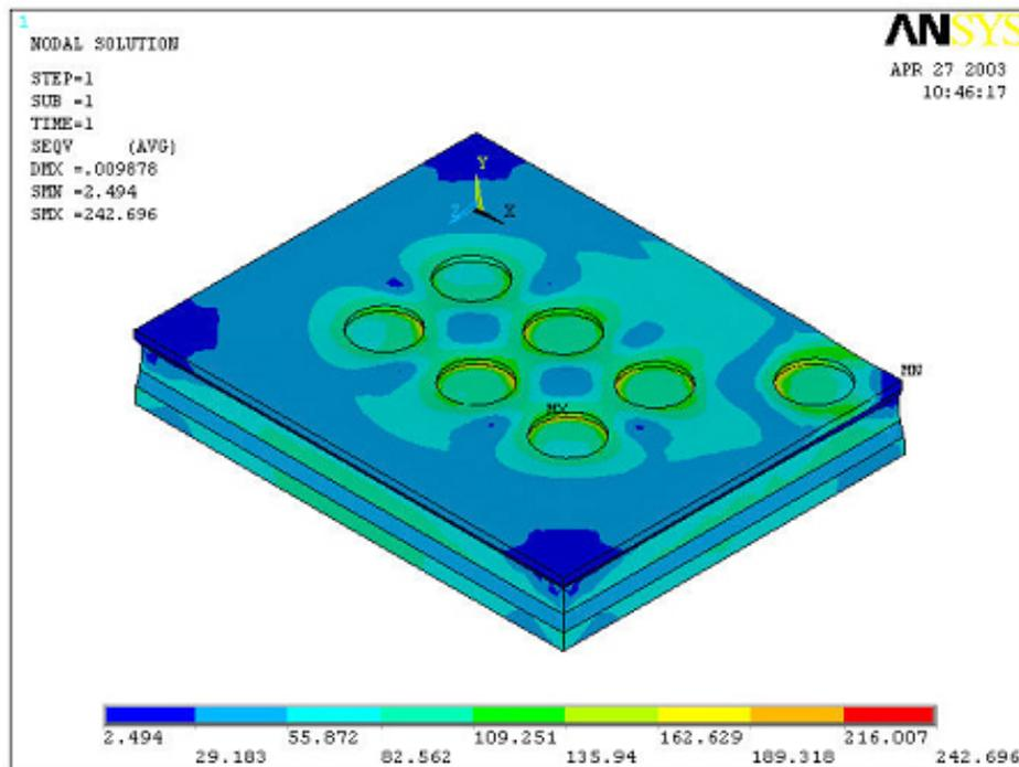
Figure 1.25. Thermal stress distribution in the local position when the MOSFET operating at 94°C in an embedded power module [61].
