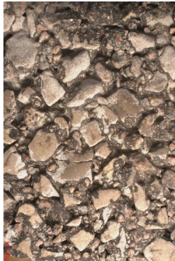
Figure 5 - Photograph of mix 14 specimen polished in the W-S machine
