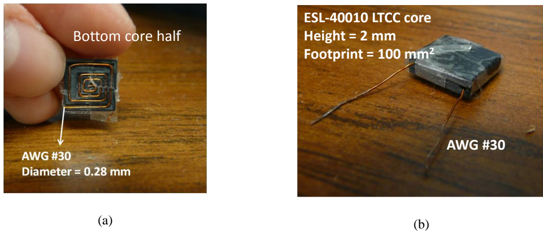
Figure 4.17. Fabrication of constant-flux inductor with copper wire as the winding and LTCC ferrite as the core: (a) A bottom core half with AWG#30 copper wire wrapped spirally inside; (b) assembled inductor prototype with two inductor halves connected at the center by solder. The inductance is 2.6\text{ }\mu\text{H} (1.9% error against simulation), and the resistance is 62\text{ m}\Omega (8.9% error against simulation).
