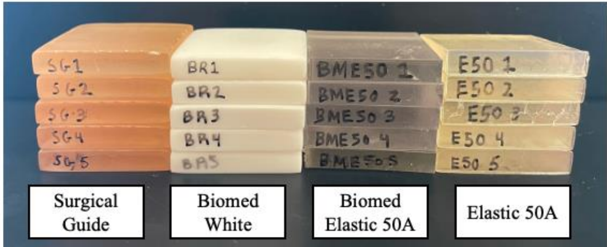
Figure 0-1. All 3D-printed material candidates tested for their material properties.
