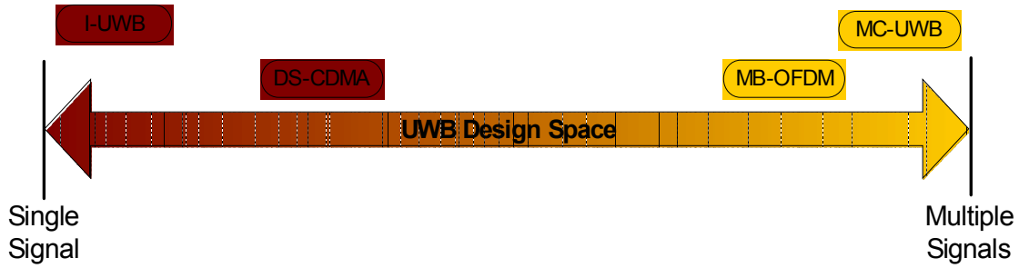
Figure 2.7: Solution Space for UWB Signaling
