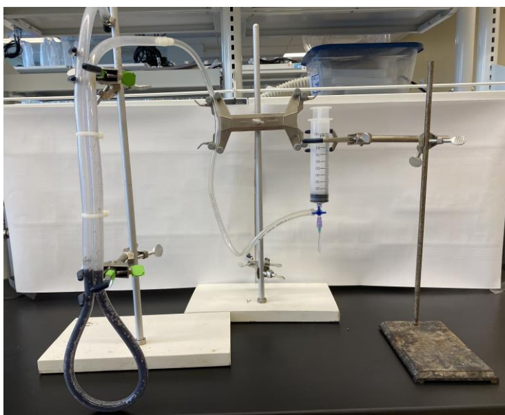
Figure 6. Biogas collection set up to measure biogas volume
