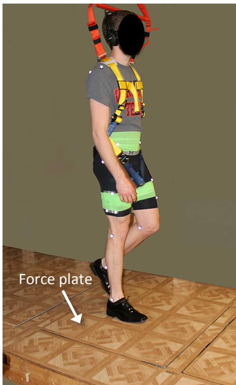
Figure 2. The experimental setup, showing a modified Helen-Hayes marker set, PVC-soled shoes, headphones, force plate, and safety harness. Photo by author, 2014.
