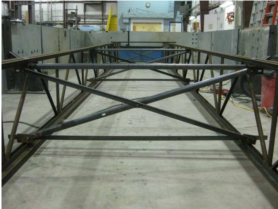
Figure 2.7 Bridging lines used during laboratory testing
