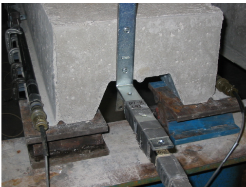
(c) Potentiometer at slab end
