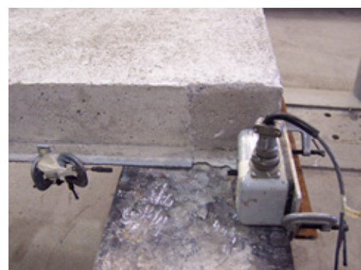
(f) Wire pot at slab end
