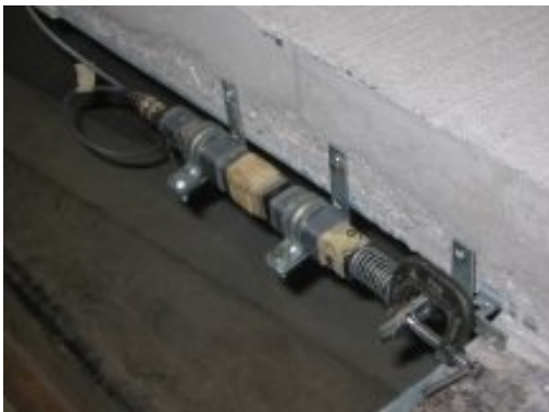
(e) Potentiometer at interior end
