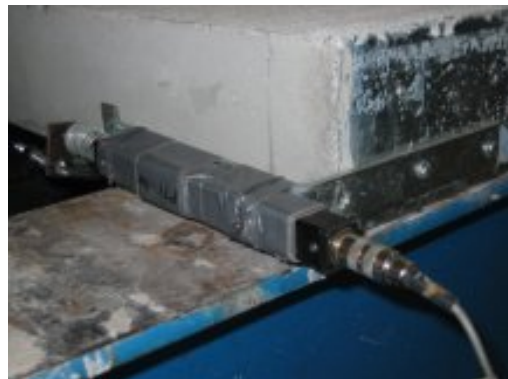
(f) Potentiometer at exterior end
