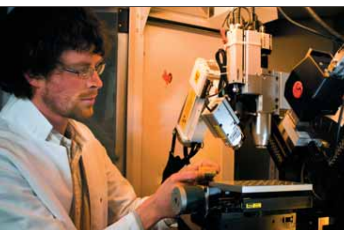
Carter Fox, a Ph.D. candidate in the Macromolecular Science and Engineering Program, prepares a sample of drug in polymer for x-ray analysis of crystallinity.
