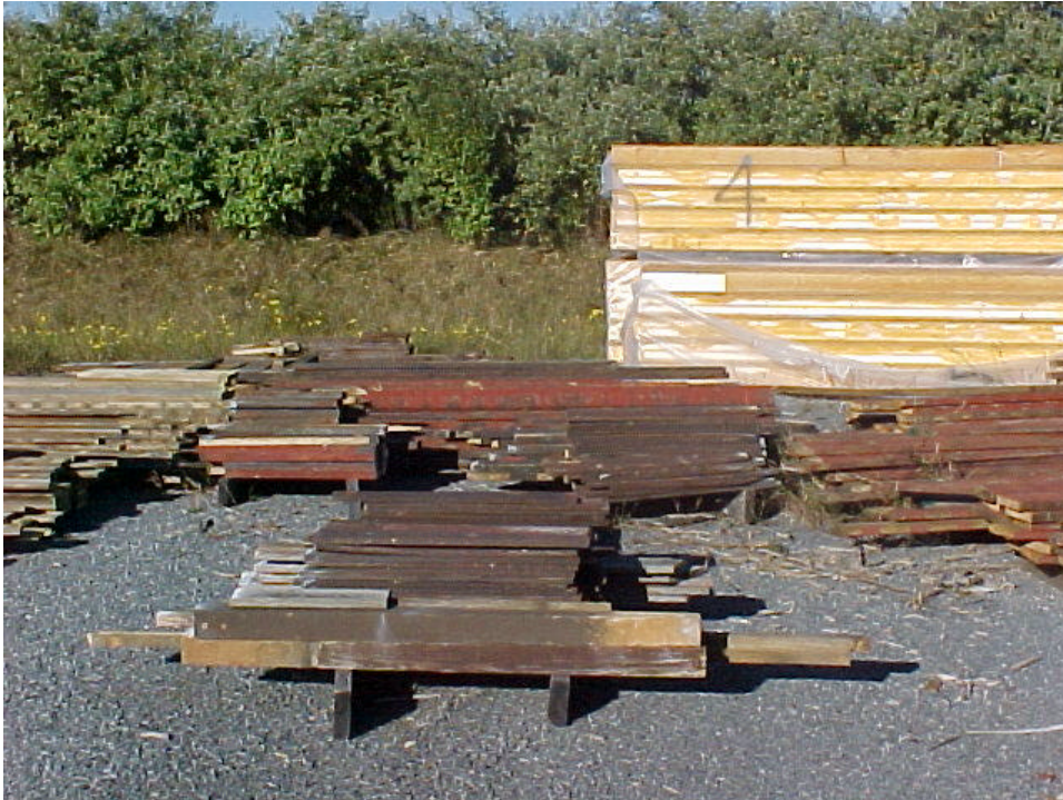
Figure A- 5. Recovered CCA treated wood from Deck #5.
