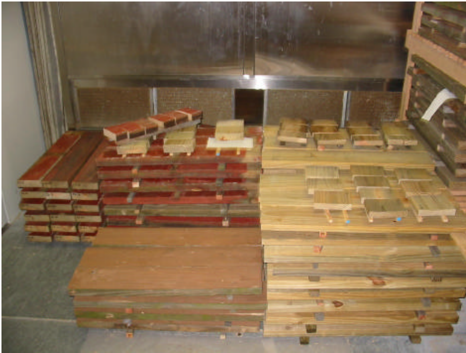
Figure A- 7. Mechanical test samples in conditioning chamber.
