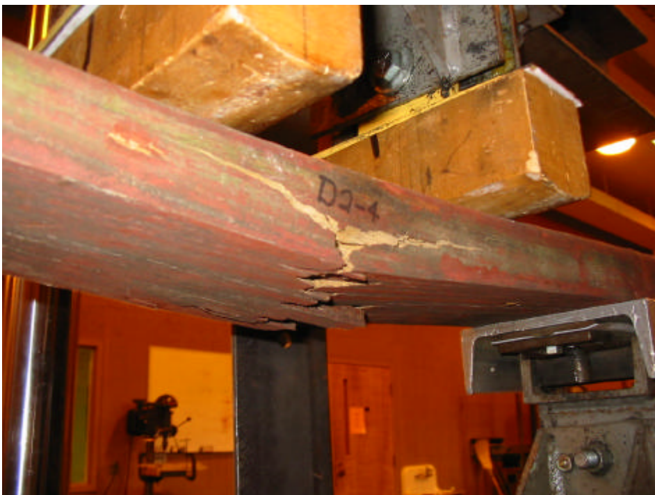
Figure A- 10. Typical failure of test samples under load.
