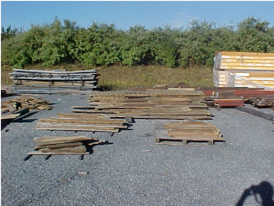
Figure A- 1. Recovered CCA treated wood from Deck #1.
