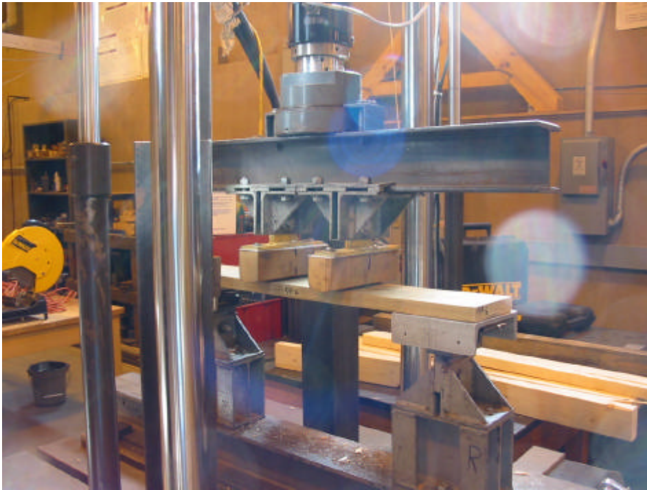
Figure A- 9. Loading of samples in MTS machine.
