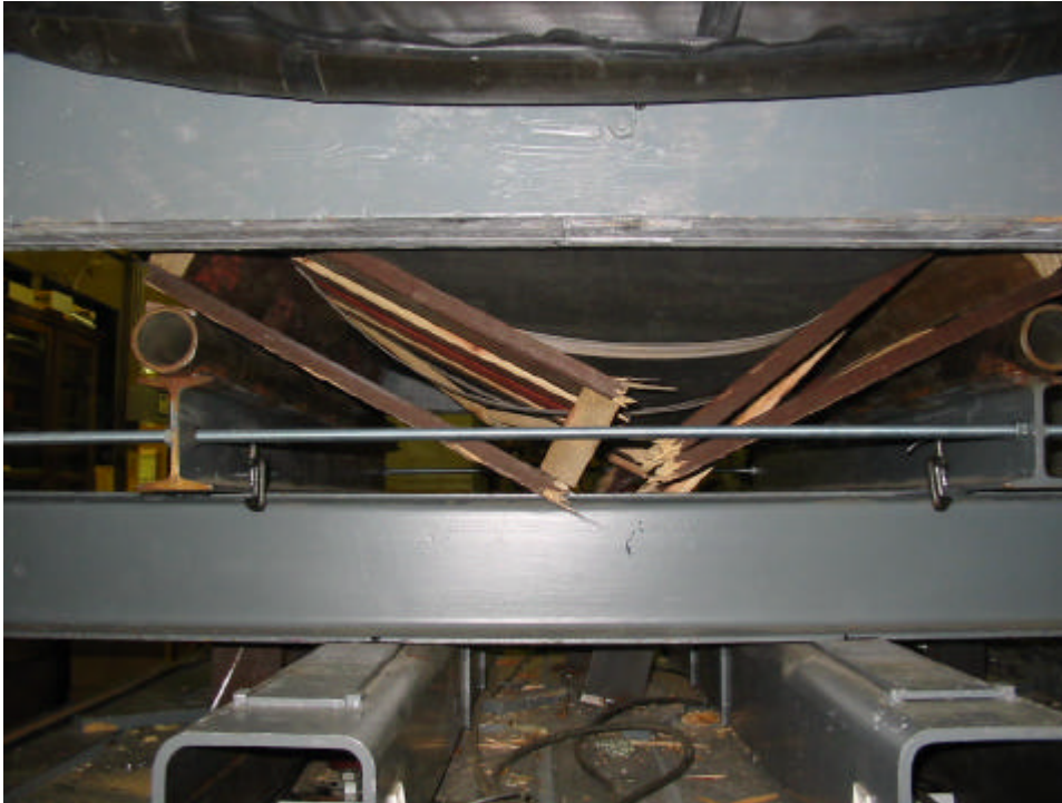
Figure 4- 14. Stringer pallet racked across the width, after failure.
