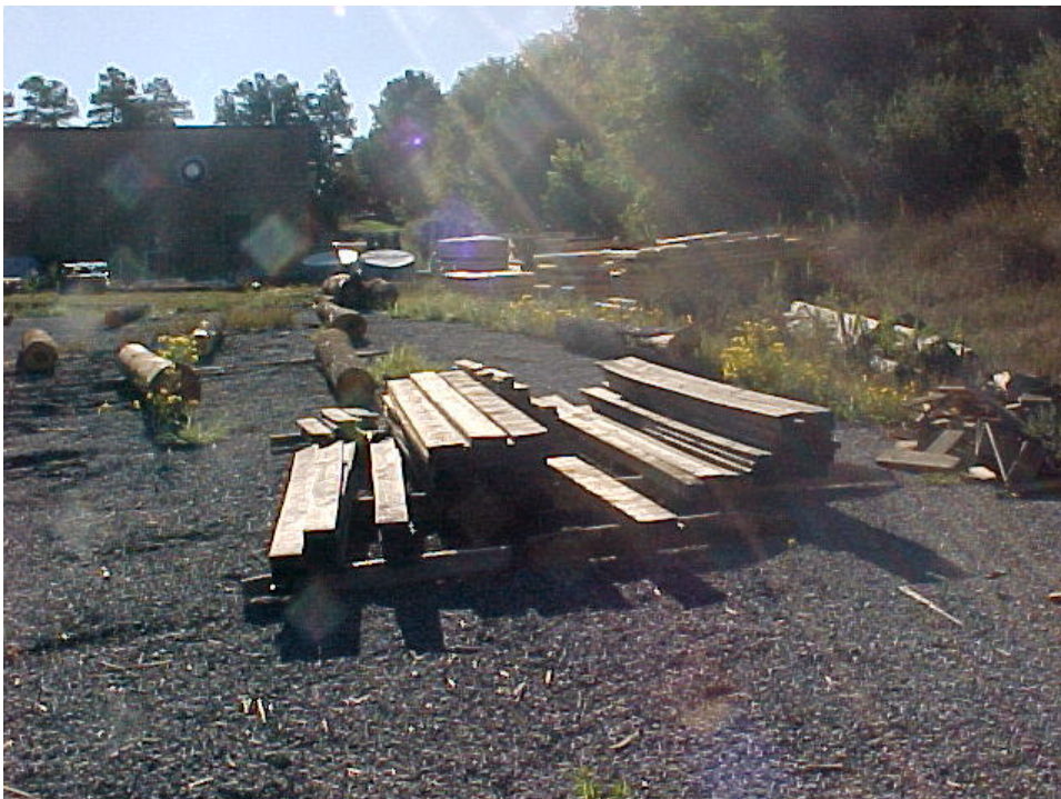
Figure A- 4. Recovered CCA treated wood from Deck #4.
