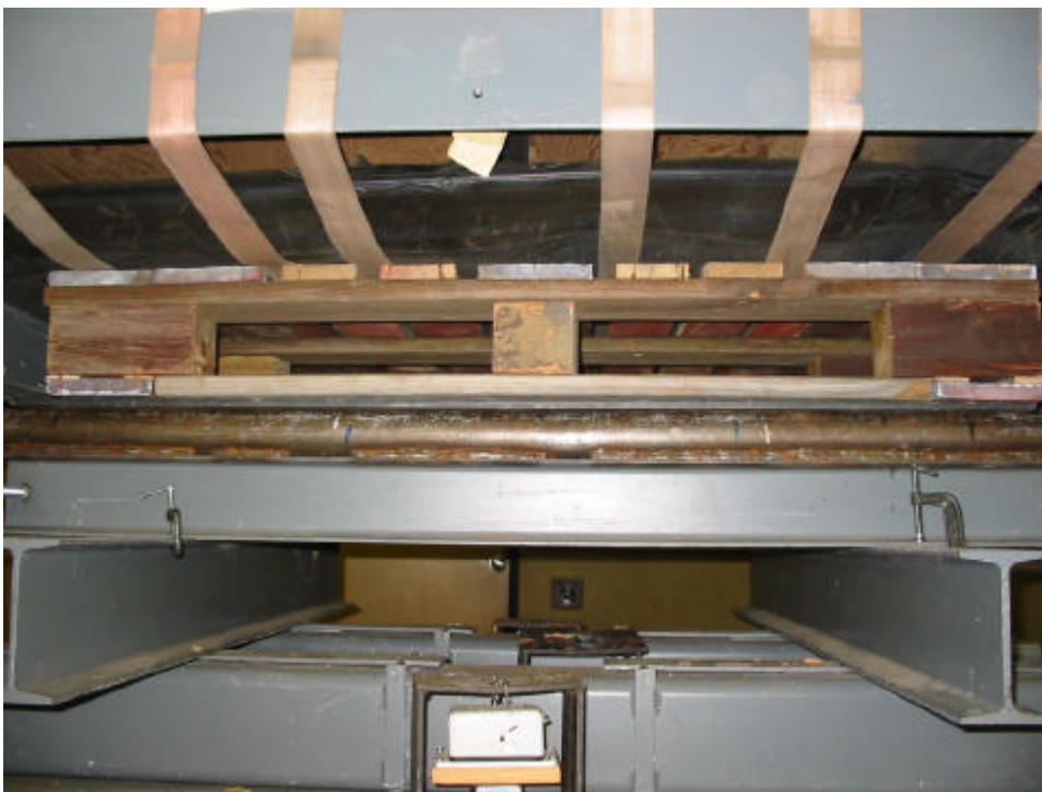
Figure 4- 15. Block pallet racked across the length, before load was applied.
