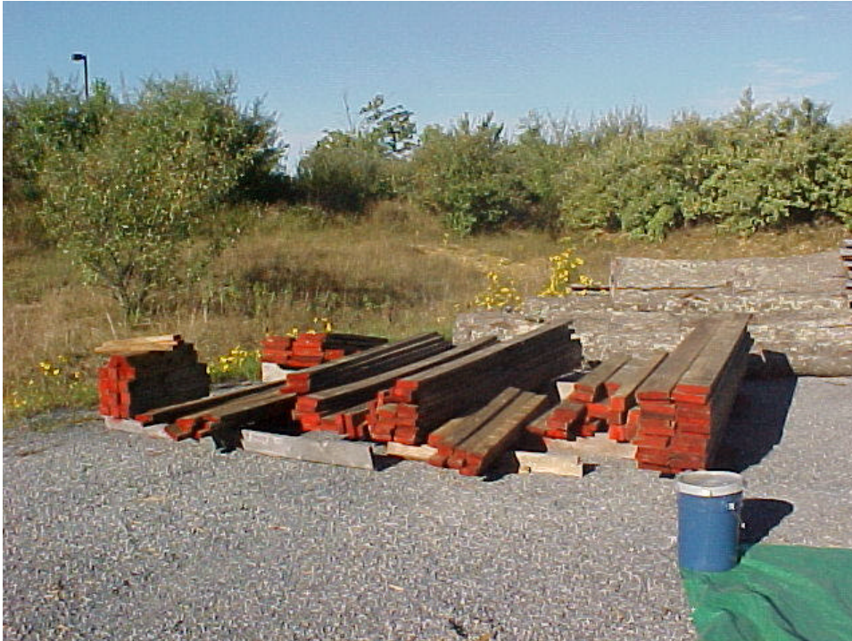
Figure A- 3. Recovered CCA treated wood from Deck #3.
