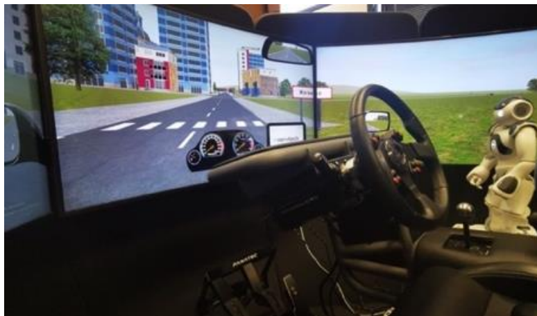
Figure 3.2-1 Experimental setup with the NervTech driving simulator and Nao.
