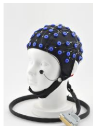
Fig 7a. Traditional Electrode Cap
