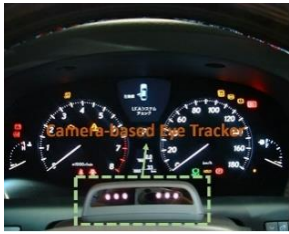
Fig 1a. Sample Driver Monitoring System (Lexus)
