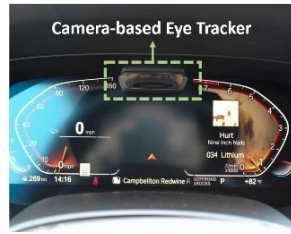
Fig 1b. Sample Eye Tracking Sensor (BMW)
