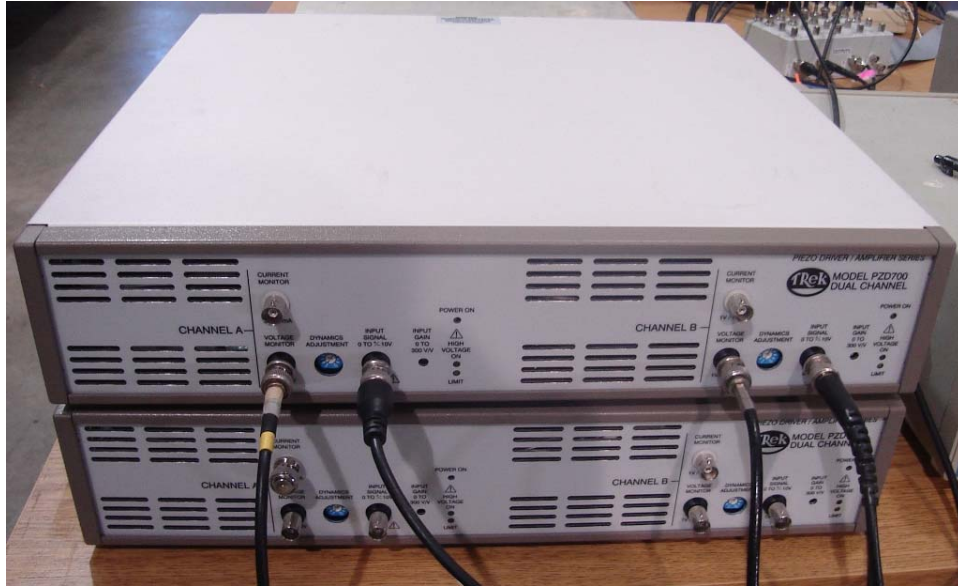
Photo by Mohammad Rastgaar, January 2008 Figure 7.5. High voltage PZD 700 piezo-drivers from Trek
