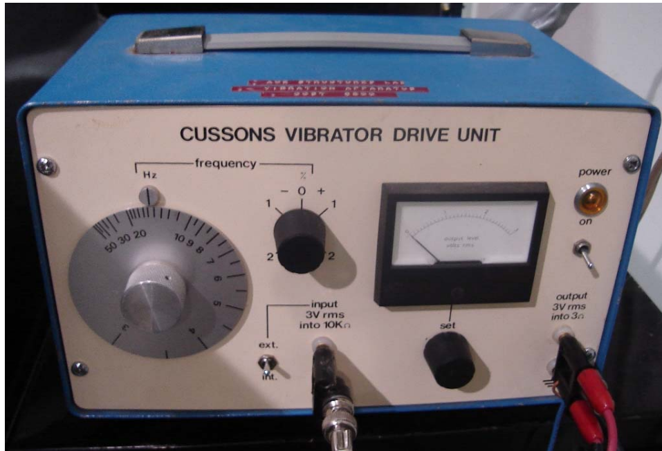
Photo by Mohammad Rastgaar, January 2008 Figure 7.3. Amplifier for the Electromagnetic actuator
