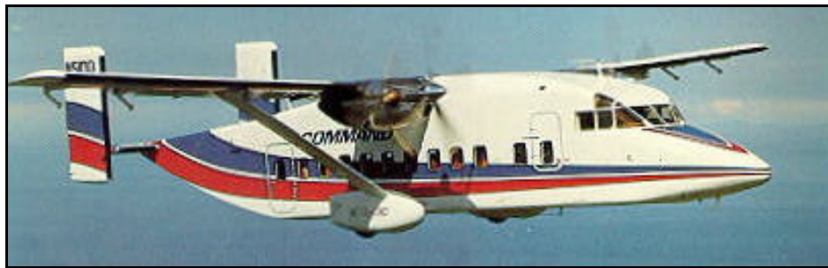
Figure 4-37: Landing gear fairing on a Shorts 330 [49]
