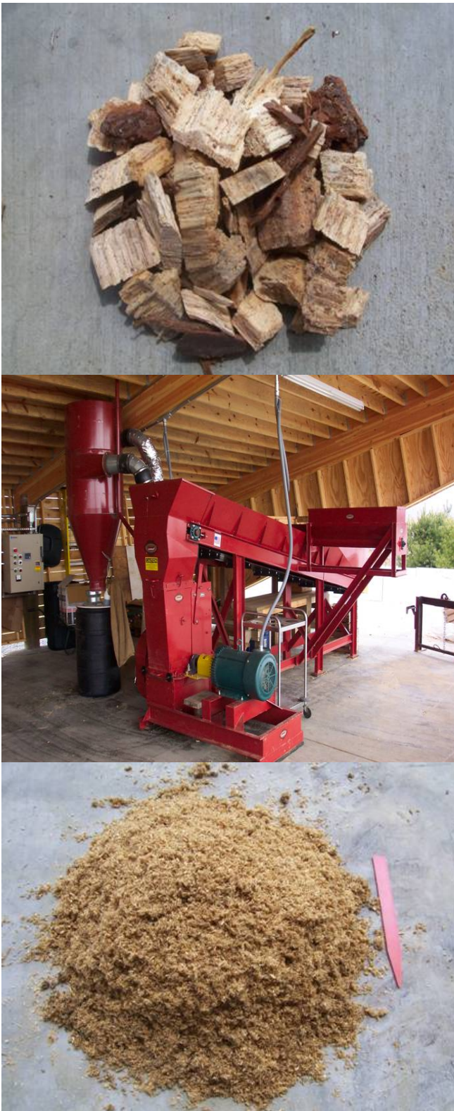
Figure 1.13. Loblolly pine wood chips (top) are ground in a hammer-mill (middle) to reduce the size of the wood to a desired particle size (bottom) to produce pine tree substrate ready for potting and planting.
