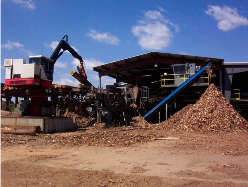
Figure 1.1. Harvested loblolly pine trees being debarked at a processing facility located in Warsaw, VA. The debarked logs are used for pulpwood or saw timber and the removed bark is a by-product which can be used as a container substrate.
