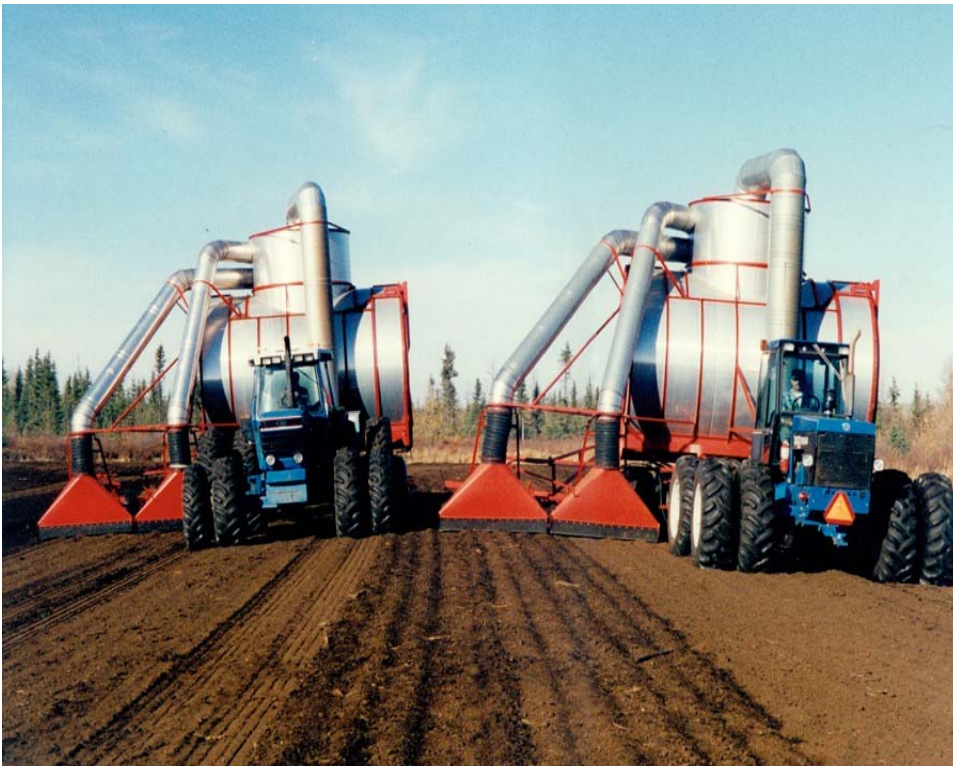
Figure 1.6. Once peat bogs are drained and cleared of vegetation, peat harvesting requires large equipment which extracts the peat by several methods including vacuuming.
