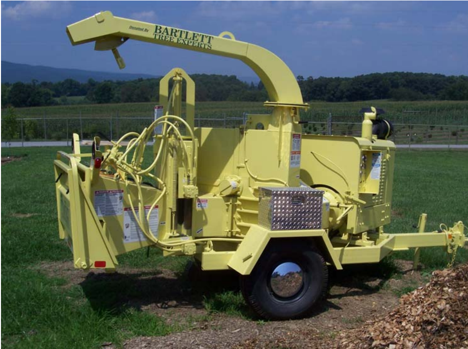
Figure 1.11. Industrial wood chipper used to chip pine logs into small wood chips that are then small enough to be ground in a hammer-mill for substrate production.
