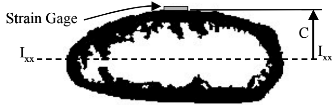
Figure 4: Geometric data gathered from rib specimen cross section for stress calculation.
