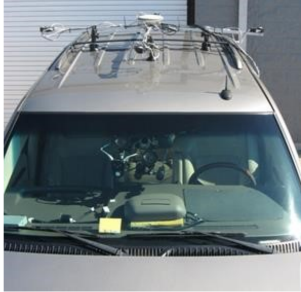
Figure 2. Photo. RLMMS system showing the luminance cameras and the Minolta illuminance head that measures the vertical illuminance.
