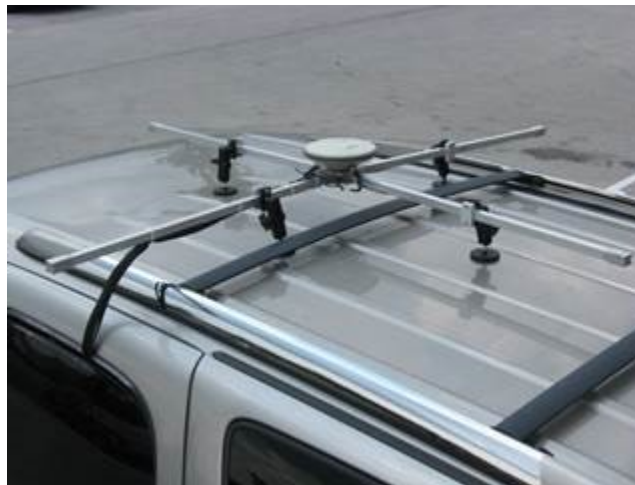
Figure 1. Photo. RLMMS system’s “Spider” apparatus with four Minolta illuminance heads and NovaTel GPS device in the center.
