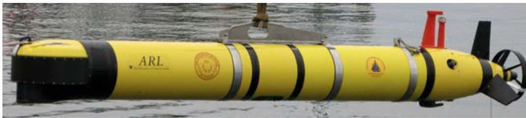
Fig. 5.9: ATLAS sonar mounted on a REMUS 600 [26] < Loeffler, C., 15 Sept. 2011, “Sonar and AUV Technology,” National Oceanic and Atmospheric Administration, Web. 5 Nov. 2014.> (public domain, 2015)
