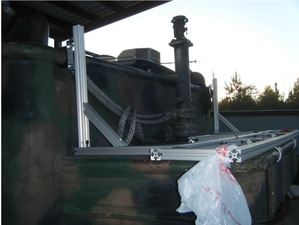
Fig. 4.5: Stern cradle for FY2013 field trials
