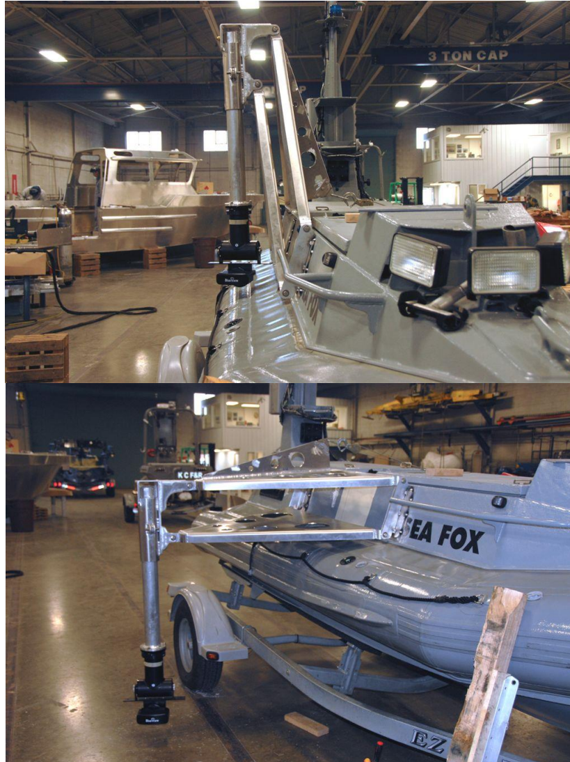
Fig. 2.8: Naval Postgraduate School's Sea Fox USV with 4-bar linkage sonar mount (Image courtesy of Sean Kragelund, 2015)
