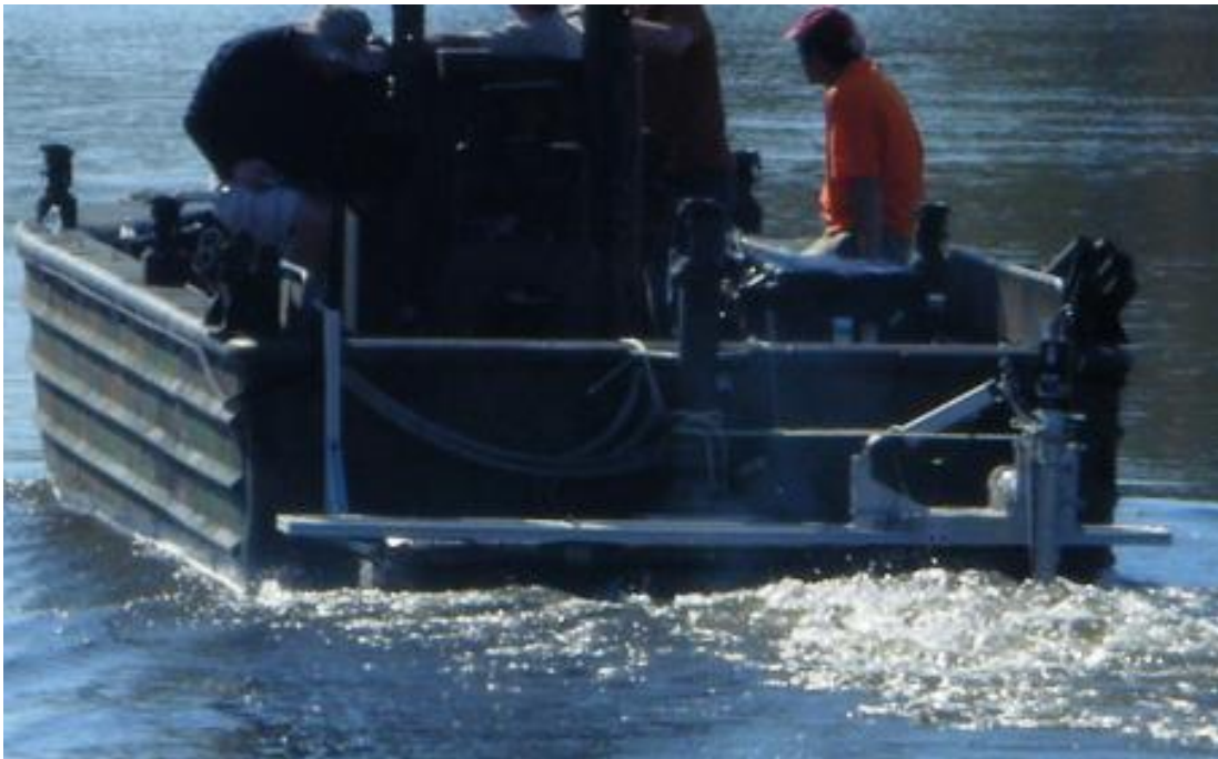
Fig. 4.7: Stern sonar mount in operation, FY2013
