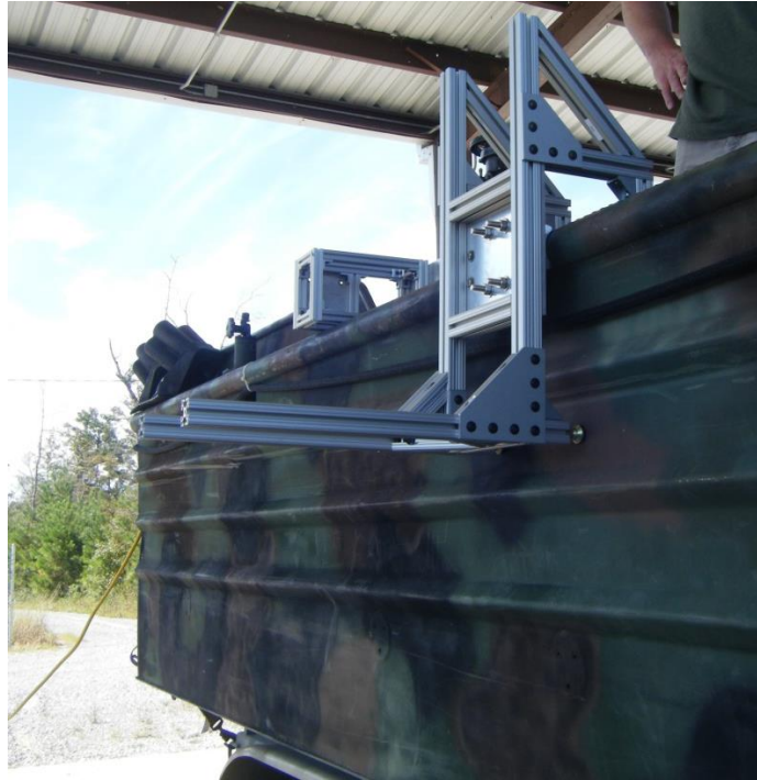
Fig. 4.3: Sonar mount cradle for FY2012 field trials
