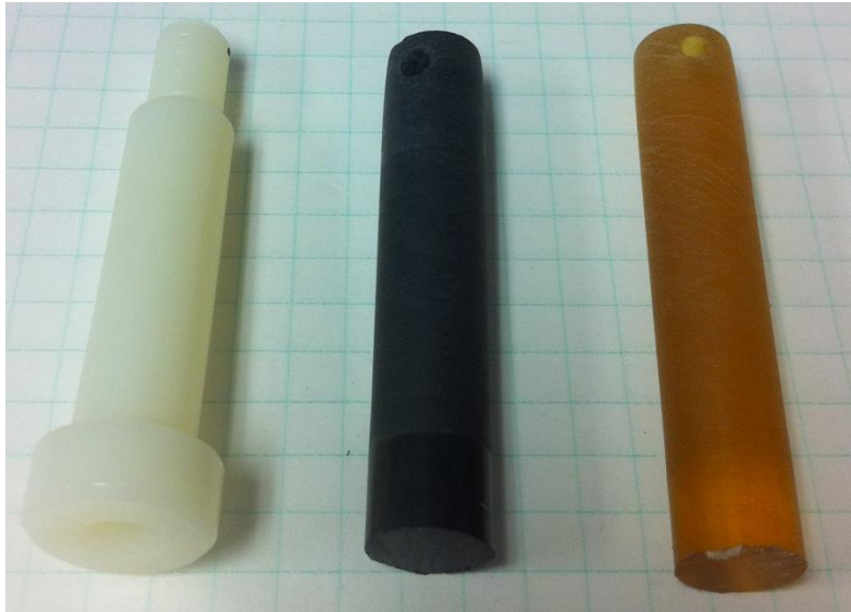
Fig. 3.10: Three shear pins purchased. L to R: Nylon 6/6 shoulder bolt, 20% glass-filled polycarbonate, ULTEM ® .
