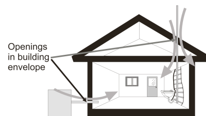
Figure 1. Bulk moisture transport
