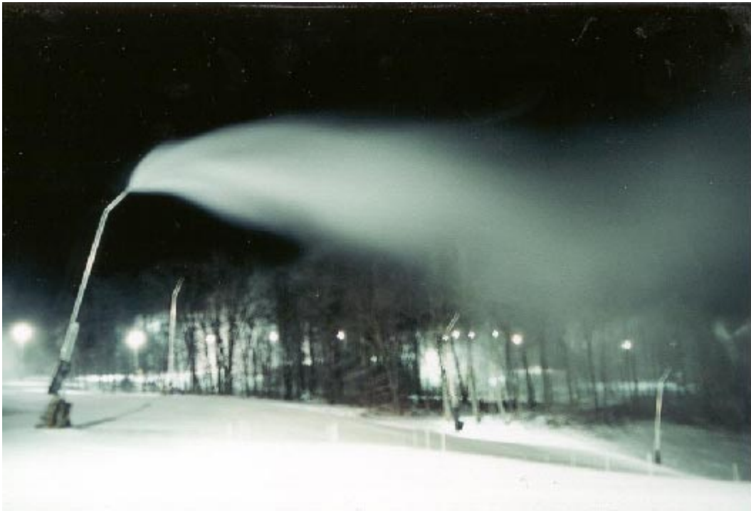
Figure 6.4 Snowmaking In High Winds With the Tower at a Steep Vertical Angle
