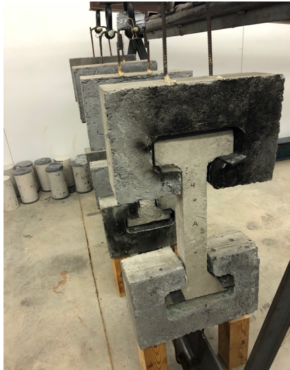
Figure 3-3: Tensile creep specimen loaded
