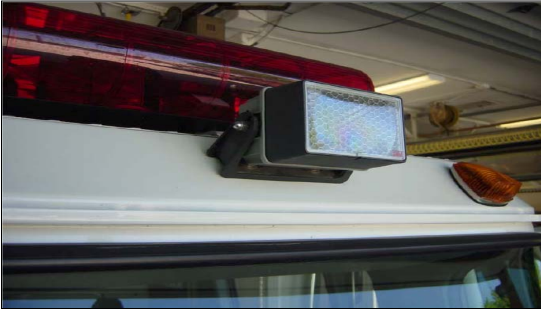
Figure 8. Photographs to show 3M Opticom Emitters
