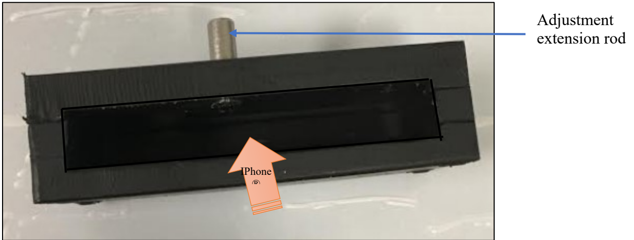
Figure 4 iPhone® 6S adaptor- front view (constructed by Steve Harris with design by Sathie Thayagan. iPhone®6S is owned by Apple Inc.)
