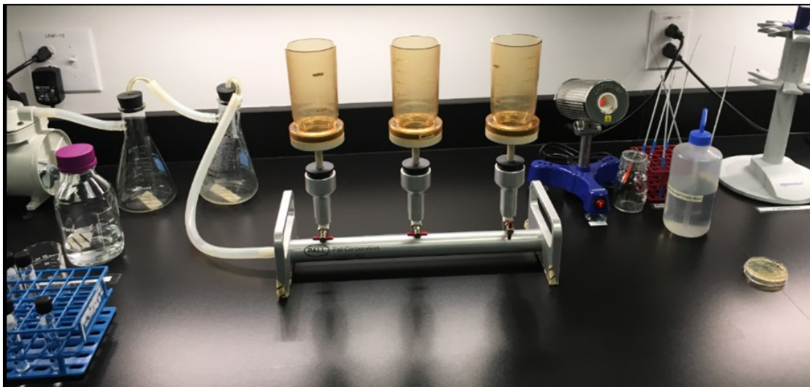
Figure 9 Typical Membrane filtration setup
