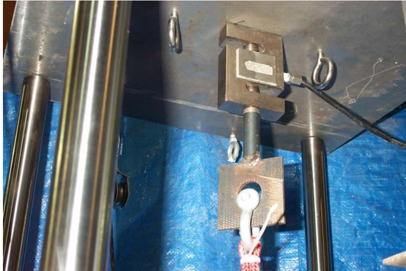
Figure 3.3 Ten-kip Load Cell with Attached Rope
