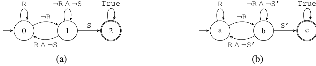
Figure 5.6: Example: (a) safety specification \varphi^s(R, S) and (b) correctness monitor \mathcal{Q}(R, S') .
