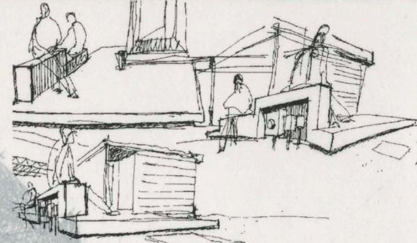
From the prefabricated concrete slab, the unit can be brought into a leveled position where the single point foundation adapts to the topography of different sites.
