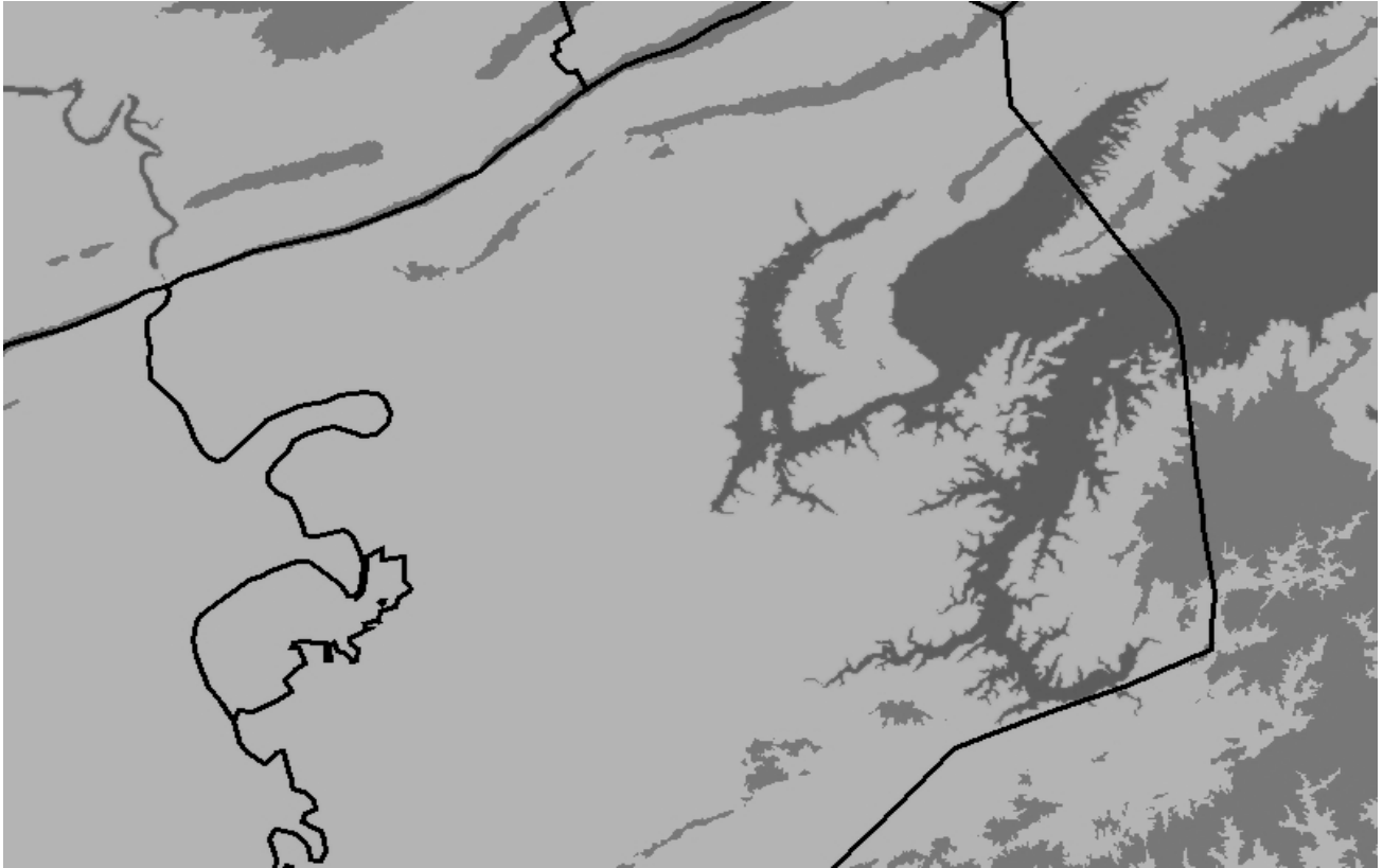
FIGURE 2.4. Geographic Information System image showing elevation levels for Montgomery County, Virginia, for example (EROS Data Center 1999). Dark gray represents elevation greater than 800 m, medium gray less than 500 m, and light gray between 500 m and 800 m.
