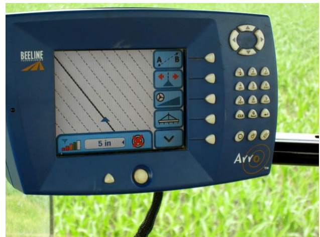
Figure 1: A tractor's GPS readout and controls " GPS Steers The Tractor " by cogdogblog is marked with CC0 1.0 .
