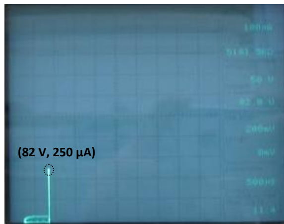
Fig. 4.22. Three series-connected MOSFETs (testing between “a” and “d”) with 82 V breakdown voltage Sample 2.
