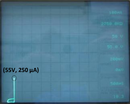
Fig. 4.20. Two series-connected MOSFETs (testing between “a” and “c”) of Sample 1 with 55 V breakdown voltage.
