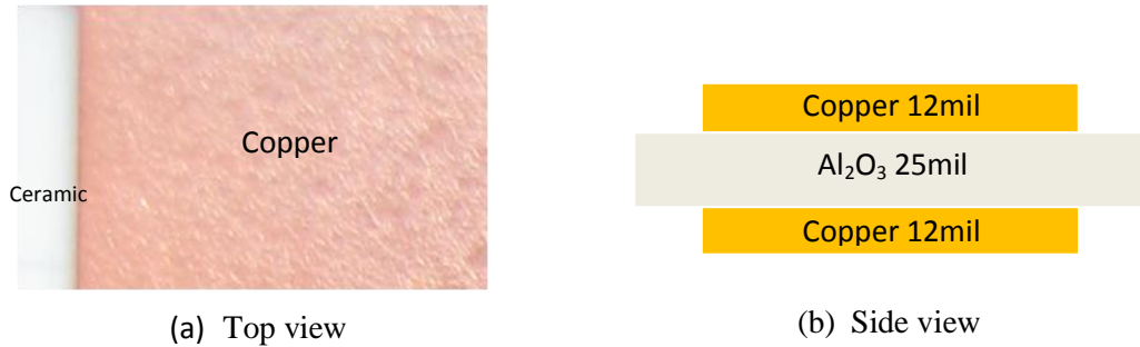
Fig. 4.2. Top view and side view of the DBC substrate.
