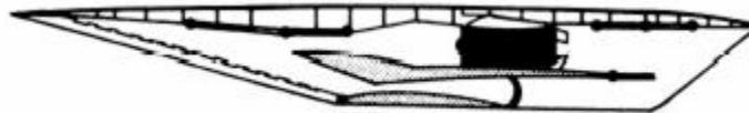
Figure 1.6. A dual mode turboramjet concept. A common diffuser accommodates both the turbojet (top) for low speed flight and the ramjet (bottom) for high speed flight [3].
