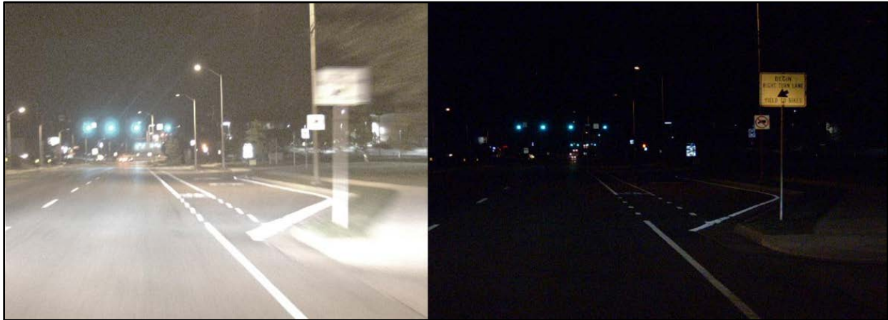
Figure 7. Photos. Images from color camera in automatic control mode (left) and using the daylight calibration file (right).
