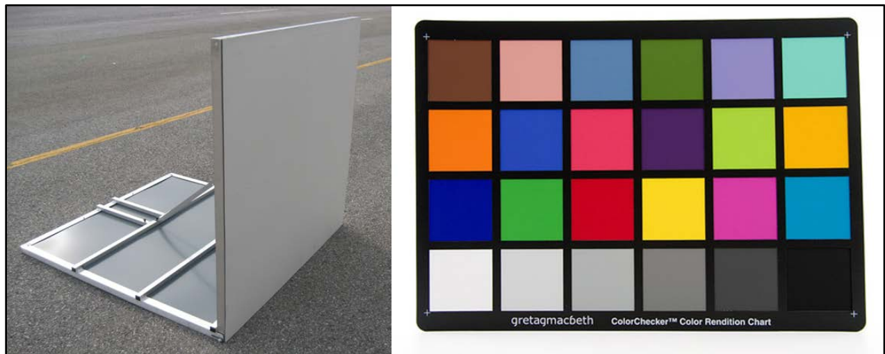
Figure 3. Images. Camera calibration equipment: diffuse white surface (left) and GretagMacbeth ColorChecker (right).
