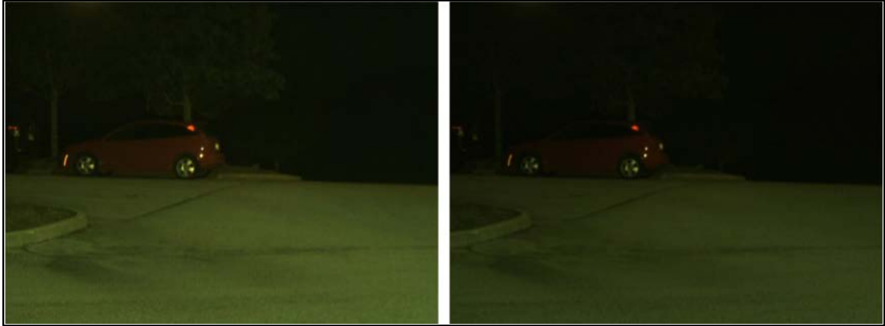
Figure 10. Photos. Scene with 55-ms exposure (left) and 33-ms exposure (right).
