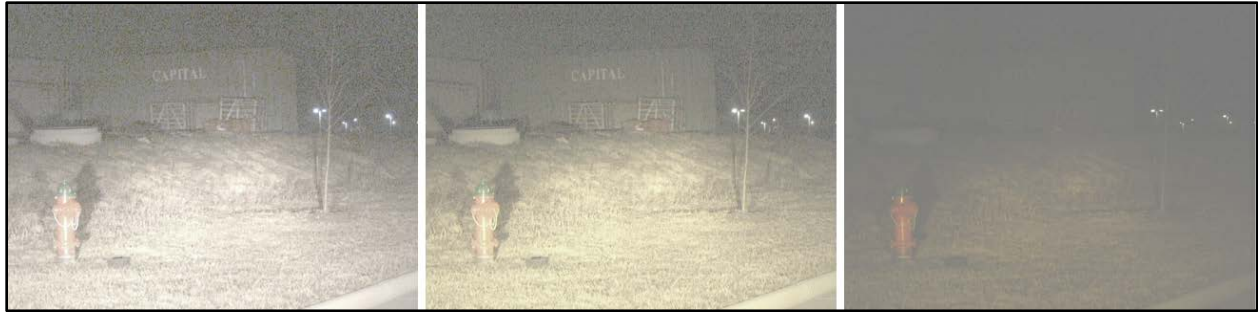
Figure 8. Photos. Examples of color camera system calibrated to 3500K LED lighting (left), 6000K LED lighting (center), and daylight (right).
