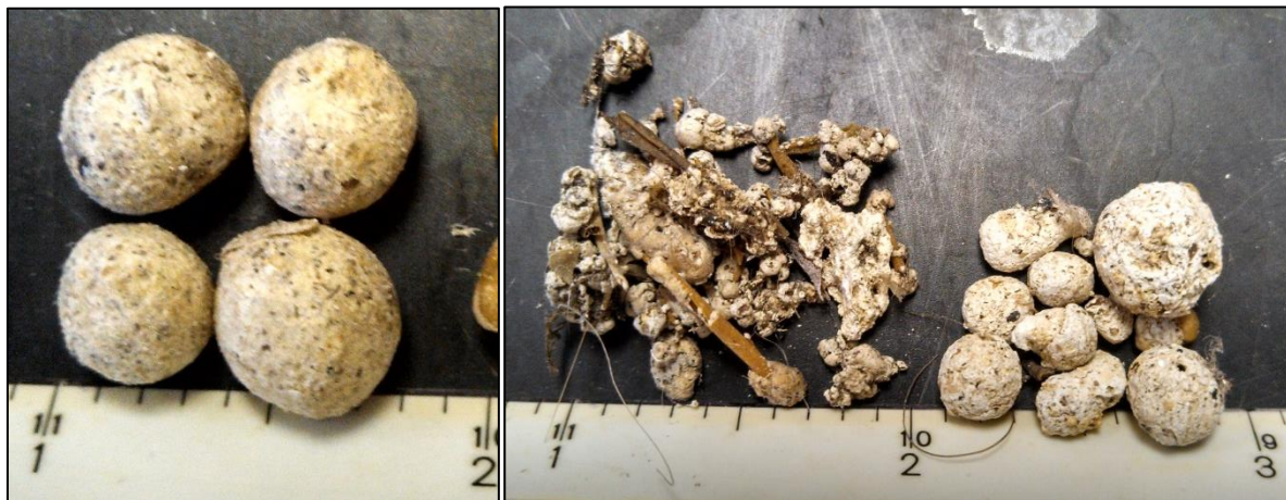
Figure 7 - Accumulated LCFAs after drying at 37°C from the FTA System APD (left), the FTG System GPD (middle), and the FTA System GPD (right) (ruler shown in inches)
