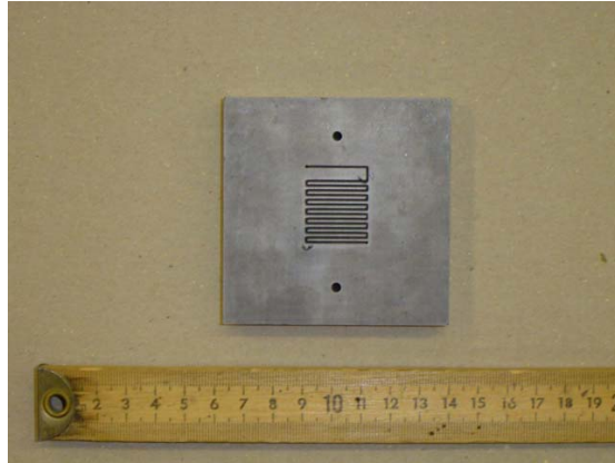
Figure 3.1 A flowfield with serpentine gas channels
