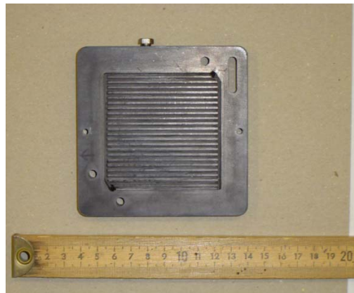
Figure 3.2 A flowfield with straight gas channels
