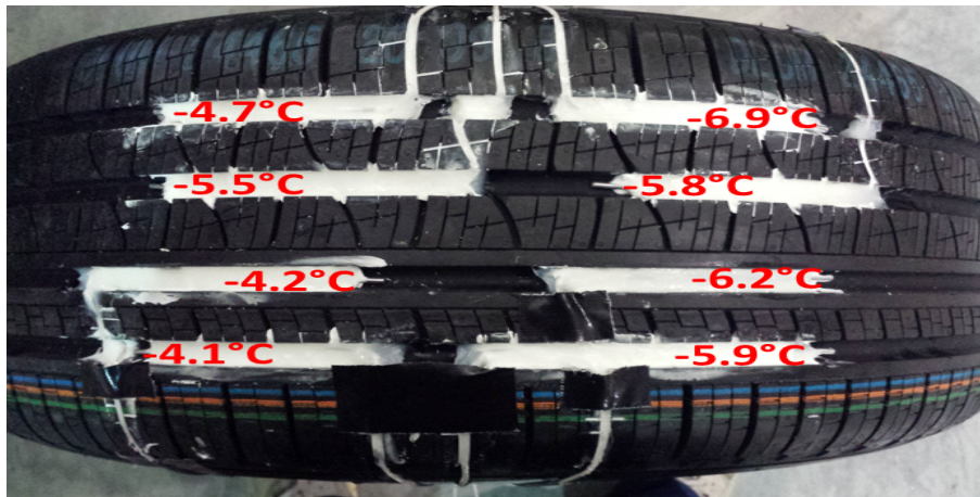
Figure 4.21: Temperature distribution measurements of contact patch for the P235/55R19 All-Season Pirelli Tire. The operating conditions were an ice surface temperature of -10^{\circ}\text{C} , inflation pressure of 35 psi, a normal load of 80% load index, +2^{\circ} camber angle, and an applied torque of 0 N-m at the wheel center.
