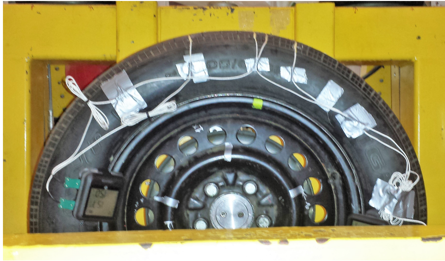
Figure B.4: Data loggers attached to the sidewall of the tire using 3M Heavy Duty Velcro.
