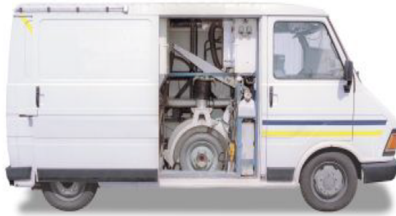
Figure 2.11: Laboratory vehicle that has been equipped with a measurement wheel. This wheel is located at the center of the vehicle. It operates independently of the other four wheels allowing for its dynamics to be investigated. Adapted from [8] under fair use; Fair use determination attached.
