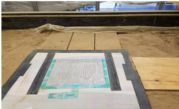
Figure 3.9: Final design for the test-setup to allow dynamic conditions to be tested on the TekScan Pressure Pad. System is composed of a wooden rigid platform covered with a plastic sheet on which the pressure pad and the protective film lays on.
