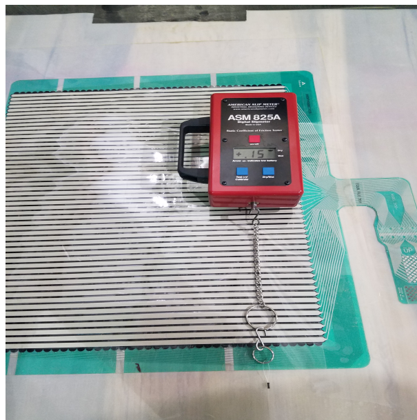
Figure 3.10: Static coefficient of friction of the pressure pad measuring system which mimics the smooth ice surface used for traction measurement.
