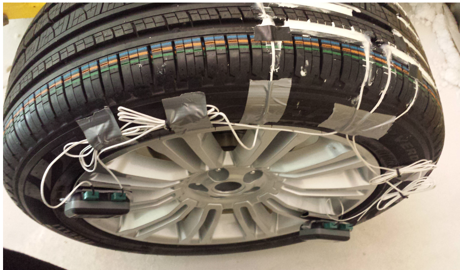
Figure B.5: Data loggers are attached at an equal distance from each other to prevent wheel imbalances.
