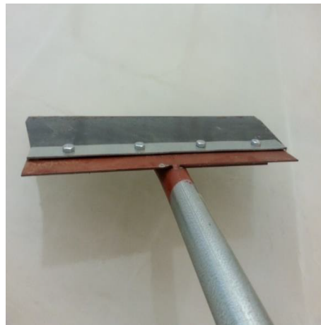
Figure 3.12: Metal scraper used to smooth the ice and create a consistent ice surface to be used for testing and allow repeatable conditions.
