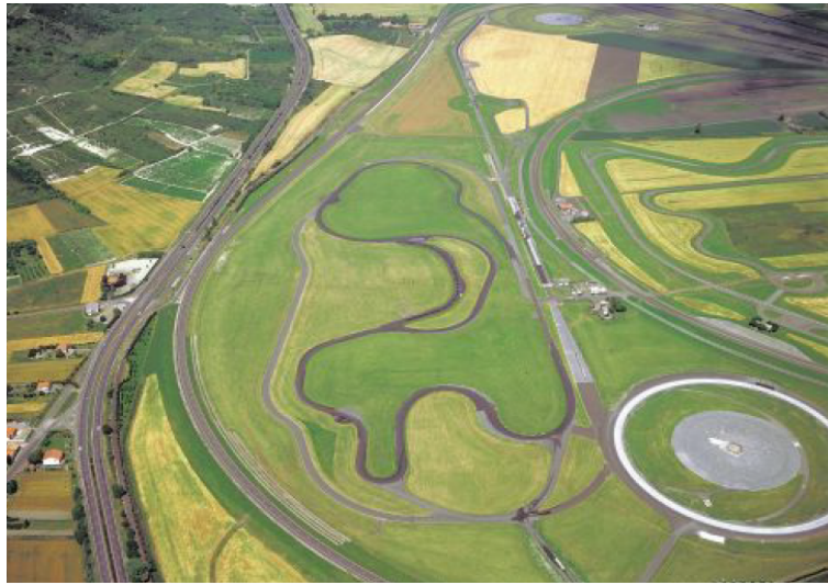
Figure 2.12: Combination circuit at the Ladoux test center, France. The track is referred to as the Duck (Canard) circuit because of its distinctive shape. This circuit alternates between wide bends, tight bends and straight stretches. Adapted from [9] under fair use; Fair use determination attached.
