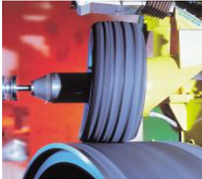
Figure 2.10: Road simulator in operation. The tire is running on the outside of the drum for this specific study. Adapted from [8] under fair use; Fair use determination attached.
