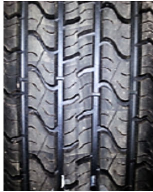
Figure 3.4: Tread pattern of P225/60R16 Standard Reference Test Tire ( SRTT )
