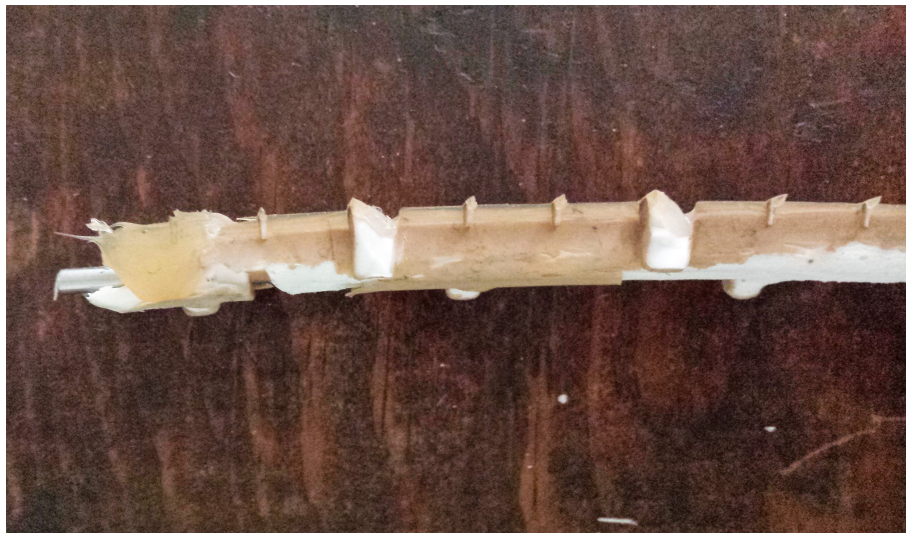
Figure B.7: After removing the thermocouples from the contact patch, the excess silicone can be peeled and scraped off.
