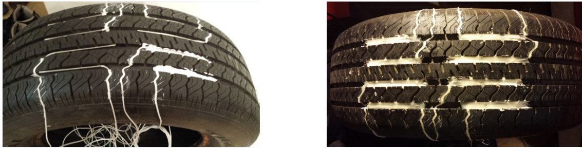
Figure 3.18: Instrumentation of the Standard Reference Test Tire ( SRTT )
