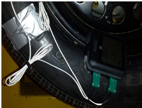
Figure 3.19: Wireless Data Logger used to transmit data from the measurement device to the communication point.
