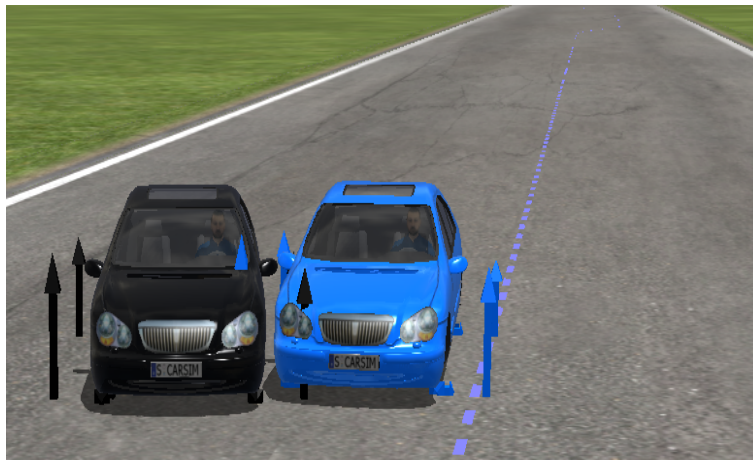
Figure 6.23: Comparison of the Modified Pacejka Tire Model (Blue) and Original Pacejka Tire Model (Black) at 120 km/h in CarSim.
