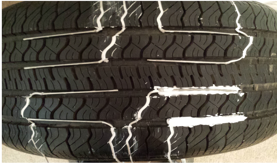
Figure B.2: After fitting the wires and thermocouples into the tire tread, apply silicone to the wires and thermocouples to adhere the measuring system to the tire.
