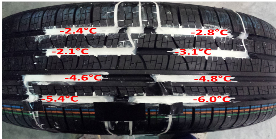
Figure 4.20: Temperature distribution measurements of contact patch for the P235/55R19 All-Season Pirelli Tire. The operating conditions were an ice surface temperature of -10^{\circ}\text{C} , inflation pressure of 35 psi, a normal load of 60% load index, +2^{\circ} camber angle, and an applied torque of 0 N-m at the wheel center.
