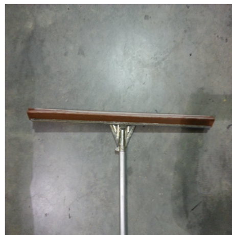
Figure 3.13: Rubber squeegee used as the final part of the ice preparation. This step removes all debris left behind from scraping.
