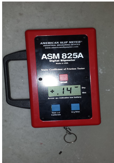
Figure 3.14: ASM 825A American Slip Meter used to measure the static coefficient of friction of dry and wet surfaces.
