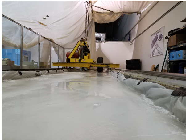
Figure 3.7: Terramechanics Rig at TMVS with water on top of solid ice.
