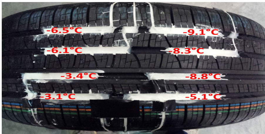
Figure 4.22: Temperature distribution measurements of contact patch for the P235/55R19 All-Season Pirelli Tire. The operating conditions were an ice surface temperature of -10^{\circ}\text{C} , inflation pressure of 35 psi, a normal load of 120% load index, and an applied torque of 0 N-m at the wheel center.
