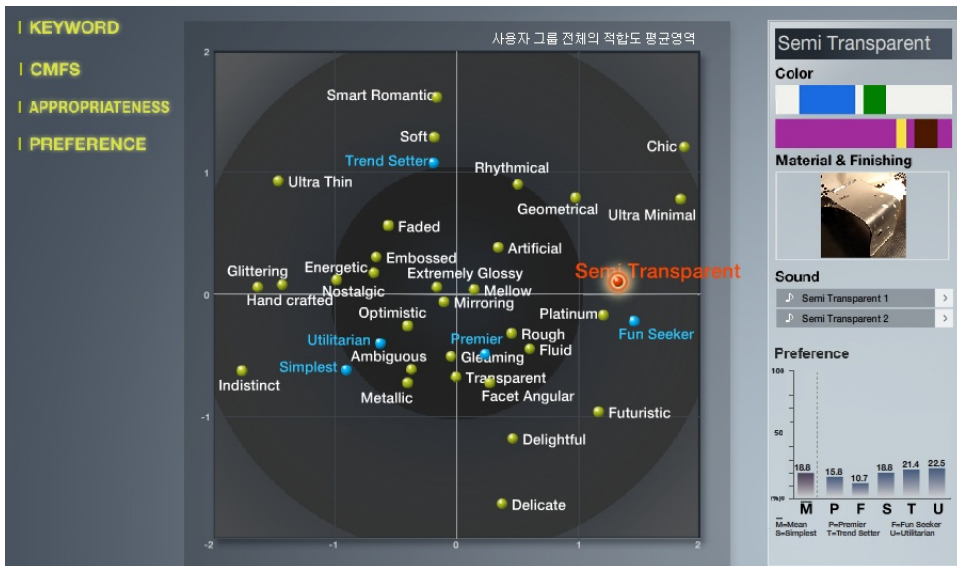
Figure 5: A screen shot of the emotional palette prototype system for mobile devices. Design elements mapped onto keywords and segmented user groups
