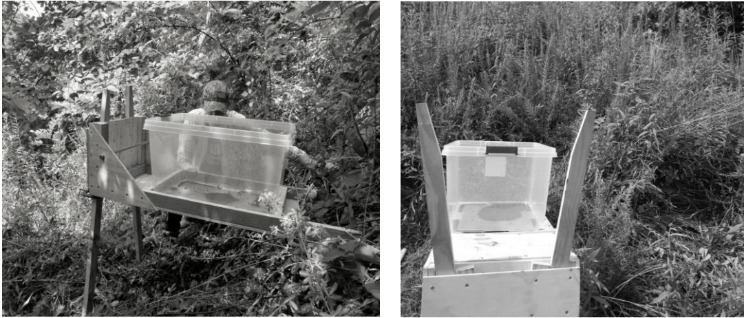
Figure 3.2 The left photo is of the reforested area and the right photo is of the grassed area. Both photos show the dye staining apparatus in place during a dye staining experiment.
