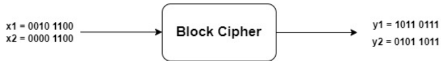
Figure 2.2: Diffusion property: switch 1 bit of x should not only change 1 bit of result y .
