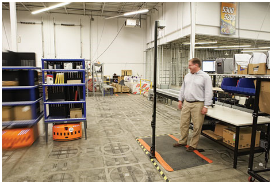
Figure 2-5. Kiva Systems® warehouse automation system.
