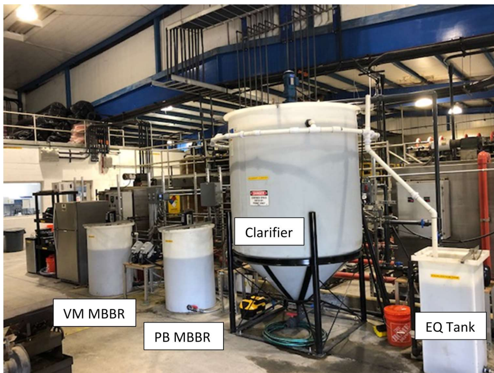
Figure 9. Pilot setup for PdNA MBBRs startup experiment.
