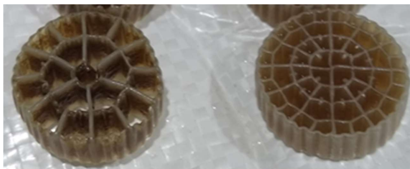
Figure 17. Pilot IFAS media (right) versus media from the first pilot MBBR (left).
