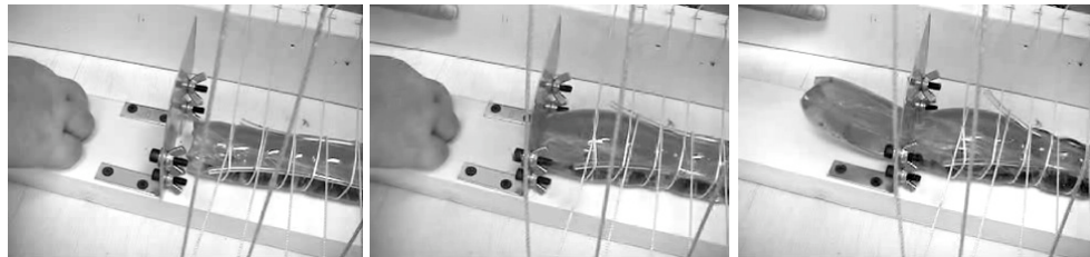
(b) Passing through a hole smaller than half the size of its nominal diameter
