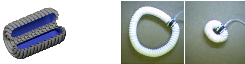
(a) WSL with pressurized expandable hoses (b) Expanded (c) Contracted
