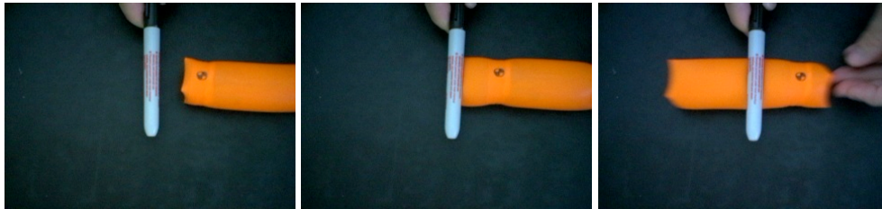
(a) Squeezing under a ‘collapsed ceiling’ using all surfaces for traction
