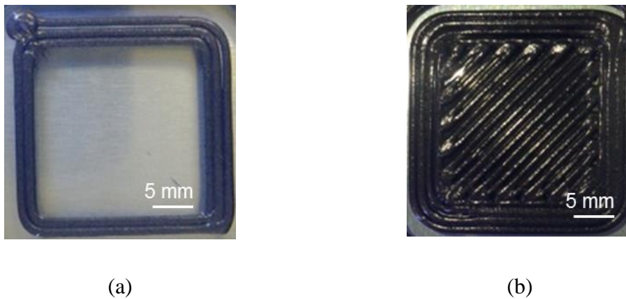
Fig. A-2. Example of printing structures: (a) incorrect input parameters with unacceptable print quality and (b) correct input parameters with acceptable print quality in material extrusion / retraction stages.
