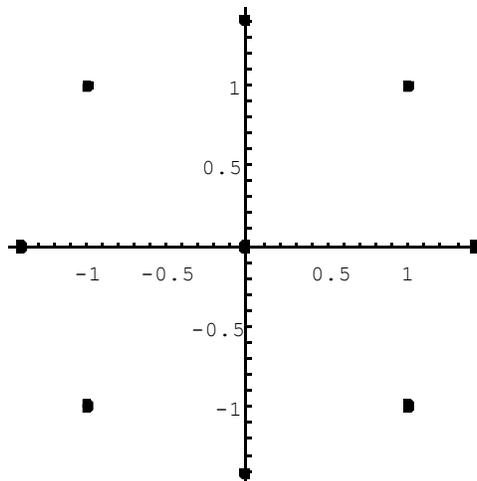
Figure 1.1 Two-Factor Central Composite Design with  $d = \sqrt{2}$  and  $n_c = 1$
