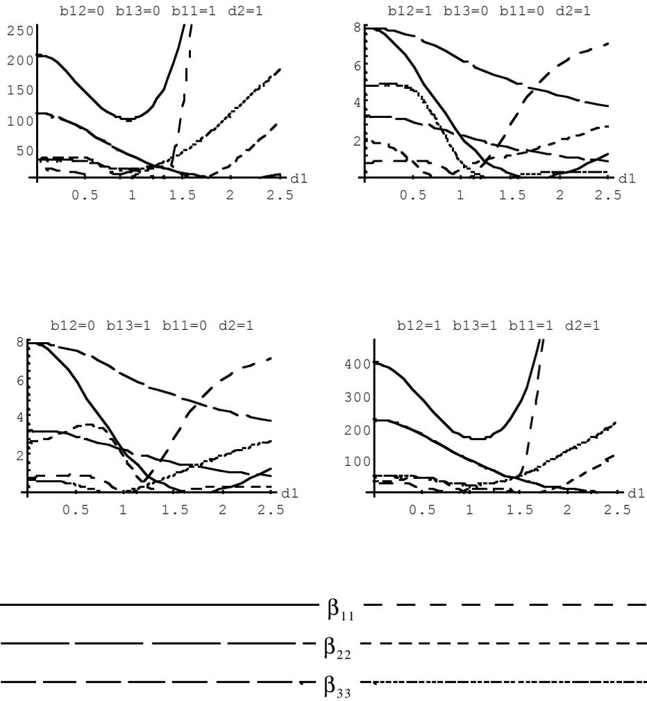
Figure 3.6 Squared Bias in Variance Estimate vs.  $d$  in a Three Factor CCD ( $d_2 = 1$ )
