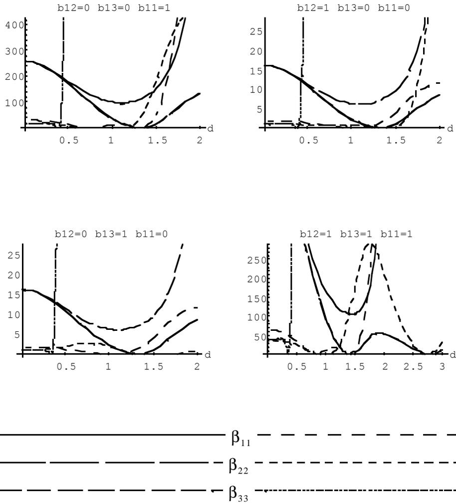
Figure 3.4 Squared Bias in Variance Estimate vs.  $d$  in a Three Factor CCD (Common  $d$ )
